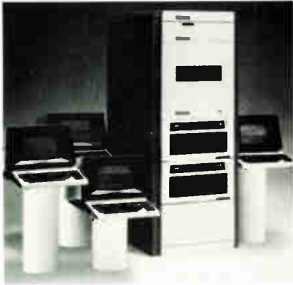
For programming. Executing the C language and UNIX operating system, BBN Computer's C/70 is a minicomputer billed as a software development system.
