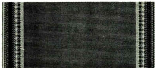
Each sensor element has 100:1 aspect ratio (25 \mu m center-to-center by 2.5 mm wide.)
