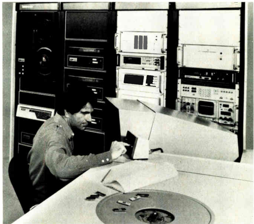
Versatile. Tektronix' new 3275 can be interfaced with any large computer. Its 2952 pattern processor will handle 16 clock phases for better data-stream pipelining.
