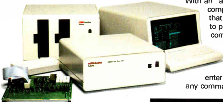
GenRad 2300 Microcomputer Development System with 2302 Slave Emulator for 8086 microprocessor. (Also available for GenRad 2301 network stations.)
