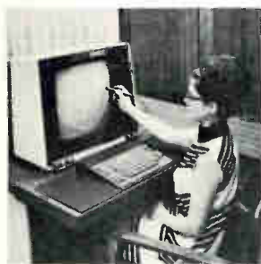
Graphic remote integrated display GRID 240 is for use in on-line computer interaction where output can be displayed in graphic form. Input to the system is by means of the light pen, alphanumeric keyboard or function keyboard which are provided as part of the system. System has its own processor with a 4K, 12-bit memory. Control Data Corp., 34th Ave. So., Minneapolis. [421]
