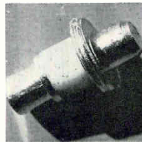
High-frequency, step recovery silicon diodes designed for X and Ku bands feature very low transition times. The GC-2500 series diodes offer all order multiplication from X2 through X20. Output power efficiencies range from 1/N to 2/N. Maximum snap time is 70 to 100 psec with maximum series resistance of 0.6 to 0.9 ohm. GHZ Devices Inc., Kennedy Dr., N. Chelmsford, Mass. [441]
