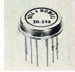
Hybrid IC FET input operational amplifier 20-248 is hermetically sealed at a cost comparable to plastic cased units. It is packaged in a TO-8 case and is operable over the full military temperature range. Maximum input bias current is 5 pa. Unit is available for immediate delivery and price is $30. Bell & Howell, Control Products Div., 706 Bostwick Ave., Bridgeport, Conn. [439]
