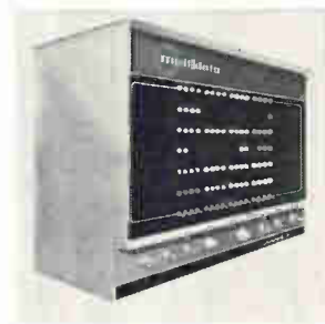
System-oriented computer model A includes 4,096 16-bit words of core memory, 32,768 words of disk memory, a memory access controller, a central processor, an input/output bus, and a teletypewriter with paper tape reader and punch. The 32,768-word disk is field expandable to 65,536 or 131,072 words. Price is $14,995. Multidata, 15142 Goldenwest Circle, Westminster, Calif. [426]
