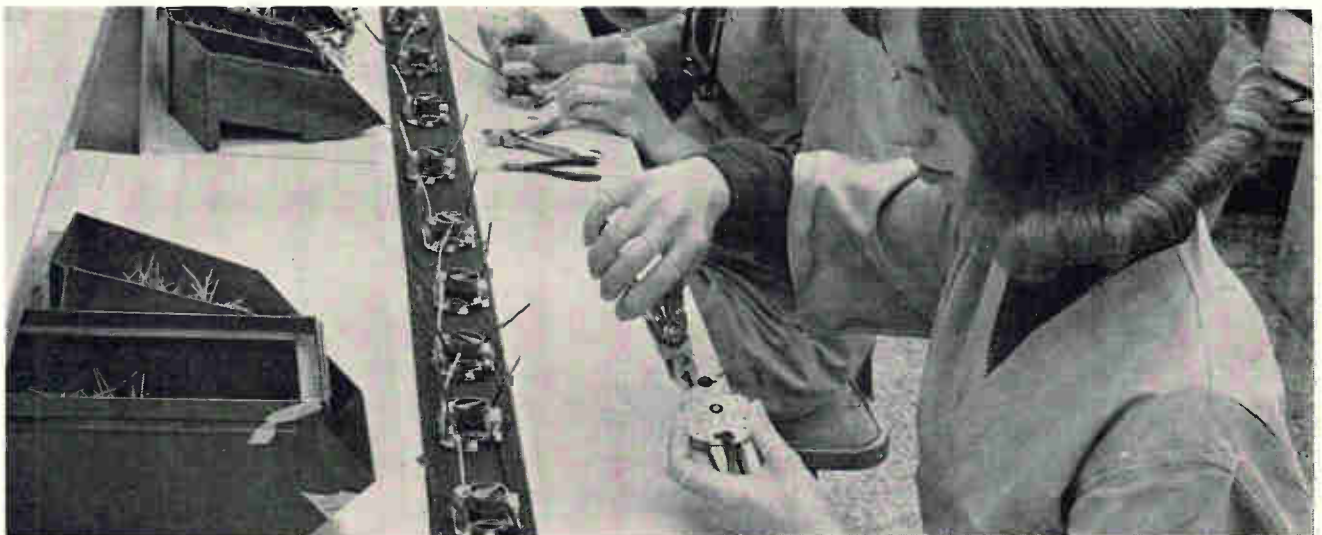
On the line. Employees at Motorola work on motor-speed controls for power tools. Subassemblies of this type can be easily installed by customers in a variety of industrial and consumer goods.
