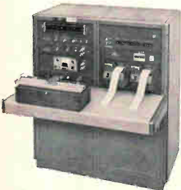
An automatic capacitor-test system produced by General Radio.
