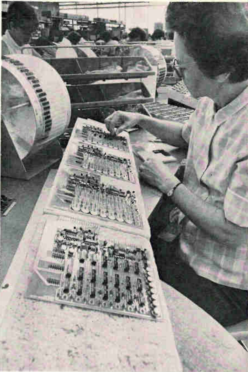
Homemade. Production worker inserts proprietary Hewlett-Packard IC's into circuit board which will be installed in a new electronic counter.
