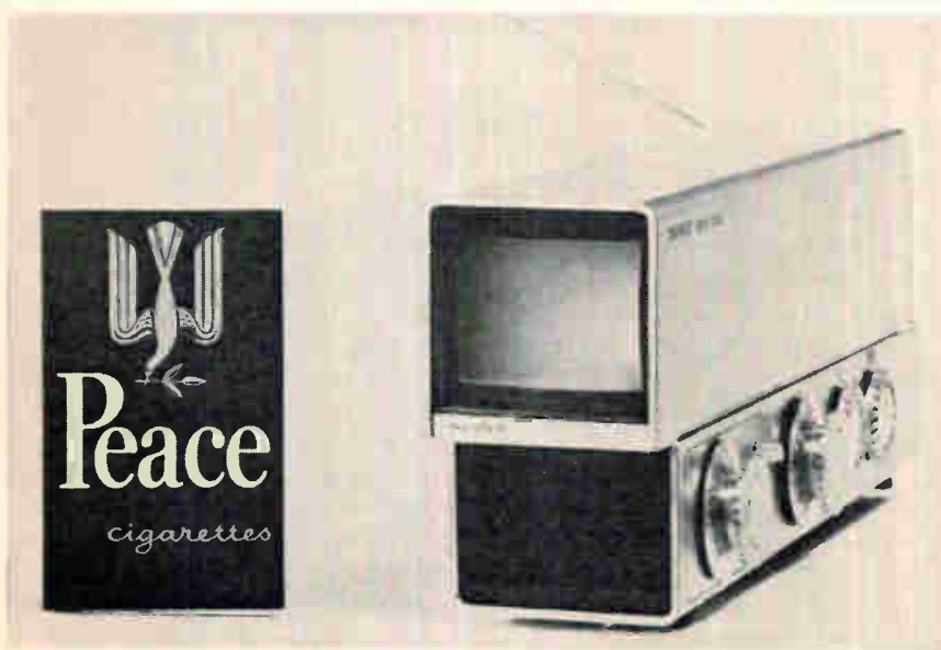
Eye opener. Sony's first tv set with integrated circuits has 1-inch picture tube.
