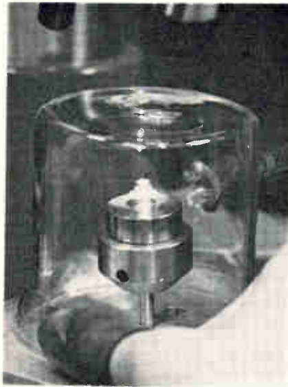
Light welder. A stainless steel jig aligns components for a miniature klystron as a laser beam bonds the parts. The glass bell jar holds argon, which prevents oxidation of the components during the welding operation.
