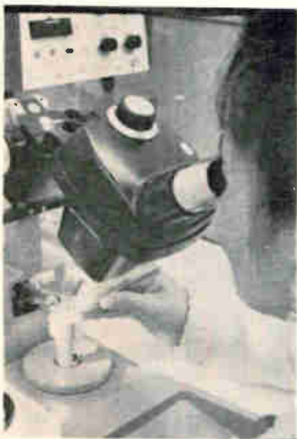
Eagle eye. Worker bonds flatpack assembly in Hewlett-Packard's integrated-circuit facility.
