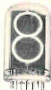
■ JUMBO SIDE VIEWING Character Size . . . 2.0" Viewing Distance . . . 100' for large audience displays to 100' preferred type for lower cost and minimal width
