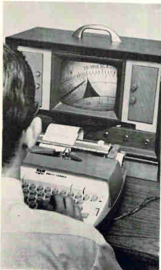
Audio-visual teaching machine developed by Dorsett Industries costs $450 and permits student to respond in three ways: by typing answers on the keyboard of an electric typewriter (left), speaking into microphone (top), or printing in block letters on pad of paper on electric grid (right).
