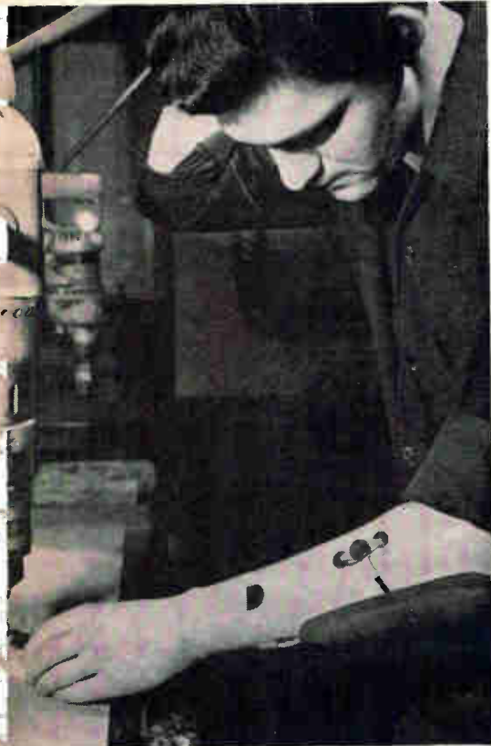
Steady. Electromyographic-controlled artificial hand manufactured in Austria has selective amplifier circuits that protect users from spurious finger movements.
