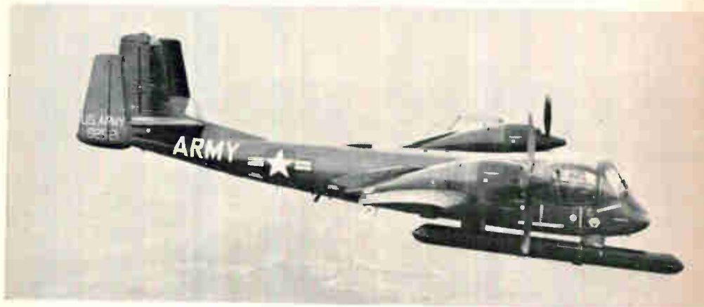
Success story. Army's Mohawk surveillance aircraft can data-link infrared and side-looking radar pictures of targets back to base almost immediately.
