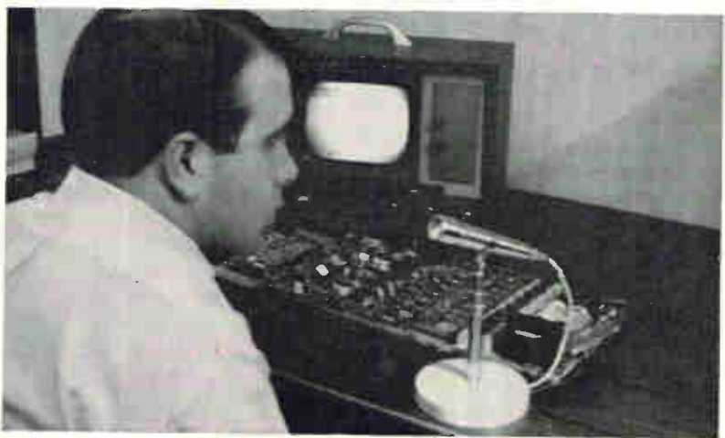
Audio-visual teaching machine developed by Dorsett Industries costs $450 and permits student to respond in three ways: by typing answers on the keyboard of an electric typewriter (left), speaking into microphone (top), or printing in block letters on pad of paper on electric grid (right).
