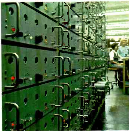
In one of numerous tests, all Model 5245L crystal oscillator assemblies are operated and observed for two weeks to determine aging rates.
