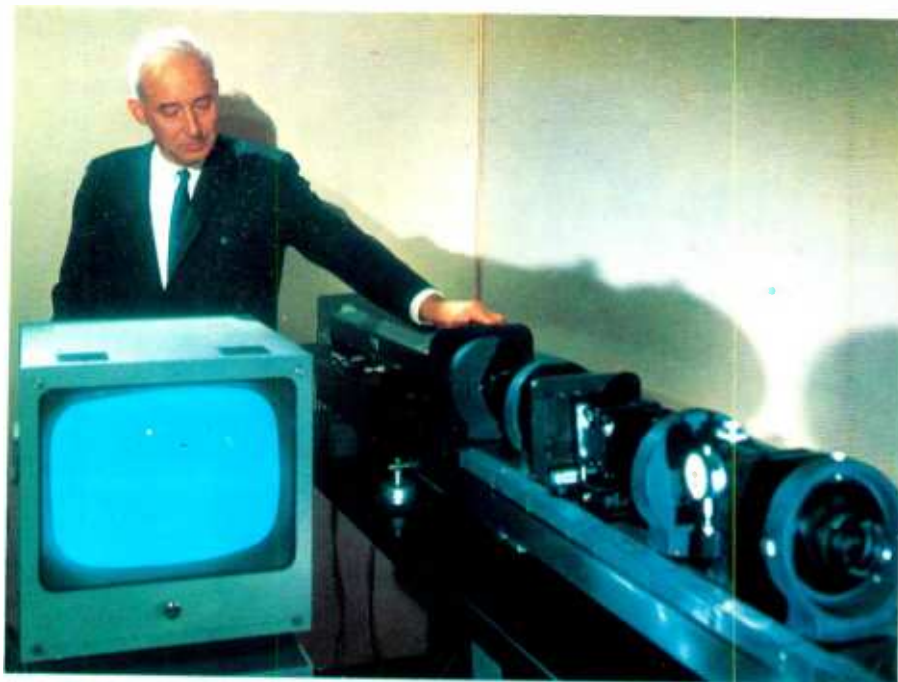
Dr. Milton B. Dobrin, United Geophysical Corporation, Pasadena, demonstrates optical filtering technique used to enhance seismic data.
