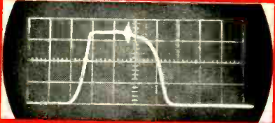
B. Crystal filter response, 3 dB bandwidth is 2.8 kHz wide at 10.7 MHz center frequency.
