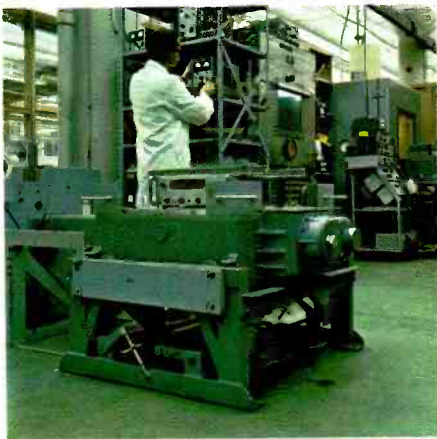
Here's a small part of hp's extensive in-house test facility where instruments are tested under extreme shock, vibration, temperature, humidity and electromagnetic conditions.
