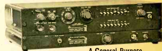
A General-Purpose 100-MHz Pulse Generator for Under $1000
