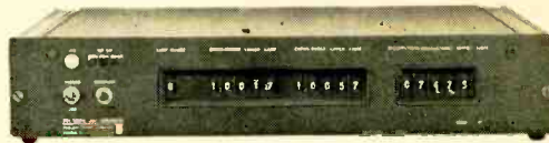
New Automatic Go, No-Go Capacitor Testing
