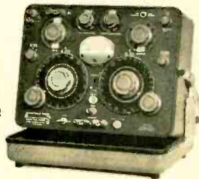
1-pF to 1-F Electrolytic Capacitance Bridge
