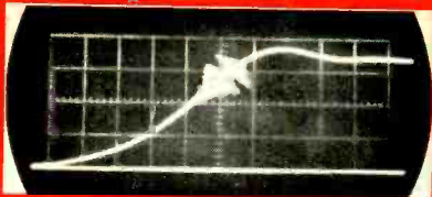
C. Same crystal filter as in (B) above, with 1/10 the sweep width (100 Hz/Div.).
