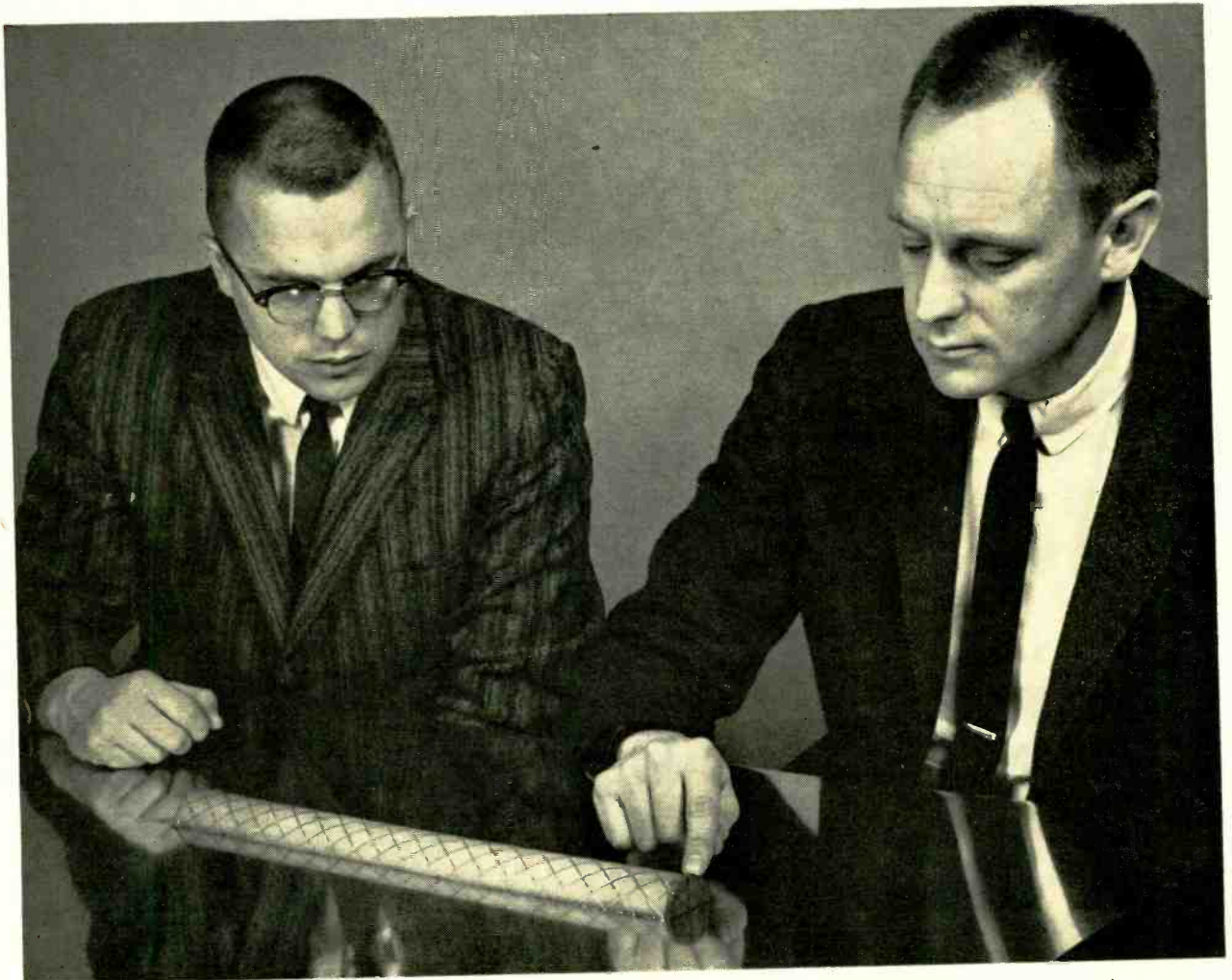
Linearly polarized contrawound helix's electrical and physical symmetry permit design of half-diameter antenna on ground plane. Carl W. Gerst, left, and Robert A. Worden look at a printed circuit octafilar version with a 9-to-1 bandwidth. Portions of eight windings are printed on each side of the dielectric cylinder.
