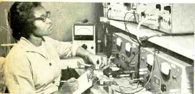
100% testing for 450 Mc/s gain and noise figure
