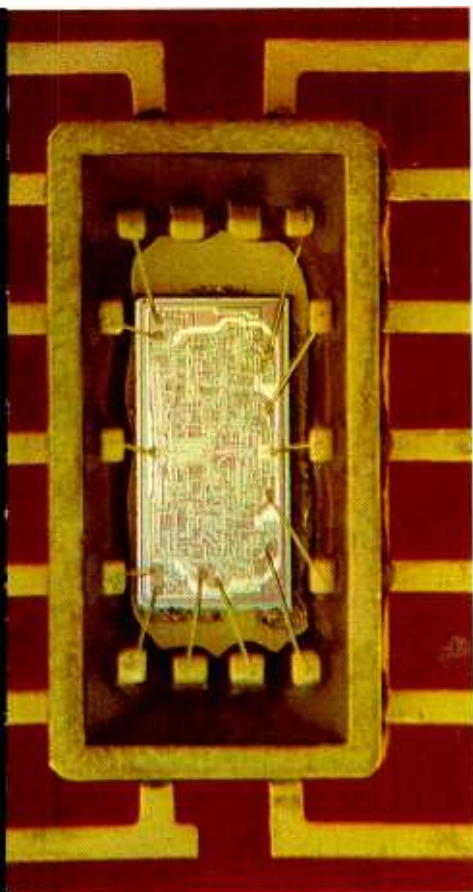
Sixteen bits of memory are packed into a chip by Texas Instruments.
