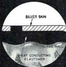
Enlarged section of Elastaclamp's inner cartridge.
