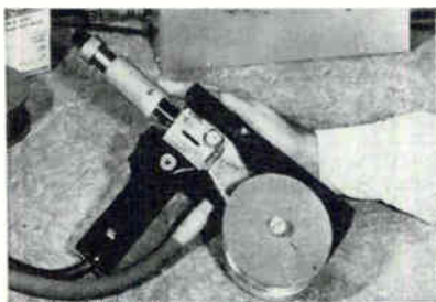
Filler wire is on spool, feed motor is in handle
