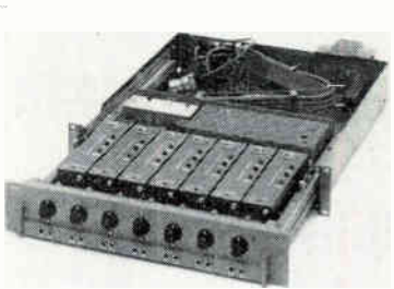
Direct-record amplifier rack. Front panel contains attenuator, input and output jacks
