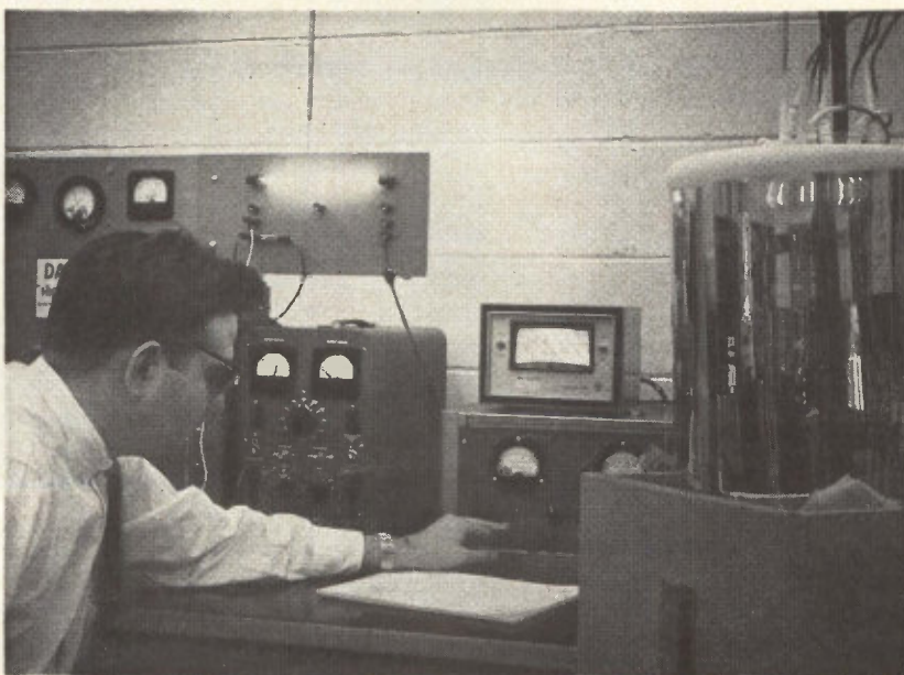
FIRING LASER flash tube with superconducting inductive power supply. Cryogenic energy storage dewar is at right, in right center is a gaussmeter atop the thermal switch control instrument; the power supply and associated circuitry is at left
