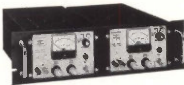
Two Trygon HR20-1.5's, rack-mounted side by side.
