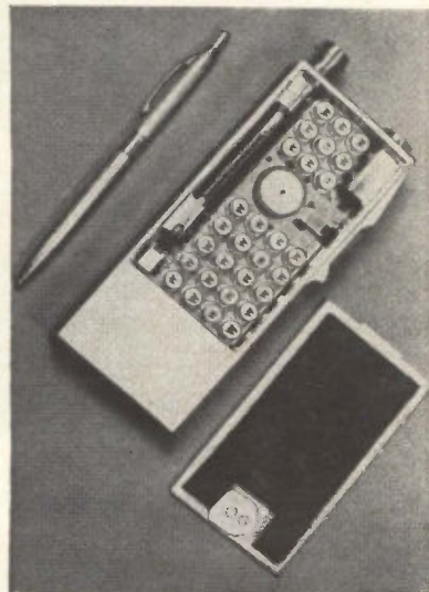
RESEARCH MODEL of a 120-Mc, a-m transmitter-receiver was built by Motorola for Air Force to demonstrate use of integrated circuits in vhf equipment. With case closed, it looks like regular transistor radio
