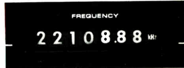
Frequency resolution to nearest 10 Hz in phase-locked tuning mode is displayed on flat-plane, high-brightness readouts. Alternative continuous tuning mode presents frequency resolved to nearest 100 kHz.
