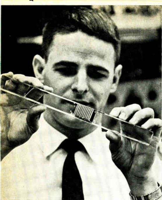
See-through. Anthony van den Heuvel, a scientist at IIT Research Institute, examines an acoustic delay line in which piezoelectric thin film taps are deposited on a glass substrate.
