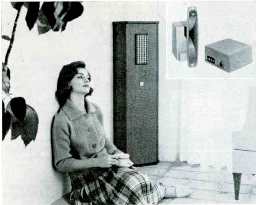
Speaker unit houses Ionovac, mid-range speakers and woofer. System includes (inset) power supply, modulator mounted at rear of acoustic horn
