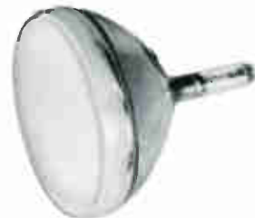
SYLVANIA-3BMP1—a 3"-diameter tube with flat, clear faceplate. It offers electrostatic focus and deflection, features post-deflection acceleration. Available with a wide choice of screen phosphors.
