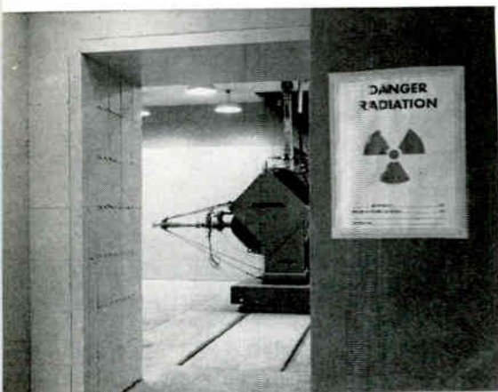
Output equipment, on floor below generator. Targets bombarded are placed in front of horizontal tube at left
