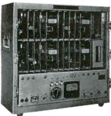
Terminal bay contains channel equipment and power supply panel.
