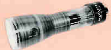
SYLVANIA-3BMP1—a 3"-diameter tube with flat, clear faceplate. It offers electrostatic focus and deflection, features post-deflection acceleration. Available with a wide choice of screen phosphors.
