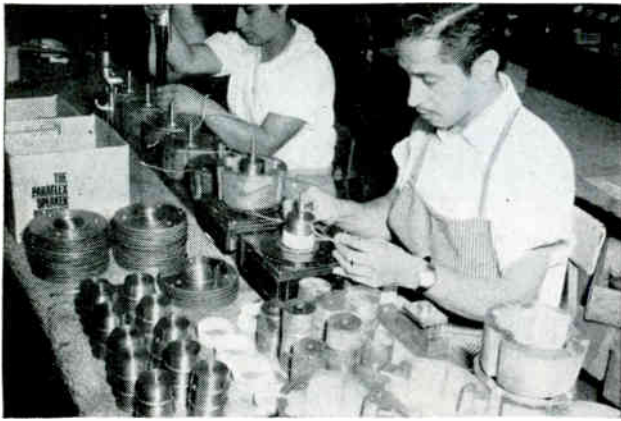
Magnetizing coils are placed around large magnets before magnet assembly is put together
