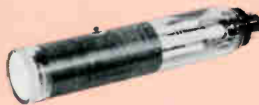
SYLVANIA SC-3016—featuring high deflection sensitivity, compact length of only 6", flat circular 1 1/8" face, electrostatic focus and deflection. Available with several different screen phosphors.
