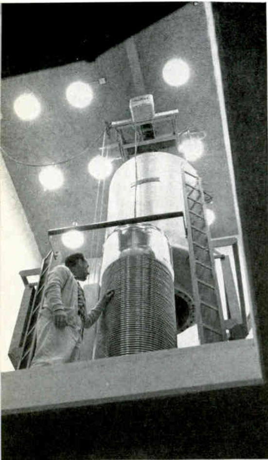
Van de Graaff generator (vacuum tank removed) installed at new radiation physics lab
