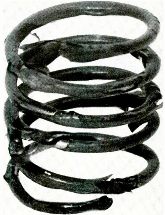
This "Glyptal"-insulated wire was exposed to ordinary chlorinated solvent for the same length of time as the one on the left. The solvent dissolved the resin binder and softened the olkyd finish.
