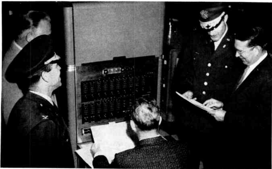
IBM tape RAMAC data-processing system, installed at Anniston Ordnance Depot, Anniston, Alabama, has total disk-memory capacity of 24 million characters. U. S. Army Ordnance Corps uses machine to handle its average of 5,500 daily supply transactions
