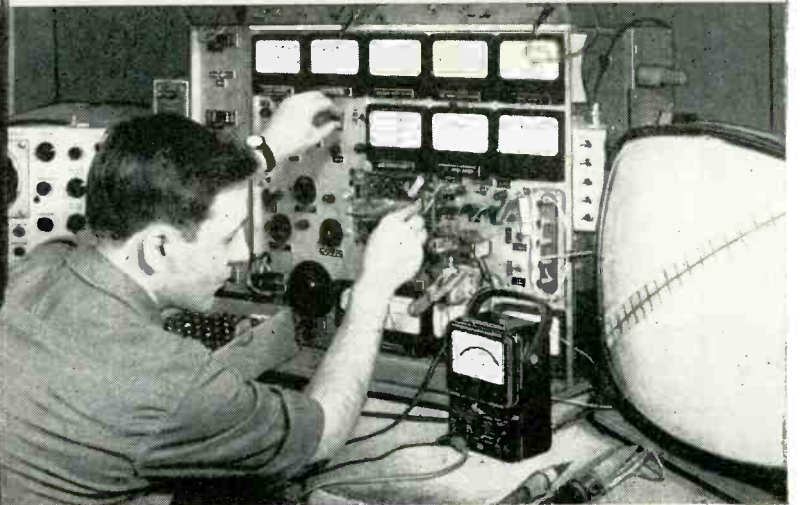
Photo courtesy of Admiral Corp. Engineer shown is using the Model 270 in evaluating operating characteristics of developmental type deflection tube.
