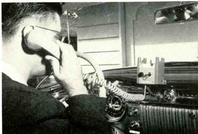
Mobile communications systems like this one by Lenkurt allow callers in vehicles to hold private conversations at will
