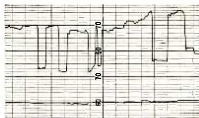
FIG. 7—Input (top) and output (bottom) levels of burst portion of color signal
