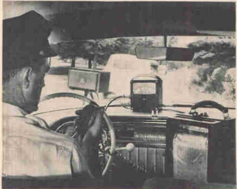
Complete transmitter and receiver assembly. Lighthouse oscillator tube is mounted horizontally at top-right
