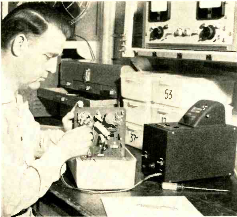
Detection unit is checked out with clock calibrator shown at right
