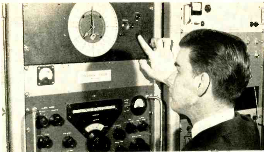
Regenerative frequency divider assembly shown in operation driving the precision clock above it. Device has proven highly reliable over long period
