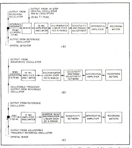
FIG. 5—Metering circuit employing crystal mixer (A) with sealed-tunable reference resonator (B) and optimum metering arrangement for sensitive scale measurements (C)
