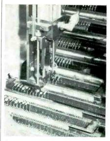
Top view of insertion head, showing notched blades that push component down through magazine
