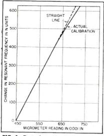
FIG. 6—Typical calibration curve of sealed-tunable cavity resonator
