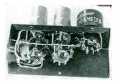
Underchassis view of the simple frequency meter
