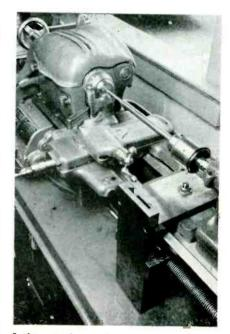
Lathe attachment for cutting nonlinearpitch screws, shown in place at right of carriage on lathe. Vertically-moving cam plate inside attachment drives tool holder carriage at nonlinear rate
