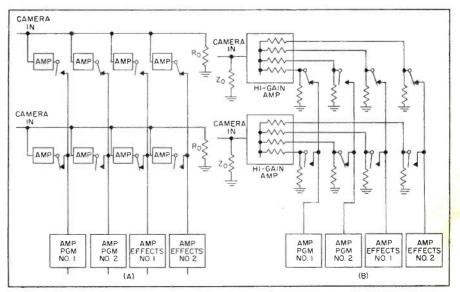
FIG. 2—Electron-tube method (A) provides —50-db isolation at 3.58 mc. High-gain amplifier drives resistance splitting pads (B) to provide 36 db of transient crosstalk isolation
