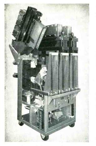
**ROLLED AND MOLDED ARC CHUTE SHELLS,** made by C-D-F for the I-T-E Circuit Breaker Company for 7.5 and 15 KV air magnetic circuit breaker, are good examples of paper-base Dilecto doing a hard job. Each completely closed insulating shell (NEMA grade X) has flame-retardant construction, negligible water absorption, and high dielectric strength at all points to withstand impulse test requirements.
