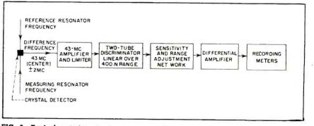
FIG. 3-Typical metering circuit arrangement for microwave refractometer
