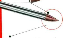
KEYSTONE NTC Thermistor in nose of stainless steel probe decreases in electrical resistance as temperature rises, permitting greater circuit current flow, thus actuating external tempera-ture gauge. Circuit consists of regulated voltage supply with thermistor and gauge connected in series.
