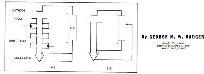
FIG. 1—Normal klystron connection to beam power supply (A) and connection for collector depression (B) to decrease power input to klystron
