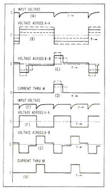
FIG. 2—Waveforms appearing at various points of Fig. 1
