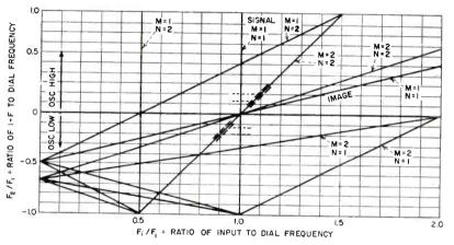
In the case of a receiver with a wide i-f bandwidth or one with a sweeping local oscillator, each line becomes a band whose boundaries are obtained by drawing two lines parallel to and equidistant from the original line. The displacement in the vertical direction from the original line is
