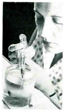
Applying air pressure with hypodermic syringe while relay is submerged in alcohol, to check for leaks. Flexible silver "needle" of hypo is soldered to relay evacuation opening
