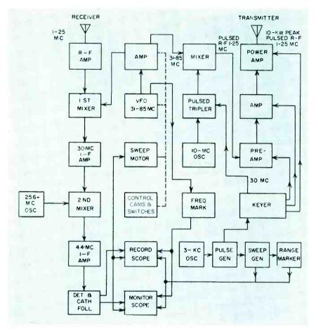
FIG. 6—Ionospheric recorder uses common vio to track receiver with transmitter
