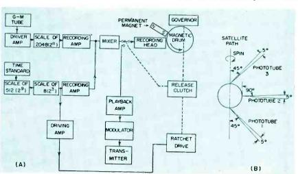
FIG. 4—Equipments to be carried in the earth satellite include recording cosmic-ray counter (A) and system for determining cloud cover of earth (B)
