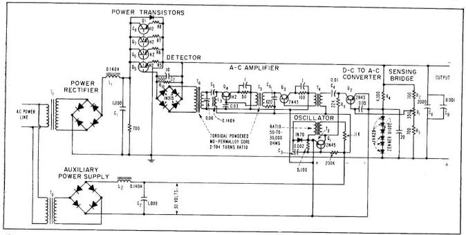
FIG. 2—Power supply uses transistors and diodes to provide 100-mv regulation at 70 volts
