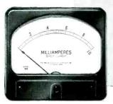
Molded-phenolic sealed cases for semi-flush or surface mounting. Has new miniature-type movement and extra long scale. DC scale length 334". AC scale length 33/16". Permits choice of two mounting stud locations for maximum versatility. Illumination technique permits easy bulb change from front panel. Also available without illumination feature.
