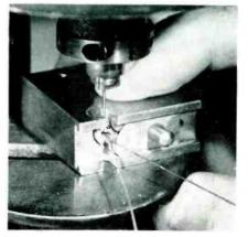
Fixture holds header on watch-tapping machine for threading tiny silver bushing
