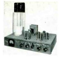
First Model Nuclear Reactor A working replica of the famous Aquarium Reactor with a genuine analog computer which automatically solves the pile kinetic equations. Neutron flux is read directly on the microammeter. 21/2 decade range. Blue light in tank represents Cerenkov radiation. Control rod regulates reaction, safety rod "icrams" it when it reaches too high a level. Reactor syllabut, experiment manual included. 110 volt, A.C. operated. Introductory price, \$295.
