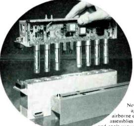
New "packaging" for airborne electronic assemblies insulates and cools vacuum tubes.
