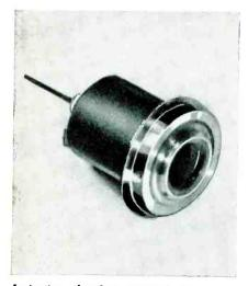
Ionization chamber mounted on rocket skin to measure solar radiation
