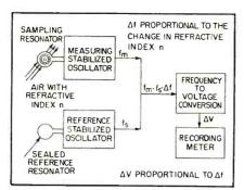
FIG. 1—Basic arrangement of airborne microwave refractometer
