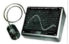
The VERNISTAT Adjustable Function Generator—a variation of the VERNISTAT a.c. potentiometer permits quick and easy alteration of any nonlinear function. The adjusting mechanism provides a graphic display of the function which may be mathematical or empirical, including those with multiple slope reversals.
