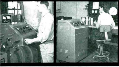
FOR VACUUM SYSTEMS or pressure systems the Type M-1 Mass Spectrometer leak detector will locate leaks as small as  $5 \times 10^{-10}$  standard cubic centimeters of air per second. Shown above (left) checking an evacuated refrigeration cooling unit, the detector detects leaks so small that in 1000 years only 1 cubic inch of air would pass through the opening.
