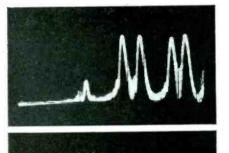
Scope pattern taken from Hoffman CV-157 showing two dualtone teletype channels on upper sideband, carrier partially suppressed. Each sideband can carry 32 teletype channels at one time.
