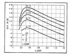
FIG. 2-Gain characteristics of the curved reflector
