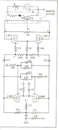
FIG. 1—Pulse repetition rates from 0 to 5 kc are shown on the meter
