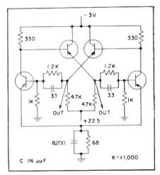
FIG. 5-Nonsaturating emitter-followercoupled flip-flop uses emitter biasing
