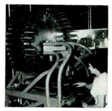
All types of components having identical lead hole spacings can be inserted one after another on a wiring board merely by positioning a pantograph stylus in one hole after another on a template and pulling a trigger each time. Magazineholding drum indexes one position after each insertion
