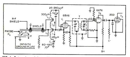
FIG. 4—Dot-sensing unit is sensitive to spot capacitance C, of dot printed on document; C, has value of 1  $\mu\mu f$  and is function of document thickness d and dielectric constant
