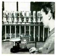
Weighing microwave antenna before filling with foam plastic
