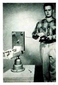
Ball-bearing fixture permits anchored ends of wires to turn independently of each other while wires are being twisted together
