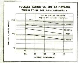
OPERATES FOR 1 YEAR AT 125 C Molded PVZ capacitors are designed for a minimum of one year's life at rated voltage and 125 C operation. Curves shown above are typical of performance.
