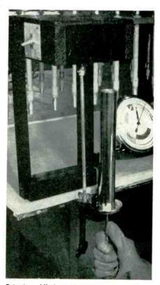
Bringing filled applicator up to motordriven mixer. Sawtooth-shaped paddle on mixer can be seen at left of base of applicator. Mixing time is about 1 minute
