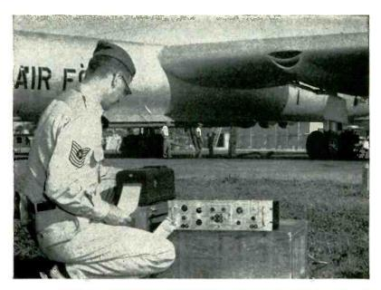
**Checks bomber refueling.** Brush instruments are rugged and durable, maintain accuracy in field use. Here they record surge pressures in gas tanks of a Strategic Air Command B-36 during refueling. For top performance, bomber must be refueled in a hurry, yet flow rate of 600 gallons per minute posed a pressure problem. Brush Recording Systems provided necessary facts.
