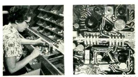
**PACKAGED** circuits are inserted in plated circuit boards at Motorola. Finished chassis, right, shows how
