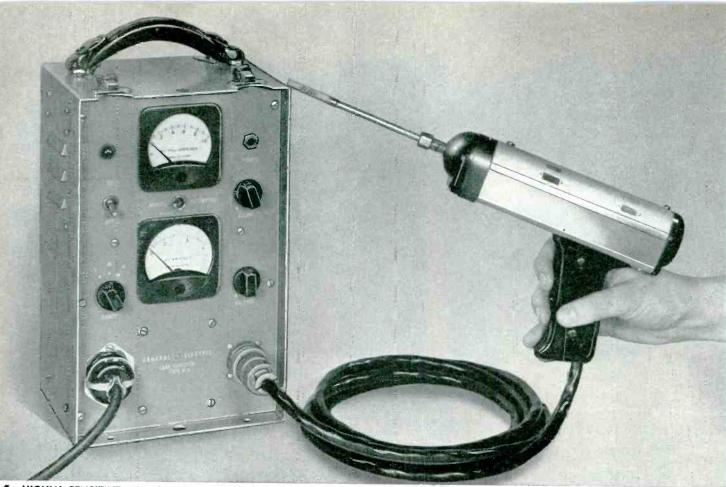
**HIGHLY SENSITIVE**, the G-E Halogen leak detector, Type H-1 will find a leak of 1/100 ounce of "Freon"\* a year. Use it to check for leaks in pressure systems such as refrigeration equipment as well as in closed systems into which a tracer gas and pressure can be placed such as tanks, tubing, fuel
