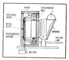
FIG. 4—Electronic printing device using photoemissive cathode
