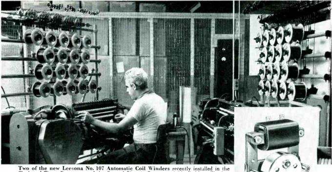
Two of the new Leesona No. 107 Automatic Coil Winders recently installed in the Clock and Timer Department of the General Electric Company, Ashland, Mass. The last word in automatic coil wincer design, No. 107's wind paper-insulated coils in stick form. Automatic operation eliminates human error, reduces wire breakage to a minimum, cuts production time and costs. Inset shows a Type H3 Synchronous Motor, one of many Telechron timing units with coil: precision-wound on Leesona No. 107 machines.
