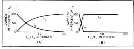
FIG. 2—Curves show improvement in characteristics of typical collectors (A) compared to special collectors (B) of the segmented type
