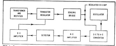
FIG. 1—Power supply regulating system in block form. The d-c amplifier between detector and regulating element is required only when oscillator frequency is above 30 kc.
