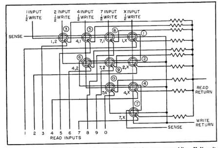
FIG. 3—Digit memory plane uses 10 RCA XF-1778 ferrite core assemblies. Half write pulse is 85 ma, read pulse is 1,000 ma and sense pulse is 80 v
