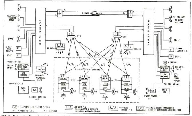
FIG. 3—Railroad radio and multiplex communications system uses microwaves for broadband radio and f-m tranceivers for ctc
