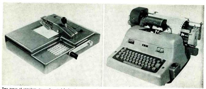
Two types of encoders; typewriter at right imprints code simultaneously with printing of digit
