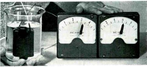
These silver-chloride/magnesium type batteries deliver up POWER to 42 watt hours per pound and 3 watt hours per cubic inch, with nearly level power output over total operating life.
