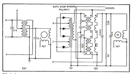
FIG. 2—Diagram shows method of connecting servo amplifier to transformer (A) and to saturable reactor (B) shown in Fig. 1
