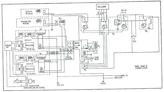
FIG. 8-Sampling panel circuits transfer a-c power from normal to standby equipment
