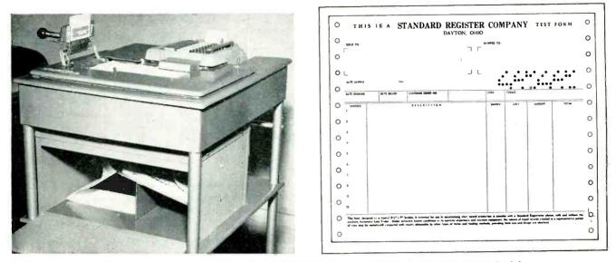
Coding register for standard perforated-edge business forms (left) imprints dot code on upper right of form (right)
