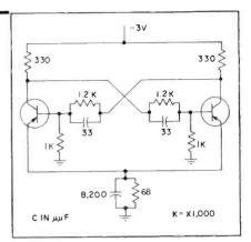
FIG. 4—Nonsaturating resistance-coupled flip-flop has d-c feedback
