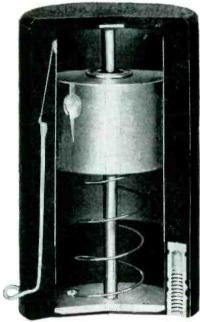
The RAM accelerometer is a uniquelydesigned, extremely low-friction type. Hermetic sealing with Rezolin compounds of BAKELITE Epoxy Resin provides a constant self-damping factor over a wide altitude temperature range. In cross section above, vertical white lines marking cylinder walls are formed by thousands of fine wire windings firmly embedded in epoxy.
