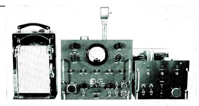
Recording meter, refractometer (external cavity above) and airborne power supply make up the measuring equipment
