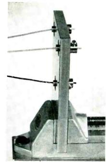
Details of fixture. Set screws hold wires in ball-bearing collars
