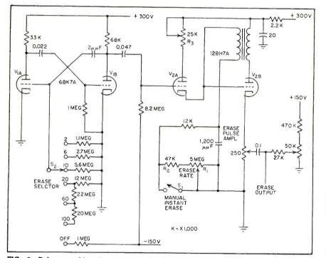
FIG. 2—Pulse repetition frequency of blocking oscillator controls latron persistence
