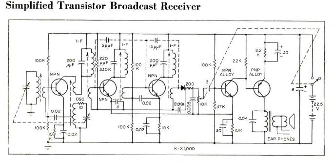
Similar to the Sony TR-55 receiver described on p 174 of the Dec. 1955 issue, the TR-57 shows evidences of simplification, having fewer parts, although it uses a 22.5-volt battery. Sensitivity is improved, being about 1 microvolt per meter. Selectivity is said to be 15 db and maximum undistorted output 20 milliwatts. The npn audio amplifier is a special alloy type
