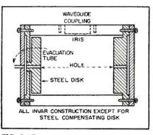
FIG. 2—Temperature-compensated, pressure-isolated resonator
