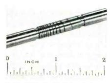
Sample screw cut with lathe attachment. Screw pitch is determined by cam
