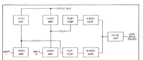
FIG. 6-Beam-switching method still in developmental stage
