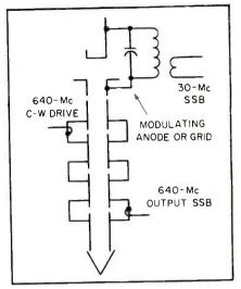
FIG. 5-Klystron connected as a highlevel mixer for high efficiency ssb power at ultrahigh frequency
