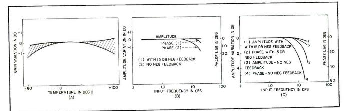
FIG. 3—Curves show spread of gain-temperature characteristic over twelve tests (A), response characteristic of 0.75-watt system (B) and 7.5-watt system (C) with and without negative feedback
