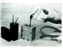
Stycast 2741 retains flexibility at -70 F and is, therefore, recommended for encapsulating, potting and sealing applications requiring low temperature use. It can also be used at +300 F without harmful effects. Shrinkage during cure is negligible; adhesion to most materials is excellent. Stycast 2741 is guite effective in adhesive applications where some flexibility is advantageous. Circle P5 inside back cover.
