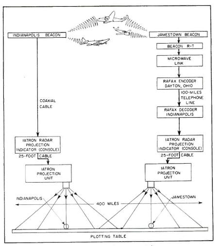
FIG. 3-CAA traffic control system utilizing radar projector indicator
