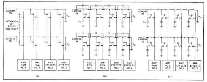
FIG. 1—Direct switcher (A) is unisolated while bridged T (B) and M-derived (C) switchers are isolated
