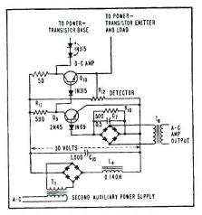
FIG. 3—Detector and d-c amplifier section used with 400-cps power supply
