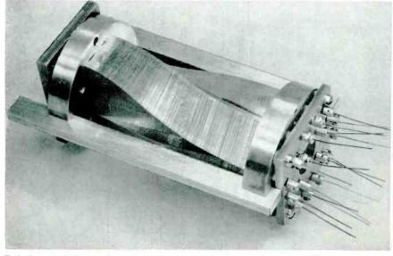
End plates hold laminations of four-waveguide twisted section in vise-like grip to insure precise alignment during soldering or brazing operation that fuses laminations together
