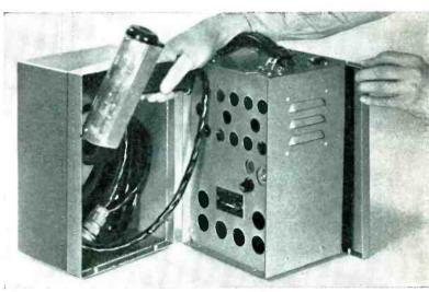
**READILY PORTABLE,** weighing only  $24\frac{1}{2}$  pounds, the unit may be carried to where it is needed. It is well suited for assembly-line use as well as for service testing in the field wherever alternating current is available. Leads and probe may be stored easily in rear of control cabinet.
