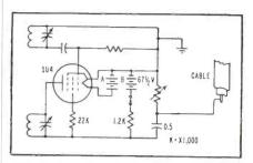
FIG. 3-Circuit oscillator for cable fault detector
