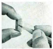
Slips of glass coated with lead sulfide give 10,000 times as much sensitivity to certain infrared rays as previous laboratory devices. Known as Kodak Ektron detectors, they are expected to find use in automatic control of chemical processing plant operations. The multiple array shown comprises 20 light and heat detectors mounted on a sheet of glass. They are intended to operate complex circuit combinations in response to projected patterns of radiation
