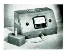
SHORTED TURNS INDICATOR tests coils in fast operation
