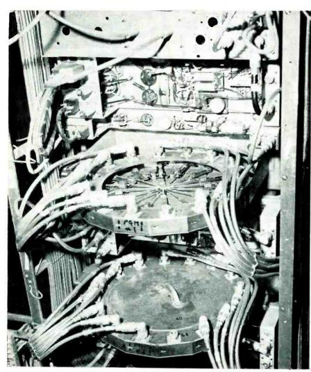
Centripetally-oriented video relay panel minimizes bus capacity and crosstalk while permitting input-output transfer within 0.001 m $\mu s$  at 3.58 mc
