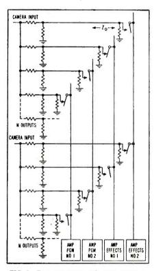
FIG. 3—Resistive video splitting pads provide a transient s/n ratio of about 30 db below signal level during overlap
