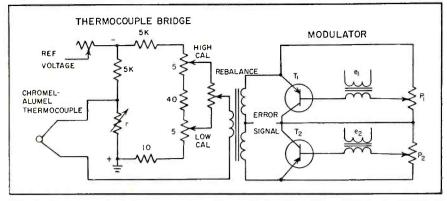
FIG. 2—Thermocouple bridge and modulator unit provide error voltage to transistor servo-amplifier
