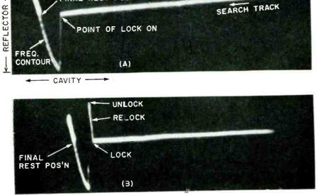
Klystron control plane and handling of evasive transient
