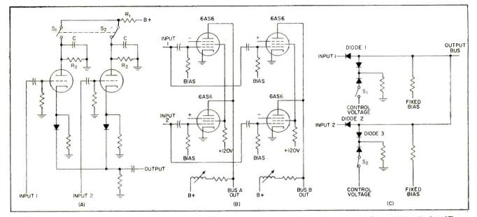
FIG. 5—Electronic switching systems remove plate voltage (A), vary suppressor grid bias (B) and use diodes in place of tubes (C)
