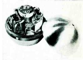
Falling-sphere air density measuring equipment. Electromagnet is at center. Teflon-separated sections of sphere serve as dipole for transistor oscillator
