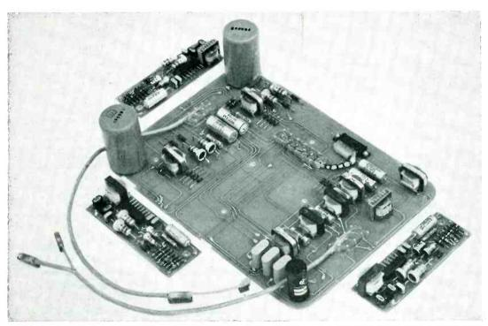
Main assembly board contains two complete 7.5-watt servo amplifier channels and a 0.75-watt channel plus related switching circuits. Subassembly boards contain complete amplifier except for output transformers
