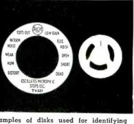
the operator merely needs to check the type of trouble observed. These notations are: CUTS OUT; IN-TERM. NOISE; WEAK; HUM;
