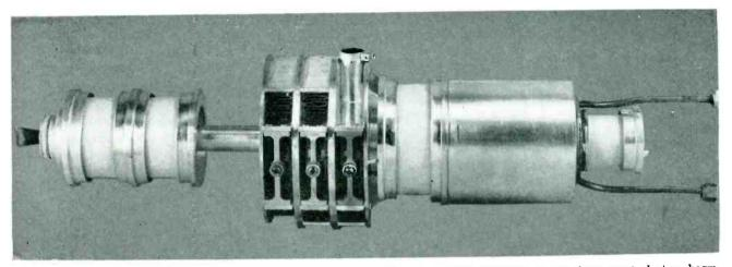
Klystron designed for high-efficiency ssb operation has segmented collector to obtain maximum energy from spent electron beam
