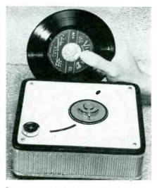
Japanese ingenuity is displayed in the transistor record player shown above. The pickup presses against the underside of the record, which is effectively locked onto the turntable. According to Sony engineers, the motor requires 50 and the amplifier only 15 milliamperes.
