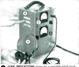
**LEAK INDICATIONS** given by a variable-pitch loudspeaker (A), earphones (B), and instrument dial (C) assure a true leak signal. Unit pin-points leaks too small to be found by older methods. Earphones may be purchased from your radio-supply dealer.
