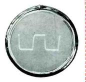
Single transient pulse, 20 microseconds wide with a one microsecond rise time, showing writing capabilities of one million inches per second. This photo was taken in full daylight without a hood.
