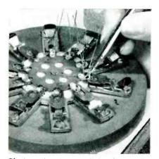
Placing wires in ceramic headers on 10position fixture
