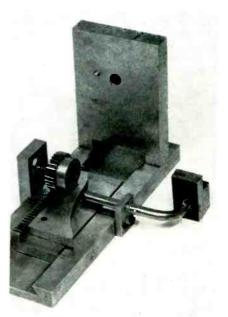
Inside view of attachment. Pinion gear is keyed to lead screw when in place on lathe and drives racks fastened to cam plate. Curve of cam plates displaces round bar. Blocks transmit resulting nonlinear motion to tool holder carriage
