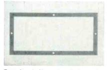
Example of  $\frac{1}{2}$  x 1 inch lamination punched from 0.005-inch brass for use in precision X-band waveguide twists
