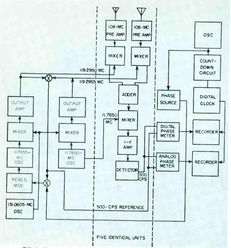
FIG. 3—Main tracking station equipment on the ground requires separate r-f-throughdetector sections for each pair of antennas
