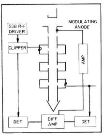
FIG. 4-Balanced feedback applied to klystron produces high-efficiency ssb power at ultrahigh frequencies
