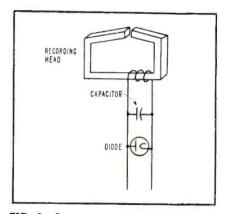
FIG. 5—One arrangement of recording head for fast, broad-band signals
