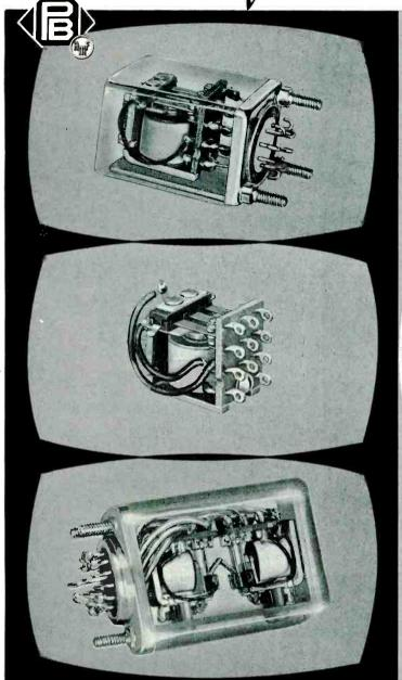
A three-pole, hermetically sealed version of the KM provides a multiplicity of action yet requires a minimum of space. Mounted with three #6-32 studs; eight solder terminals. This relay is especially useful in low voltage, DC applications where size and weight are critical factors.
