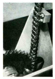
Method of anchoring tray bracket on chain. Below is idler sprocket wheel for preventing side sway
