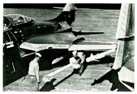
SIDEWINDER with infra-red guidance system is loaded aboard Navy plane as . . .
