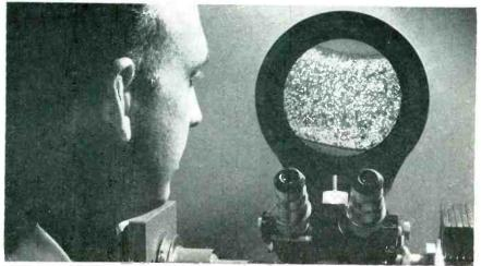
Grain structure of a fertite is magnified 300 times and projected on a viewing screen by GE scientist R. W. Johnston. Rings of the material having a diameter of 1/125 inch are now in use for electronic computer memories (*Continued on page* 194)
