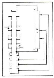
FIG. 3-Segmented collector klystron
