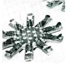
Loaded fixtures go into infrared oven for curing of epoxy bonding material
