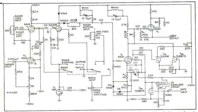
FIG. 1-Radar, Rafax, mapping and marker signals are amplitude-controlled, mixed, peak-limited and equalized in control-console
