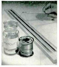
New "Dutch Boy" mercury bath inspection does away with trouble-making "skips" in core continuity of rosin core solders.
