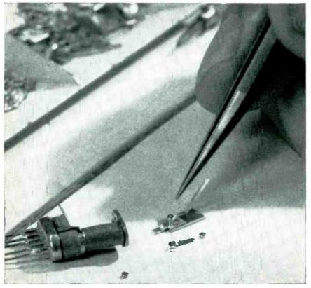
Tweezers point to banking pin (watch industry term) which runs through relay armature to prevent it from jumping out of position. Coil has already been mounted on relay header and armature goes on next
