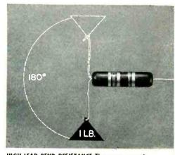
HIGH LEAD BEND RESISTANCE The new capacitors withstand one-pound-vertical-pull test moving the body of the unit 90°, then 180° in the opposite direction, then back 90°, to the original vertical position.
