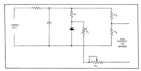
FIG. 1—Reference-voltage circuit using silicon diode has less than 0.03-percent change in output in more than 10,000 operating hours
