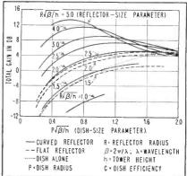
FIG. 3—Total gain characteristics of passive reflector systems
