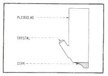
Delayed shear-wave transducer used to check thin-wall pipe
