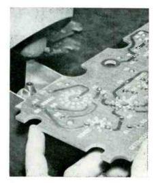
Both upper and lower staking dies are heated when wiring is on both sides of board. Only upper die need be heated when wiring is on one side
