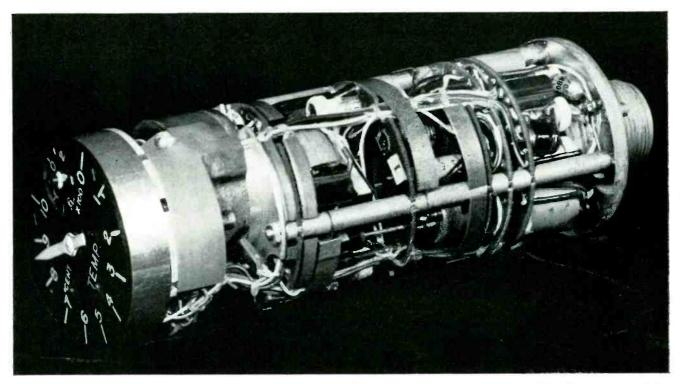
Transistorized temperature indicator occupies space of 17 cu in. behind instrument panel as compared to 75 cu in. for vacuum tube unit. Power consumption is about 7 watts and weight is less than a pound
