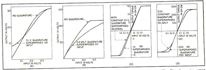
FIG. 4—Curves show output-input voltage characteristic of 0.75-watt system (A) and 7.5-watt system (B). Also shown are output torque-input voltage characteristics for the 0.75-watt (C) and 7.5-watt (D) systems
