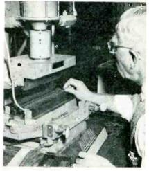
Manual loading of components, as required when loading different components in a predetermined sequence. Press can operate only when one hand is on each control button in foreground
