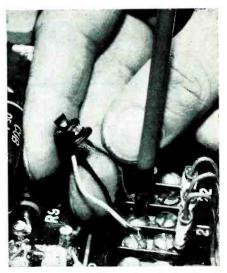
Installing transistor in control section of regulated power supply. Screw mounting is used for low-power transistors
