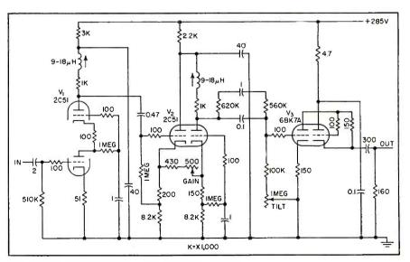
FIG. 4-Video preamplifier used in switching systems
