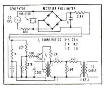
Circuit shows transistor converter to supply 1,600-cps ringing tone
