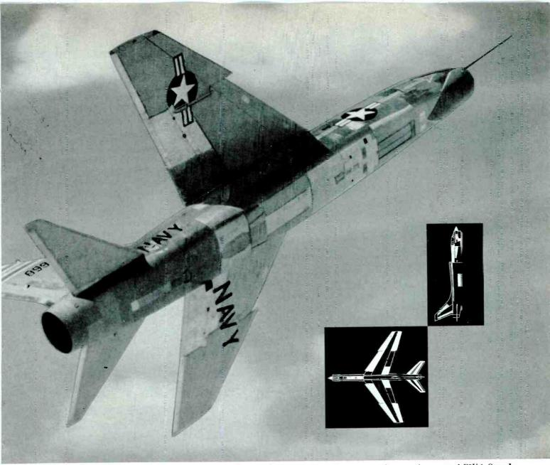
Weight-saving magnesium sheet (white areas) is used for leading edges, empennage, wheel doors and many other parts of F8U-1 Crusader.
