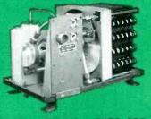
MODEL B/HT-210, TYPE 200 DIS-SIPATION: 1500 watts. ALTITUDE RANGE: see level to 10,000 feet. POWER REQUIRED: 208 volts, 400 cycle, 3 phase. WEIGHT: 35 pounds. SIZE: 1114" x 194" x 1214" high.
