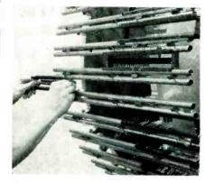
Loading component magazine onto rotating magazine carrier of machine
