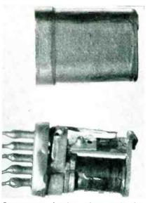
Appearance of relay when ready for hermetic sealing in transistor-size housing at top. Relay body is  $\frac{1}{2}$  inch long and coil is only  $\frac{1}{4}$  inch long
