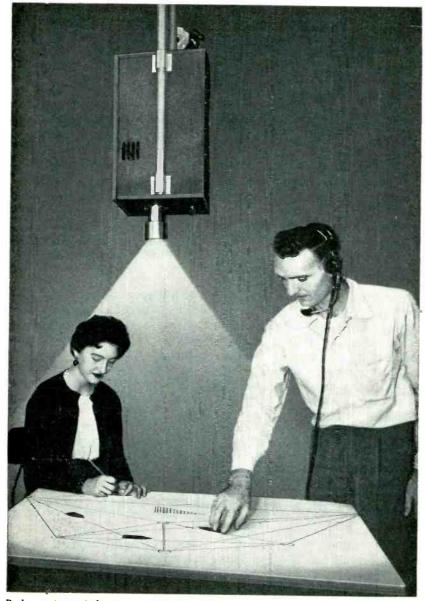
Radar projector indicator as used with plotting board for air traffic control
