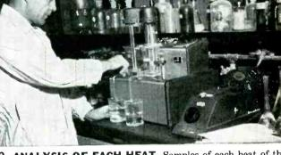
**2. ANALYSIS OF EACH HEAT.** Samples of each heat of the alloys are sent to Superior's metallurgical laboratory for extensive chemical and physical analysis. Metal must conform with rigid specifications before acceptance.
