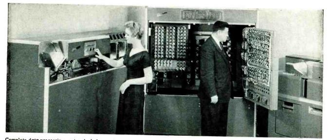
Complete data-processing system includes sorting and sensing unit (left) memory and translating unit (center) and readout unit (right)
