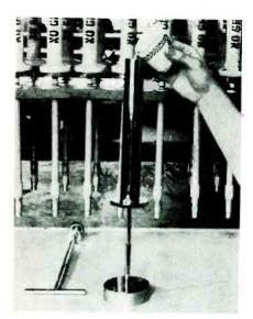
Method of supporting applicator while pouring in isocyanate and catalyst. Brass plunger of applicator, on bench at left, has good slip fit. Antennas awaiting filling are on rack at rear
