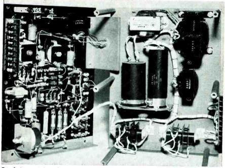
Regulation-control section of power supply shows terminal-board wiring with control transistors mounted on screw terminals and power transistor on heat sink at top center
