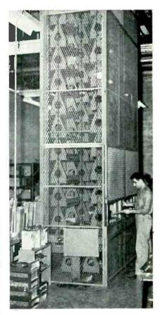
Storage unit rises 18 feet above plant floor, yet gives access to any one of 50 trays in a few seconds. Stock clerk is pushing motor control button. Trays were formerly stored under workbenches or in piles on floor as at left
