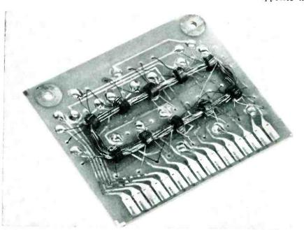
Digital memory plane unit, shown schematically in Fig. 3, has 10 magnetic cores
