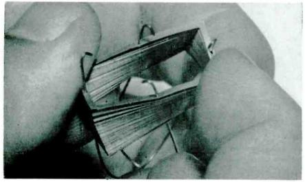
Stack of laminations is strung on four wires to insure alignment. Twisting in manner shown here gives desired uniformly gradual curve while keeping end laminations parallel to each other
