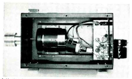
Inside view of projector unit shows last stages of video amplifier and latron
