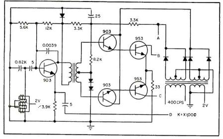
FIG. 1—Amplifier, supplied by unfiltered, rectifier a-c, drives either push-pull transformer or saturable reactor shown in Fig. 2
