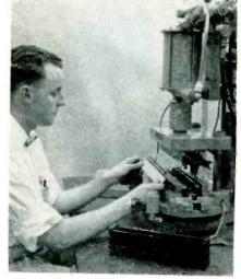
Bulk loading of components into empty magazine on press that shears and forms leads in one operation
