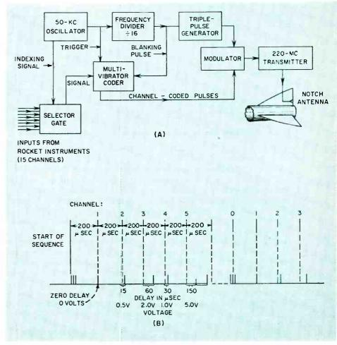
FIG. 5—Rocket telemetering system (A) uses instrumentation output to delay triggering of multivibrator in proportion to voltage level as shown at (B)
