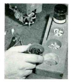
Method of changing plastic cups in partsholding tray. Jar at rear contains fungicide that is applied to terminals with brush
