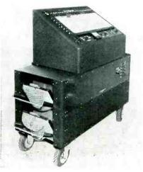
patchcords. Therefore, the terminations of an aircraft's electrical system can be connected, with simple cables, to the terminals of the analyzer without reference to circuitry. The desired circuitry can then easily be set up on the plugboard. Circle P7inside back cover.
