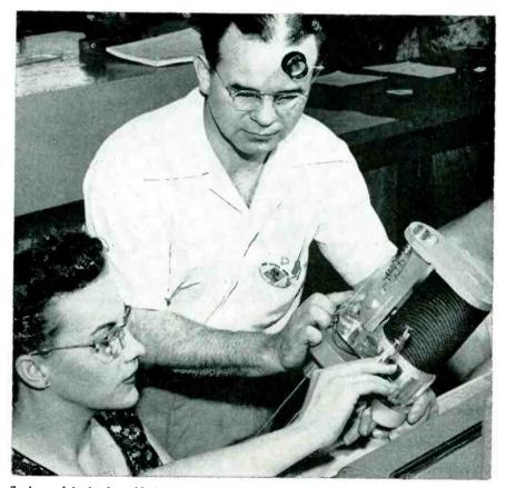
Scale model of relay, 20 times actual size, aids in training operators to make delicate adjustments of contact screws, so small that over 8,000 are needed to fill a thimble
