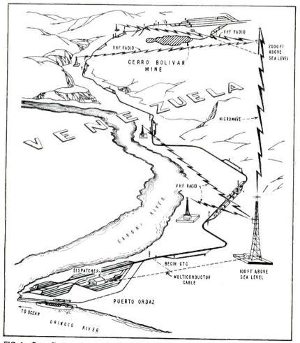
FIG. 1—Overall view of centralized-traffic-control system used between Puerto Ordaz and Cerro Bolivar
