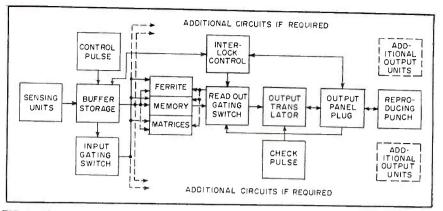
FIG. 2—Block representation of dot-code sensing and translating system
