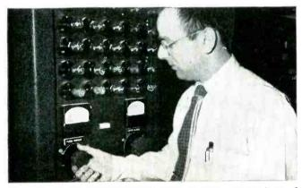
**3. TESTED IN ELECTRON TUBE.** Samples of each heat of Cathaloy are fabricated into cathodes and assembled into ASTM standard diodes. They are operated under controlled conditions. These tests evaluate each heat for emission and sublimation characteristics. Satisfactory results approve the heat for production.
