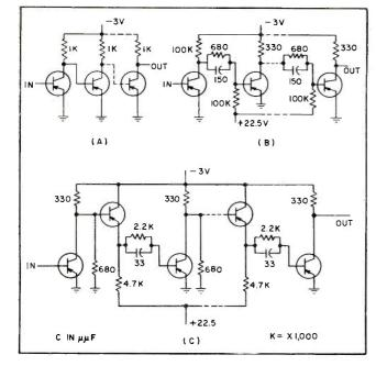
FIG. 1—Direct-coupled (A), resistance-coupled (B) and emitterfollower-coupled (C) pulse amplifiers coupled in cascade
