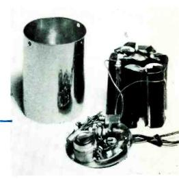
Transistor oscillator for satellite tracking is shown with silver-cell battery pack. Single high-frequency transistor is at rear center of plate
