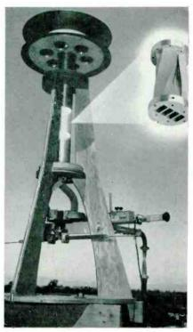
Four-waveguide twisted section, shown in inset at upper right, is mounted within tube supporting antenna of instantaneous direction finder that receives radar signals from all directions simultaneously over wide frequency range to determine direction of enemy pulsed radar
