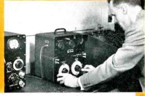
Matching Components to Close Tolerances To select or to check matched pairs of resistors, capacitors or inductors, the pair are simply connected to the two terminals. The bridge directly indicates the difference in impedance and dissipation factor between the two.
