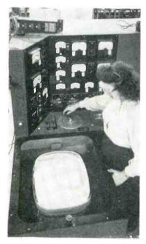
Special test set for picture tubes. Operator swings crank arm on table to 18 different detent positions in turn and observes screen or reads meters
