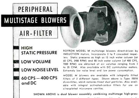
SHOWN ABOVE is dual blower assembly combining multistage high-pressure blower and a conventianal centrifugal blower, driven by one single induction motor, representing special assembly for use with General Electric air-cooled tetrode transmitting tubes.
