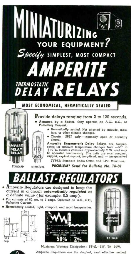
Amperile Regulators are the simplest, most effective method for obtaining automatic regulation of current or voltage. Hermetically sealed, they are not affected by changes in altitude, ambient temperature (-55° to +90°C), or humidity. Rugged; no moving parts; changed as easily as a radio tube. Write for 4-page Technical Bulletin No. AB-51 AMPERITE CO. Inc., 561 Broadway, New York 12, N. Y. In Canada: Atlas Radio Corp., Ltd., 560 King St. W., Toronto 2B
