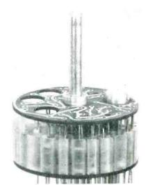
Top plate is now in position and pin 2 threaded into pin I
