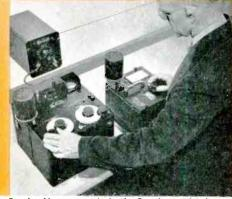
Precise Measurements in the Development Lab Where the impedance of a component must be determined with a high degree of accuracy, a precise substitution measurement can be made against a standard whose value is close to that of the unknown.
