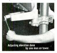
• Two lead-screw systems permit continuous, stepless adjustment in azimuth and elevation by one man on the tower with only a hand wrench.
