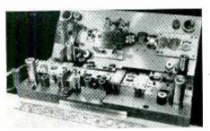
ACCURATE DIES-Volkert-built multi-stage dies like this "13-stage progressive" for stamping control covers assure uniformly high quality in long production runs for many manufacturers.
