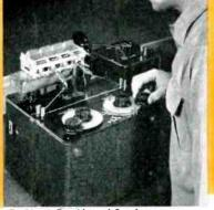
To Check Tracking of Condensers Ganged potentiometers or condensers which must track each other within a given tolerance can be checked with a high degree of accuracy and ease with the Comparisor Bridge. Each section of a two-ganged unit is connected across each bair of terminals — the units are then checked in a second or two by rotating them through their range while watching the cachode-ray-tube. Checking is continuous over the whole range.
