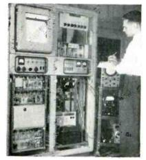
Laboratory technique employing a mass spectrometer at Baton Rouge, La., automatically sorts and identifies oil molecules for Esso research chemists. Such work was formerly done manually, which required obtaining samples and testing them individually. Adapted to operate as a robot, this electronic assembly now provides a continuous, graphic analysis of petroleum products. The general approach is said to hold promise for future use in actual refinery operations
