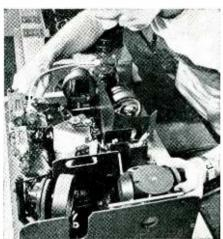
Assembling a Perkin-Elmer Infrared Spectrometer
