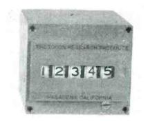
ated counter that adds or subtracts from 0000.0 to 9999.9 when magnetic pulses are applied to add or subtract terminals respectively. Each wheel may be individually set to any predetermined number. Typical applications of this continuousduty-cycle counter are for net pulse counting in pulse guidance systems, and for the remote indication of net totals in any reversible system.
