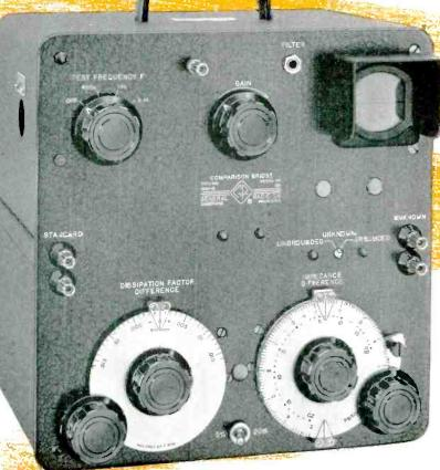
The Comparison Bridge uses the highest quality components, including a specially designed doubleshielded bridge transformer, and bridge ratio arms which incorporate the best precision resistors G-R knows how to make.
