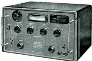
Typical of the best in current design is the Muirhead-Wigan D-650 decade oscillator covering lc/s to 111,100c/s with a frequency accuracy of  $\pm$  0.2% or  $\pm$  0.5c/s.
