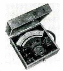
ingly high torque-weight ratio that eliminates pivot friction as a factor. The instrument is a milliammeter down to 1 ma full scale; an ammeter, up to 10 amperes full scale; and a voltmeter, down to 1 v full scale and up to 1,000 v full scale. A 4-page folder, entitled "Electrical Measurements," Vol. 21, No. 7, gives complete technical data.
