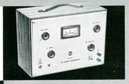
The new WR-86A UHF Sweep Generator is recommended for continuous production-line testing and for general service applications on color and black-and-white TV receivers, converters, tuners, filters, antennas, transmission lines, and other equipment operating in the range from 300 to 950 Mc.
