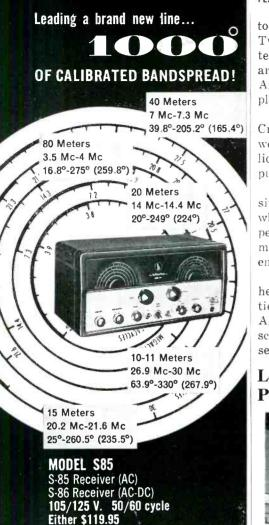
We here at Hallicrafters are proud of our new communications line, especially the new S-85 receiver with over 1000° of calibrated bandspread. Broadcast band 540-1680 Kc and three shortwave bands 1680 Kc-34 Mc on large easy to read dial. Separate bandspread tuning condenser and built-in speaker. Seven tubes plus rectifier. Coupon below brings complete specifications.
