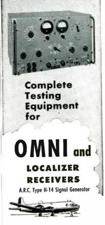
For a quick and accurate check by pilot before take-off, or for maintenance on the bench, this is the favored and dependable instrument. Checks up to 24 omni courses, omni course sensitivity, to-from and flagalarm operation, and left-centerright on localizer. For ramp check, RF output 1 volt into 52 ohm line; for bench checks, 0-10,000 microvolts.
