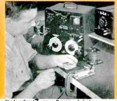
Winding Exact Turns on Precision Inductor Several manufacturers have rigged up devices to continuously measure impedance of precision inductors as they are actually being produced. One or two excess turns are purposely wound on the core — the "unknown" terminals are connected to the winding ends through a special jig — then, as turns are removed, the cathode-ray-tube continuously indicates the approach to the desired value. Components with 0.1% accuracy are easily wound in this manner.
