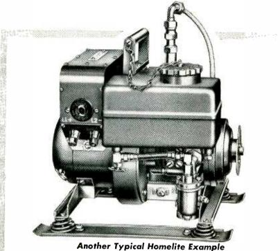
This is the first generator of this size procured to meet the requirements of MIL-G-10286A(CE) and the requirements of the reference engine specification MIL-E-11275A (CE). Only 22 pounds complete, it has a military rating of .15 KW, 120 V., 60 cycle, 1 Phase, 1.0 P.F. reconnectable to 120 V. DC. One
