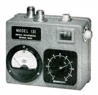
The model #131 "S" Band Wavemeter (Amerac's version of the popular military model TS-117) covers the frequency range from 2400 MC to 3400 MC in 16 revolutions of the micrometer thimble, by either the transmission or absorption method.
