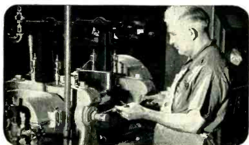
Milling the rubber-like compound which is subsequently molded over Titeflex flexible waveguides to protect them.
