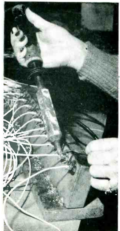
Jig for holding phono-type plugs while soldering leads to outer skirts of plugs for use as speaker cables. Plugs were previously soldered to the center conductor at a dip soldering operation
