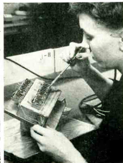
This chassis support jig rotates on an angle-cut pedestal. Spinning the jig changes the angle as required for optimum work with the pencil-type soldering iron
