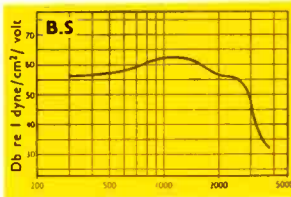
MME/G (B). Constant input of 0.2 volts. Sound pressure measured in artificial ear of 1.5 cubic centimetres and 240 ohms acoustic resistance.
