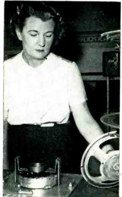
Operator demonstrates use of fixture for applying ring of red thermosetting cement to speaker frame for anchoring spider. When she releases lever in right hand, the ring and its strap iron side supports will drop down into the pot to pick up cement for the next speaker
