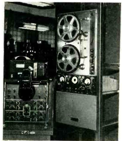
Test setup for evaluating short sample method of measuring flutter introduced by magnetic tape recorders used in guided missile instrumentation. Discriminator is on panel below tape recorder. Dual-beam oscilloscope and recording camera are at left
