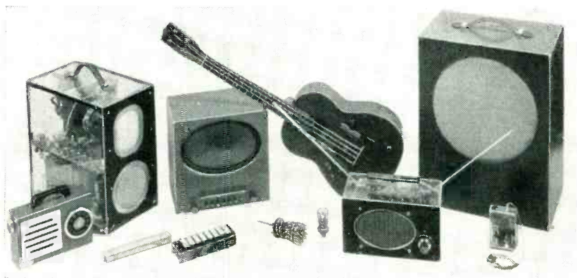
Group photo shows many of transistorized items described in text. Left to right in rear are, portable radio, tv receiver, auto radio, ukulele and public address amplifier. Front row shows roving microphone, toy organ, decade scaler, complementary symmetry audio amplifier, portable f-m receiver and paging receiver
