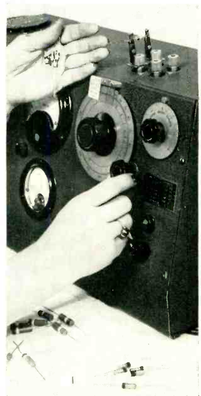
Testing small choke coils by using calibrated terminals on top of Q meter
