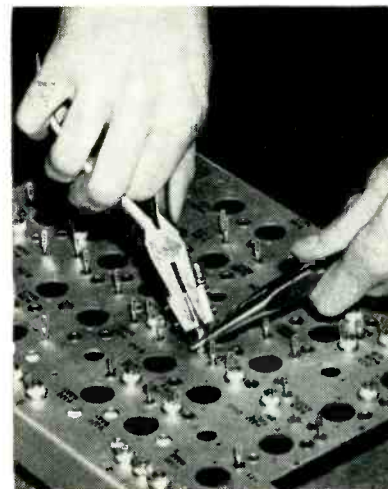
Method of holding tools for stripping insulation close to chassis
