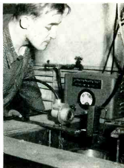
Experimental setup of optical thermometer, here aimed between turns of work coil to measure heat of test sample inside
