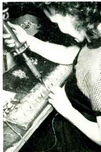
Recessed jig for trimmer subassembly work
