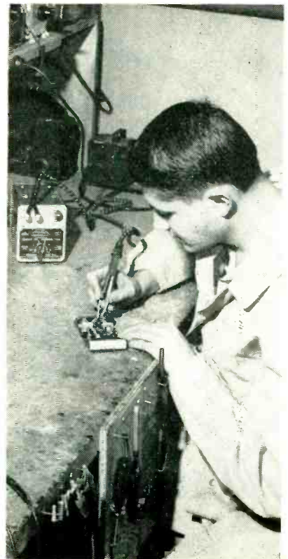
Use of tweezers for soldering a small joint in an experimental hearing-aid unit in an MIT laboratory. Tool rack fastened to front edge of bench keeps most-used tools within reach and encourages putting each one away when work with it is finished. Loop of wire inserted in edge of bench is support for clip leads
