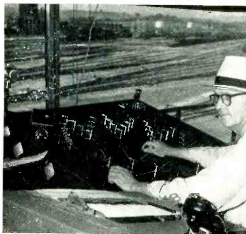
OPERATOR in freight-yard control tower (left) engages remote car-retarder when speed meter (right) warns that coupling speed is unsafe as . . .
