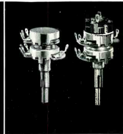
Centralab Model 2 Radiohm. Left, twin unit plain type, front section tapped; Right, twin unit switch type, rear-section tapped. Concentric shafts.
