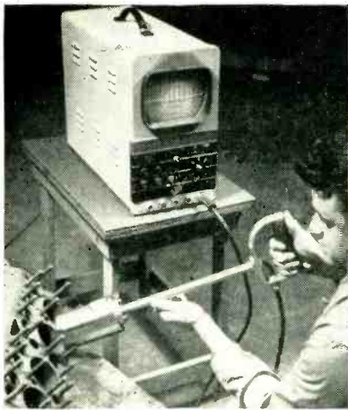
FIG. 1—Thickness-measuring instrument being used with special jig-holder device to determine cylinder wall thickness in automotive engine
