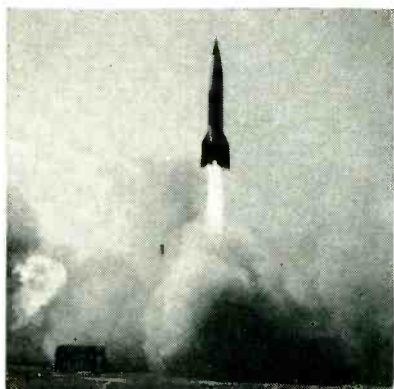
GERMAN V-2 (left) carried its 2,000-lb warhead 250 miles at 3,600 mph; multistage rocket gains range when 'Wac Corporal' in V-2's nose is fired at top of trajectory (right); intercontinental missiles seem closer today because...
