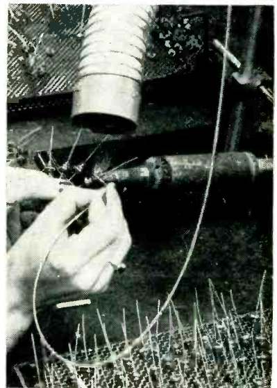
Vacuum-system duct used to pull off soldering fumes, and stand for supporting soldering iron rigidly at optimum working position
