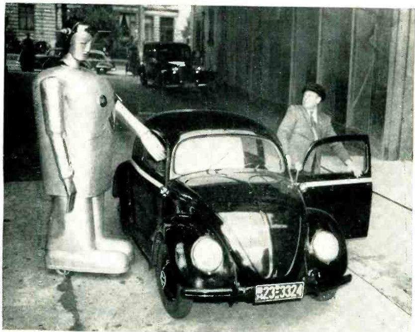
Mr. "Sabor IV" the 500-pound robot shown in the photograph, has its movements directed by a built-in short-wave radio receiver. Cost of the metal giant was $7,140
