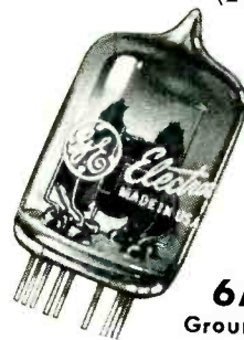
6AJ4 Grounded-grid r-f triode (2 stages)
