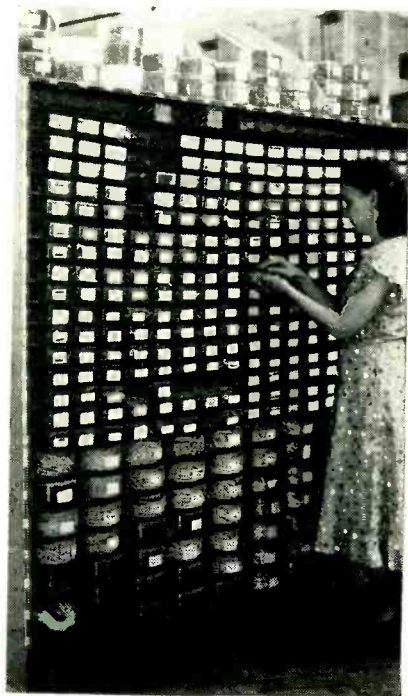
Rack for plastic boxes containing pre-cut wires
