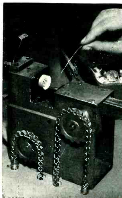
Setup for soldering antenna lead inside cavity for RCA uhf pencil triode. Solder is applied to inside wall of cavity after needle-point gas flame at right end of fixture has heated wall from outside
