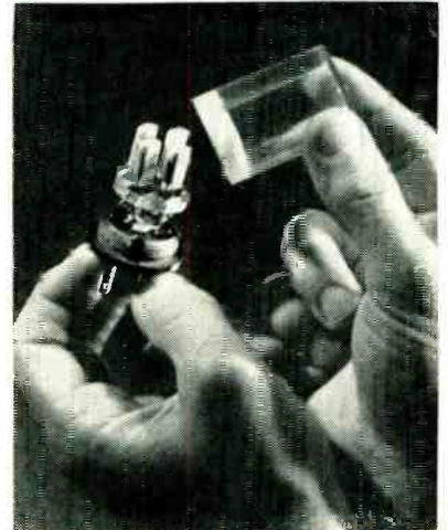
In this four-transistor audio amplifier pnp and npn types are combined to provide transformerless class-B amplification with direct coupling to loud-speaker voice coil
