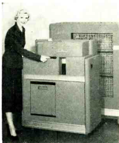
Electronic calculator made by IBM has 1,400 tubes. Over 1,000 of the machines are now used in business offices in the U. S.
