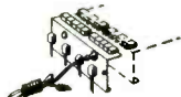
Back Connectors mount on Back Plate to give one point to check all chassis connections.
