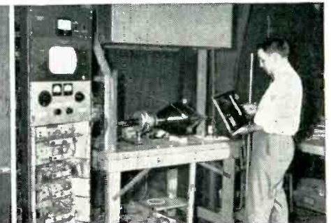
A physicist using a Rauland-developed radiation meter in checking X-ray radiations from cathode ray apparatus.
