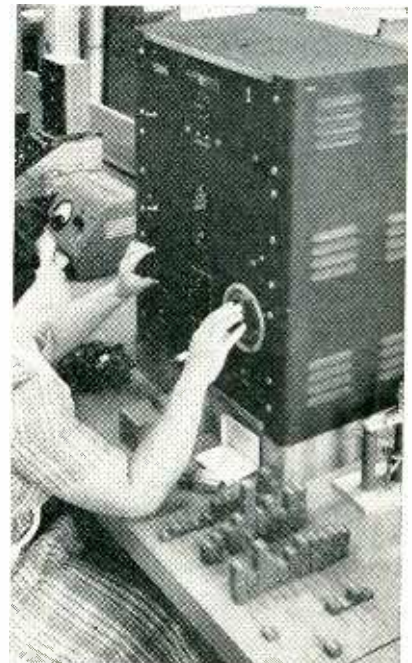
Using test bridge to check values of mica capacitors. After value is measured, operator uses rubber date stamp to stamp exact value in \mu\mu\text{f} directly on the capacitor, then places each capacitor on the stack having that value. Units on bench range from 1,947 \mu\mu\text{f} at lower left to high of 1,990 \mu\mu\text{f} at lower right, with each pile having a different value
