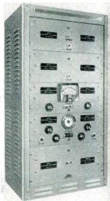
The complete equipment is housed in a single cabinet with five compartments
