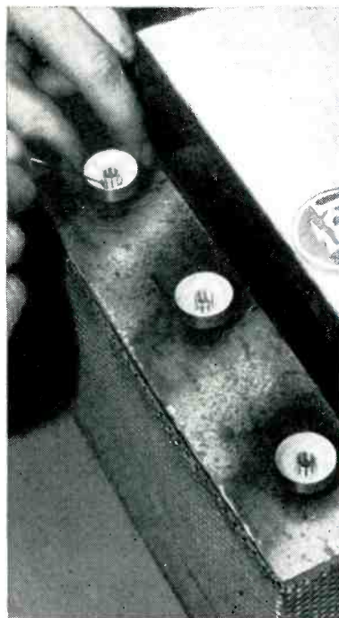
Protective metal cage encloses three vertically mounted electric soldering irons having machined tips on which three cavity sections are resting
