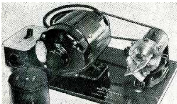
CASE HISTORY NO. 6 —Location and length of stripped wires on ignition coils had to be controlled accurately. A rotary stripper having rotating blades was adjusted to the diameter of the bare wire, and the length of stripping was controlled by an adjustable stop inside the machine. Not suitable for wires finer than AWG 24. Housing at left foreground fits over cutting blades, and wire is inserted in conical hole in end of housing. Stripping blades can be removed for sharpening
