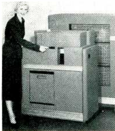
Electronic calculator made by IBM has 1,400 tubes. Over 1,000 of the machines are now used in business offices in the U. S.
