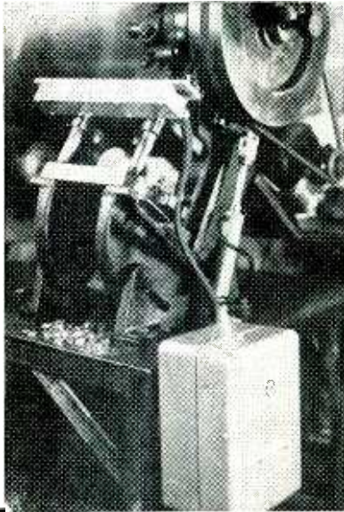
Radiation-type safety control installed on small motor-driven punch press
