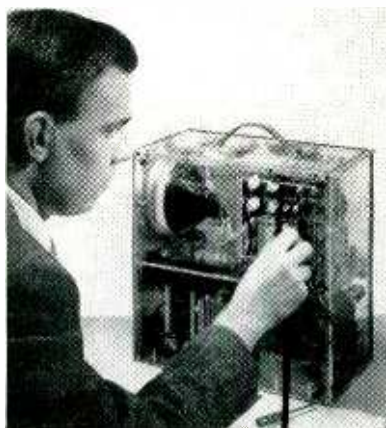
Thirty-six transistors perform all the functions in this 5-inch battery-powered tv set, except for c-r tube
