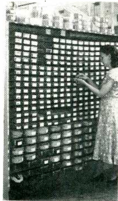
Rack for plastic boxes containing pre-cut wires
