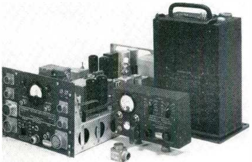
Complete system for measuring dynamic pressure under wing of aircraft in flight
