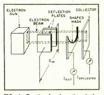
FIG. 1—Functional schematic of the beam-deflection tube
