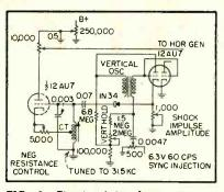
FIG. 6—Circuit of interlace generator for obtaining 525-line interlaced sweep
