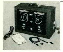
Electronic hair-removing setup consists of equipment shown. The foot-switch initiates automatically-timed pulses and controls length of manually-timed pulses
