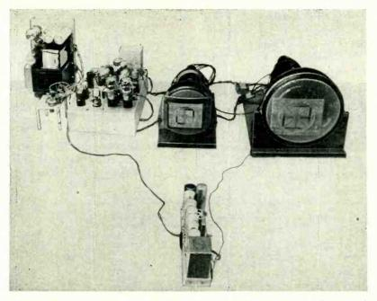
The phototube and video amplifier chassis faces test transparency on the face of the transmitting crt. For demonstration purposes the monitor picture tube at right is fed deflection currents and high voltage from the sweep chassis
