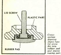
This refrigerator lid screw *might* have been made by other methods. With cold heading, however, in the hands of Scovill engineers, toolmakers and operators, this special part is produced in one piece, to close tolerances, with a better finish and greater strength, at lower cost.
