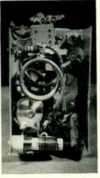
Closeup of underside of exciter **cha**ssis shows close fitting of components required. Authors advise a 12AU7 provides greater output than the 7F8
