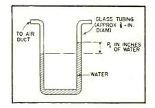
FIG. 6—Simple U-tube manometer, useful for system tests
