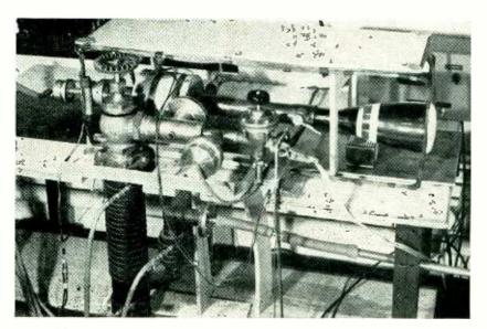
FIG. 2—Special cathode-ray tube setup for field-mapping equipment
