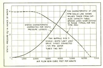
FIG. 1-Fan performance and system characteristic curves
