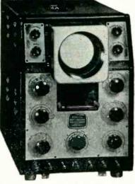
MODEL 1035 Provides FAST SWEEPS, from 150 Millisec. to 5 Microsec., and Video Frequency Amplifiers, Stepped -VE Feedback Type, with Gain of 3 at 7 Mc. Bandwidth to Gain of 3000 at 60 Ke. Bandwidth, ± 1.5 DB., *PLUS* Triggered Sweens, Suppressed Flyback, ± VE Sync.
