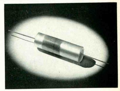
**SOLUTION:** This capacitor weighs .7 oz. It replaces a 10 lb. dry battery in a portable instrument requiring an ionizing voltage of 1900-2200 VDC. The instrument load is negligible and is due mostly to leakage of the circuit insulation. The capacitor itself must have a high enough resistance so that no more than 5% of its energy is lost in 24 hours. This problem was one of the most difficult we have had.
