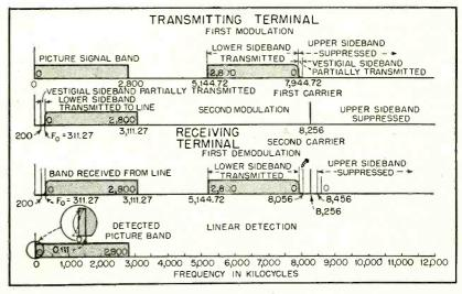
FIG. 2-Modulation diagram for television carrier terminals
