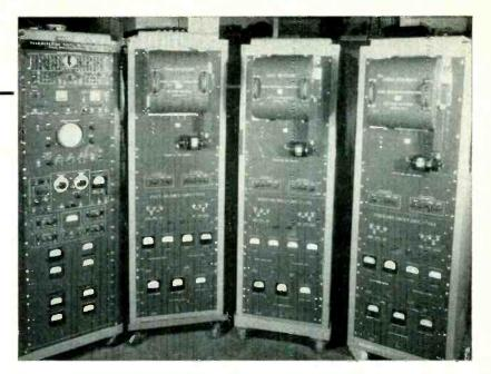
FIG. 2—Receiving station equipment employs direct video recording on continuous film strips
