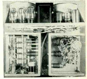
Front and rear views of the admittance analyzer with shielding removed
