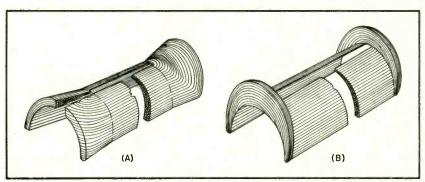
FIG. 2—Cross-section of initial experimental model of cosine deflection coil A and coil actually used in television receivers B
