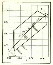
FIG. 3-JETEC color limits for P4 white phosphor
