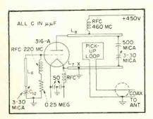
FIG. 2—Final stage of the transmitter after modification. Inductor  $L_{_{0}}$  couples to  $L_{_{5}}$  of Fig. 1
