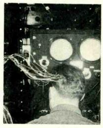
sponds in brightness to the potential at the corresponding test position. The equipment is being used by Stanford Goldman at Syracuse University in studying traveling waves in the brain.
