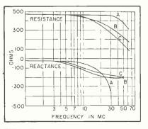
FIG.1—Resistance and reactance characteristics of MPO-17 resistor
