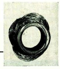
FIG. 3—Cross-section of finished cosine deflection coil
