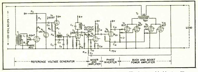
FIG. 2—Simplified schematic showing arrangement of reference generator, amplifier, inverter and buck-boost amplifier
