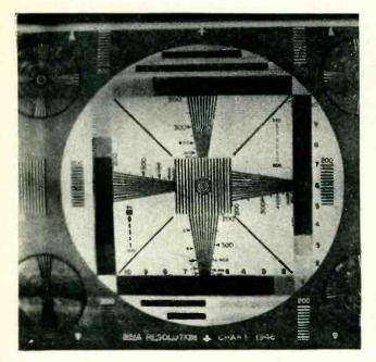
Example of interlaced resolution of standard test pattern. The gamma range is not representative because overexposure of film was made to emphasize wedges
