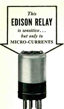
Sensitive is about the only word that can describe a relay which will operate on input powers as low as 25 micro-watts. Sensitivity also suggests lack of strength, but that's not true in this case. Electrically this Sensitive Relay will continuously withstand input powers 10,000 times its nominal ratings, and mechanically it's truly rugged. Originally developed for aircraft use, it is standard equipment on thousands of planes in the air today.
