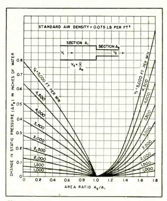
FIG. 3—Change in static pressure due to abrupt change in airflow cross-section
