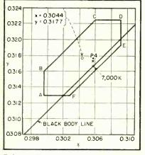
FIG. 4-JETEC specification for neutral filter face-plate glass
