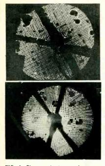
FIG. 3—Photograph at top shows no magnetic field within magnetron. Bottom view shows distortion of shadow network due to magnetic field, and a space-charge ring in central region
