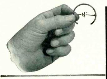
**CONVENTIONAL POTENTIOMETERS** have a coil diameter of approximately 11/2" and provide only 4" (about 300°) of potentiometer slide wire control.
