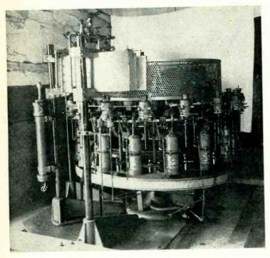
**EXHAUST MACHINE.** 16 heads. Mfd. by GE, can be converted to standard tube production. Has all controls, with trap transformer, gauges, controls for each head, timers, two Brown panel pyrometers.
