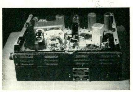
Complete transmitter-receiver for citizens band after crystal exciter has been added. Cover plates cause slight detuning of doorknob grid circuit
