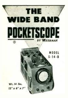
Another Waterman <u>POCKET</u>-SCOPE confirming the obsolescence of conventional oscilloscopes. Characterized by wide band amplifier fidelity without peaking as well as amazing portability. S-14-B <u>POCKETSCOPE</u> is ideal for laboratory and field investigation of transient signals, aperiodic pulses, or recurrent electrical wave forms.
