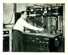
Electronic Engineering Laboratory equipment for testing emission characteristics of nickel cathode materials.
