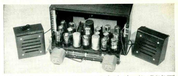
Complete automatically switched intercommunicator. Remote stations contain only speaker and annunciator pushbutton for signaling master station to originate a call. Pushbutton switches are used to insert 14-tube voice-switched master unit between desired calling and called stations
