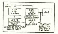
FIG. 1-Elements of the 60-cycle voltage regulator
