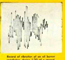
Record of vibration of an oil burner installation during 1/30 of a second, photographed on oscillograph screen.
