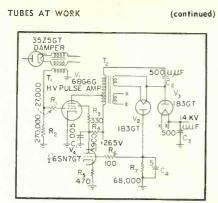
Regulated high-voltage power supply utilizes ringing current in primary of  $T_2$
