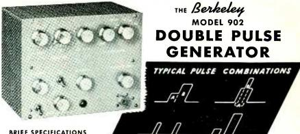
PULSE DURATION individually adjustable from 0.15 to 1.5 microseconds; RISE TIME is .05. DECAY TIME 0.10 microseconds. SPACING between pulses variable from -0.5 to +3 microseconds, REPETITION RATE adjustable in 3 ranges, 1 to 10, 10 to 100 and 100 to 1000 cycles; can be externally triggered. OUTPUT IMPEDANCE opproximately 400 ohms, maximum output voltage, -200 v. CONTROL CALIBRATION ACCURACY ± 5% over entire range.
