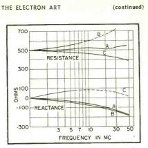
FIG. 3—Resistance and reactance characteristics
