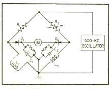
FIG. 2—Simplified schematic of inductance bridge used in ceramic thickness gage
