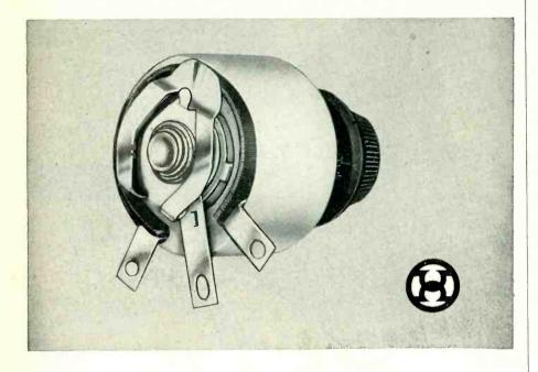
THIS COMPACT, rugged type M 25 watt rheostat offers exceptional heat dissipation. An exclusive Hardwick, Hindle feature is the lock tab which prevents deformation of the contact arm due to rough handling. Its steel stop pin will withstand over 40 inch pounds torque.
