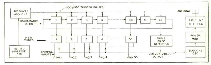
FIG. 3-At the transmitter, timing intervals are initiated by a 10-kc oscillator
