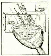
FIG. 1-Exaggerated view of picture tube and safety window shows effects of ambient light and halation
