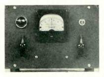
FIG. 3-Panel of the indicator contains balancing potentiometer at lower left and checking switch at lower right
