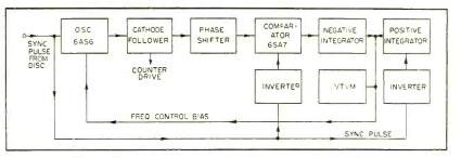
FIG. 6—Block diagram of receiving station matrix oscillator
