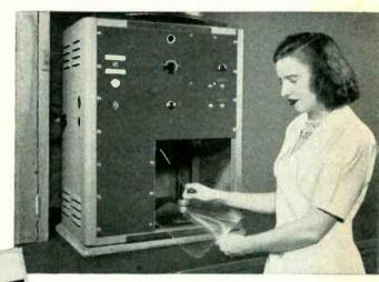
Preparing a sample for measurement of dielectric constant and power factor. Kodapak Laboratory, Rochester, N. Y.
