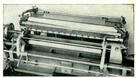
Closeup showing coil arbor in transfer position.
