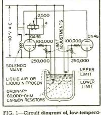
FIG. 1—Circuit diagram of low-temperature liquid level control A LITTLE ROUTINE SERVICE SAVED A LOT OF BRAZING ALLOY
