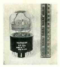
FIG. 2—Leam-deflection tube for squaring 40-mc pulses
