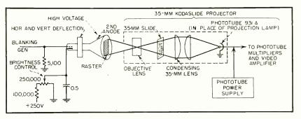
FIG. 5—Small transparencies can be accommodated by employing the optical system of a 35-mm projector backwards, with the phototube in place of the usual lamp
