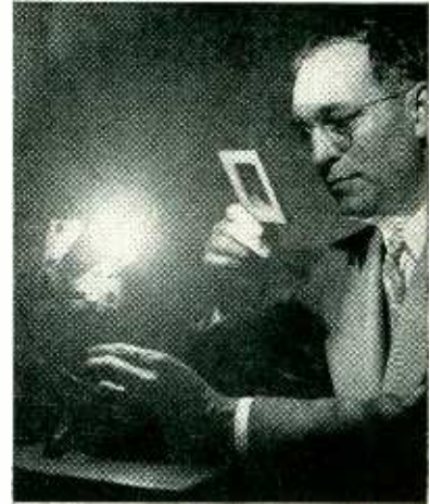
W. D. Buckingham examines new molten-zirconium arc lamp he developed, using dark filter. Intensity is one-eighth that of sun
