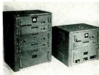
Remote control equipment used to control six relay transmitters used in the Raydist system
