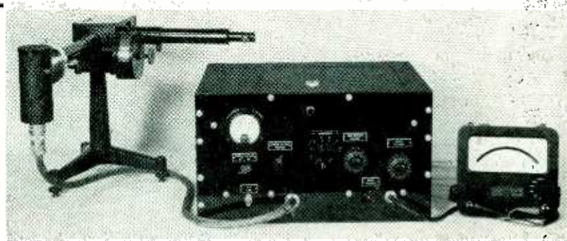
Use of connecting cables permits the pickup box and meter to be moved independently of the control cabinet
