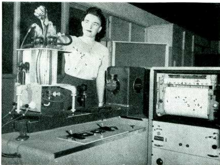
Chemist places vial of unknown solution into chemical analyzer which will print curves that can be interpreted to yield chemical and molecular properties of solution in a matter of minutes
