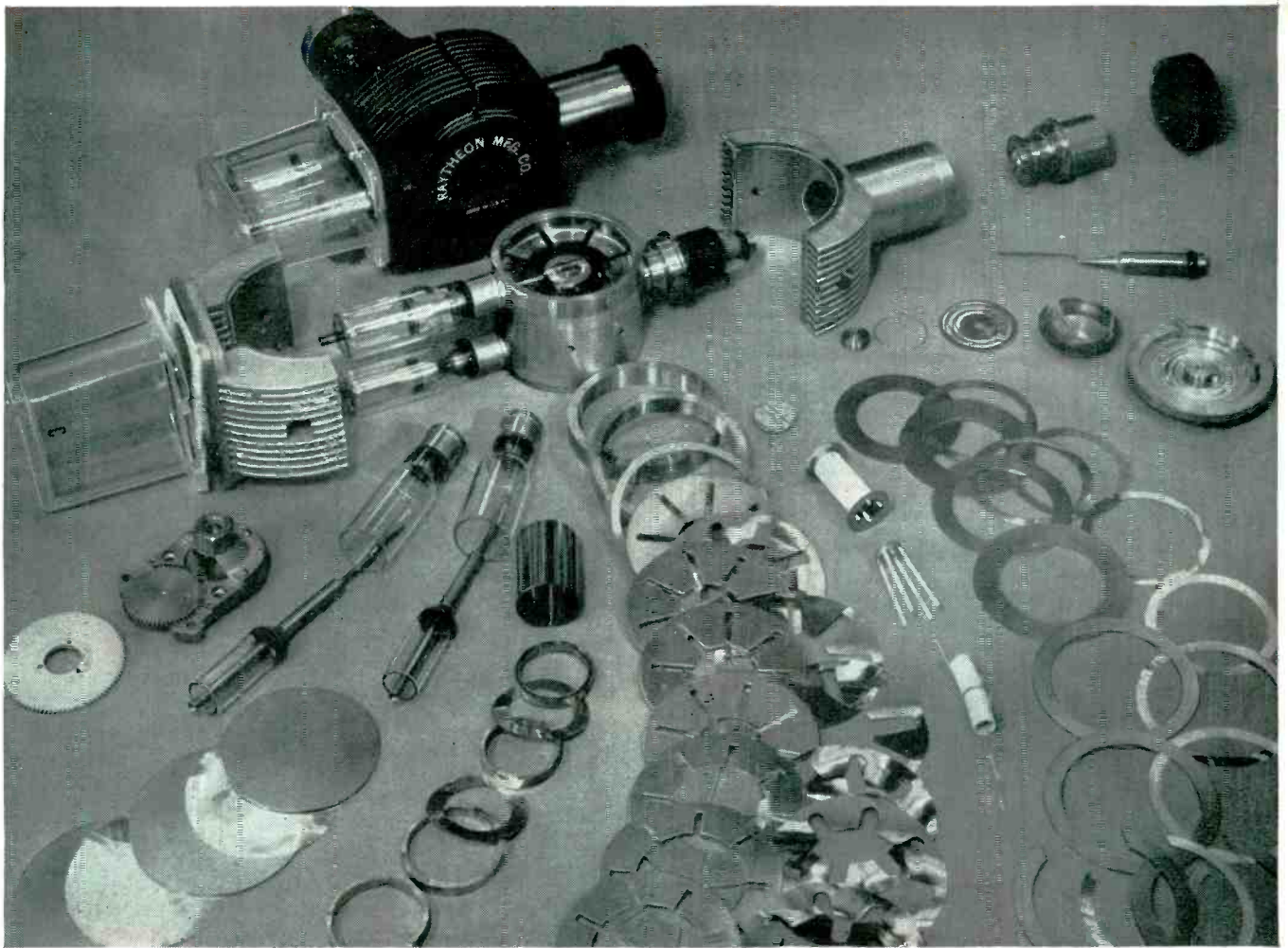
▲ One of the Magnetrons made by Raytheon Manufacturing Co., Waltham, Mass. Most of the parts shown in the foreground are OFHC Copper.
