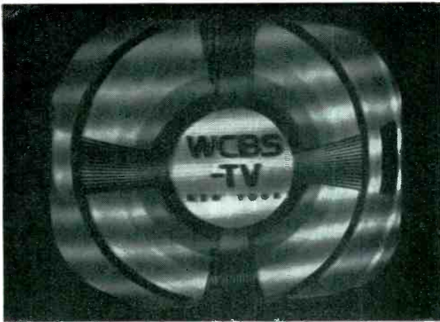
Venetian-blind effect on station 40 miles away by Baltimore station 220 miles away. The horizontal bars represent a visible beat between carriers
