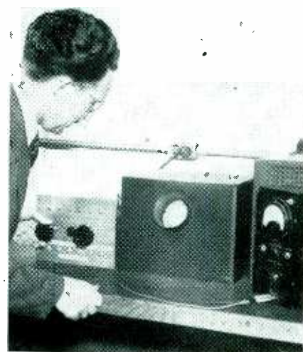
J. T. McNaney of Consolidated Vultee demonstrates his Electrontype system for producing messages or numerical results on screen of Charatron cathode-ray tube in response to coded signals applied to multiple deflecting electrodes
