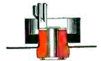
Silicone bushings and plastic cups used with capacitors 660-v a-c, or 1500-v d-c and lower.
