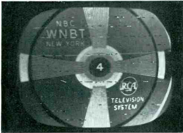
Spark-plug interference. Black streaks are spark impulses and white are torn portions of horizontal scanning line
