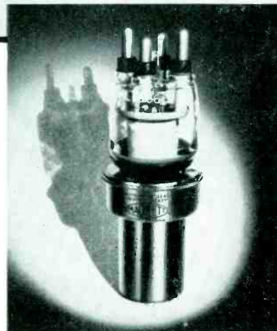
Use of the ML-5666 to replace 889A, carries the added advantage of the Machlett automatic-seal water jacket.
