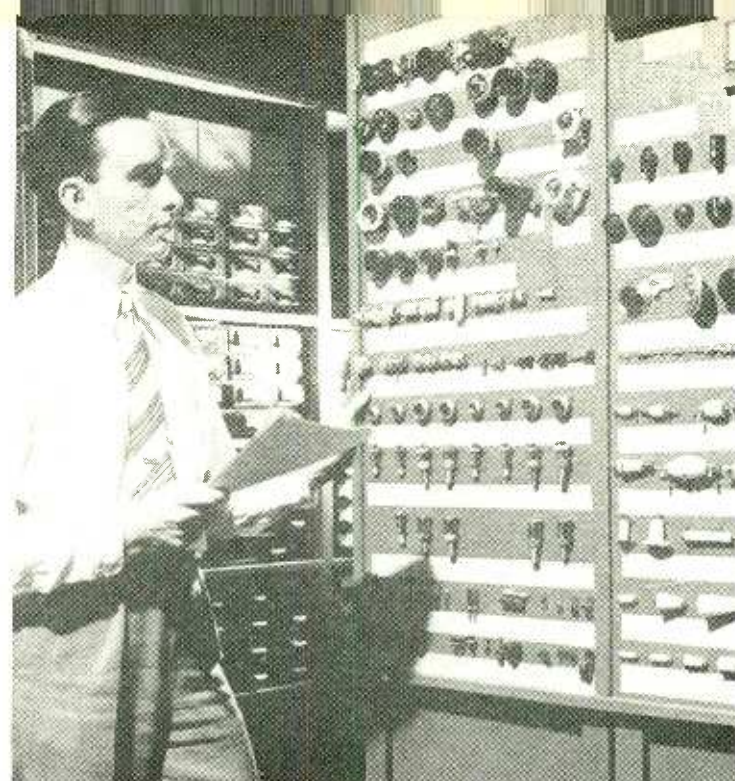
HELP-YOURSELF STOCKROOM —For engineers who like to pick and choose, this Transmitter Lab stockroom ranks tops in popularity. Cabinets have numbered drawers, and samples of parts are mounted on boards having corresponding drawer numbers
