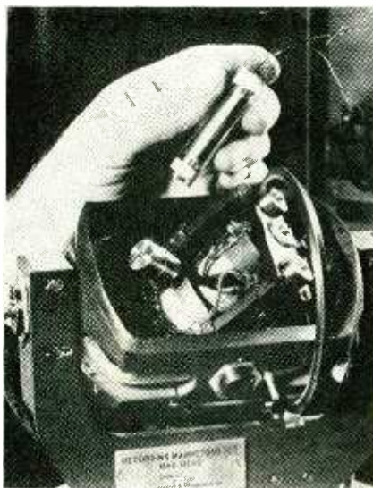
Sensing element of the airborne magnetometer and the gimbal mounting for positioning the unit parallel to the earth's magnetic field
