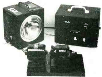
FIG. 2—The Synchrostab is used with a tachometer and a Strobotac to observe rotating machinery
