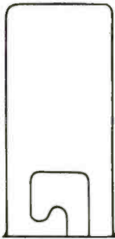
Three lengths of shield cans are available: No. 8660, height 1 3/8" No. 8661, height 1 3/4" No. 16G12564, height, 2 1/4"
