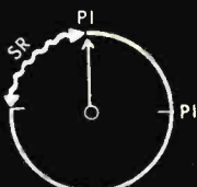
6 Three position index — two positive spring return from counter-clockwise.
