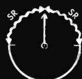
5 Three position spring return from both sides to center.
