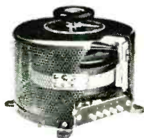
Transtat Type TH for .3 to 20 KVA —Manually operated a.c. voltage regulator providing arcless, stepless control. Brush track on coil periphery where it may be banded to insure trouble-free operation under exacting conditions of service.
