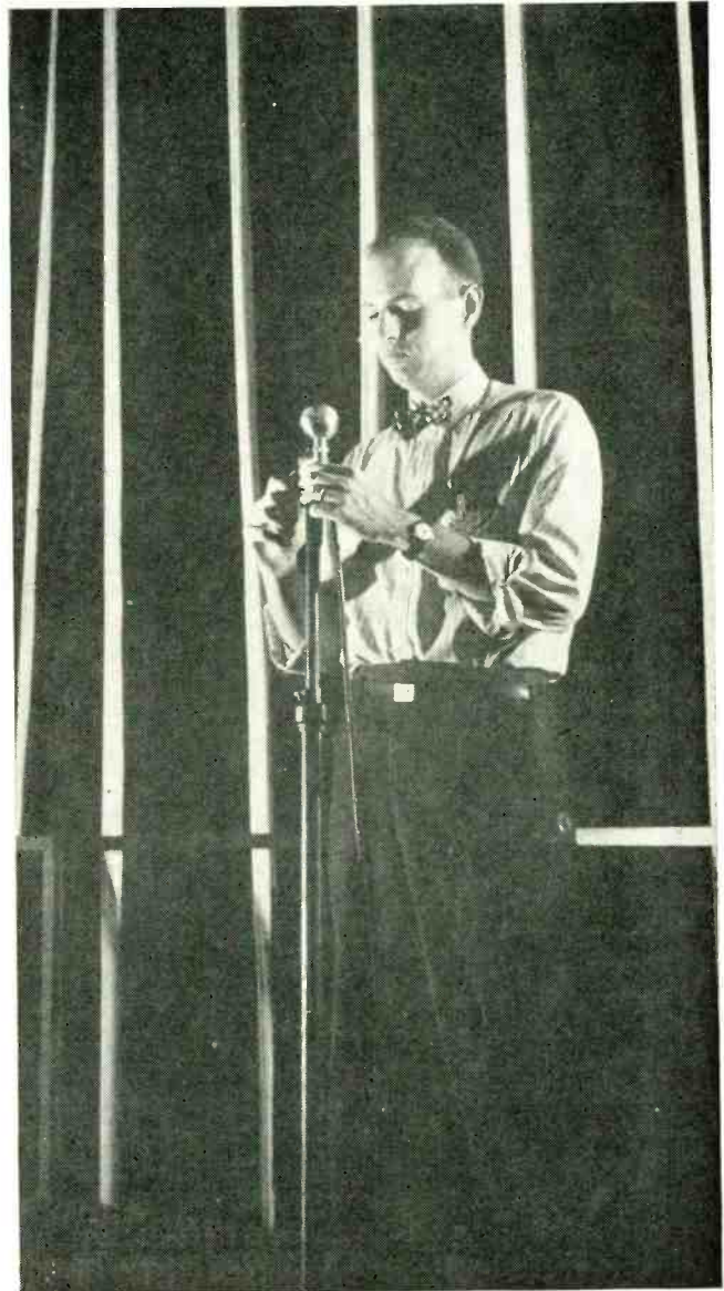
soundproof room and the measurement room, facing the microphone. A motor drive sweeps an audio signal generator gradually from 50 cycles to 20,000 cycles, while an inking pen traces on graph paper the amplified output of the microphone
