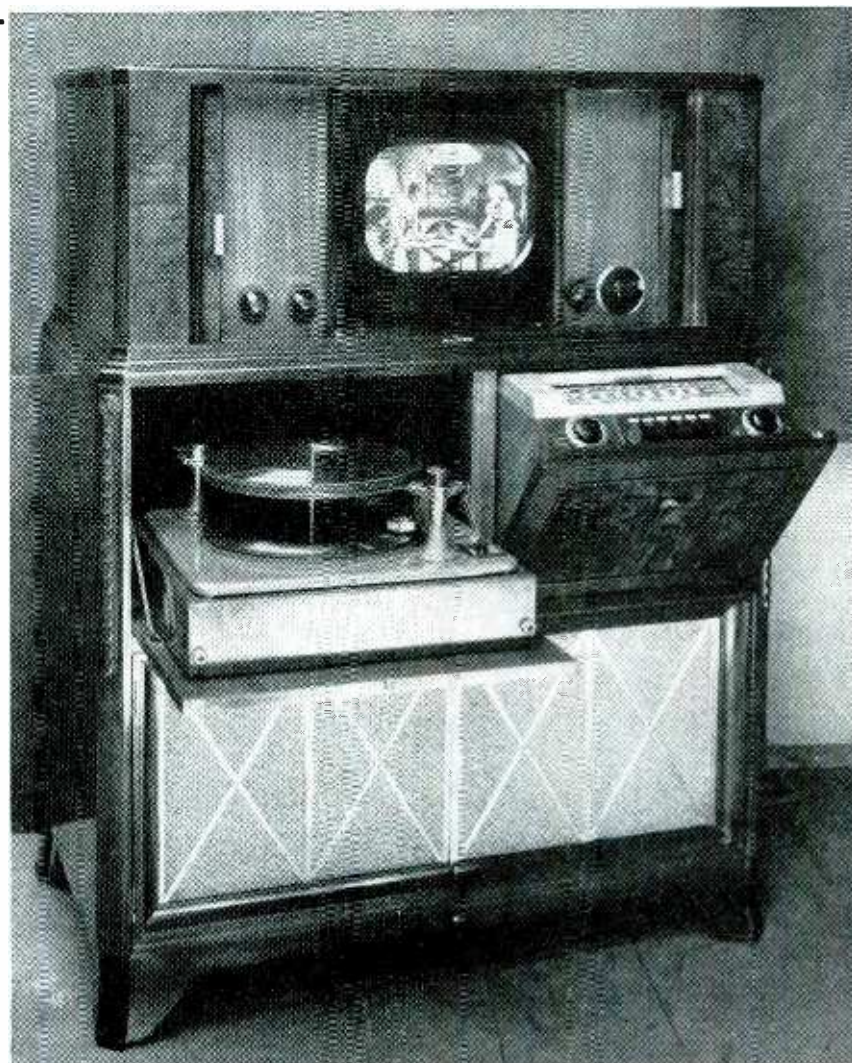
Direct-viewing combination console with ten-inch picture tube. All direct-viewing types have a safety glass panel mounted in front of the picture tube
