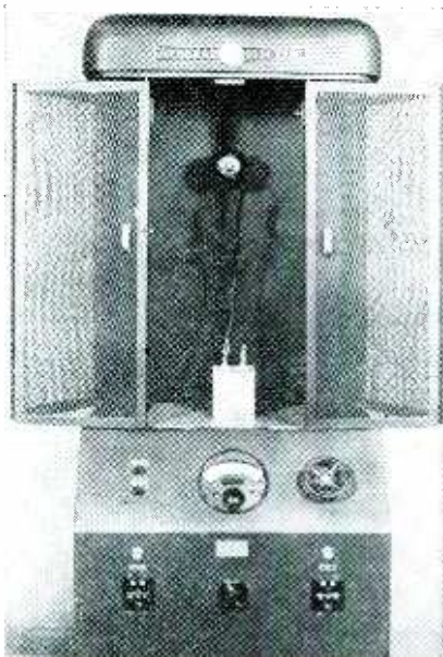
Testing of capacitors at voltages in excess of 5,000 volts is done in a test cage. Doors are closed and voltage applied. Opening doors turns off high voltage and discharges capacitor
