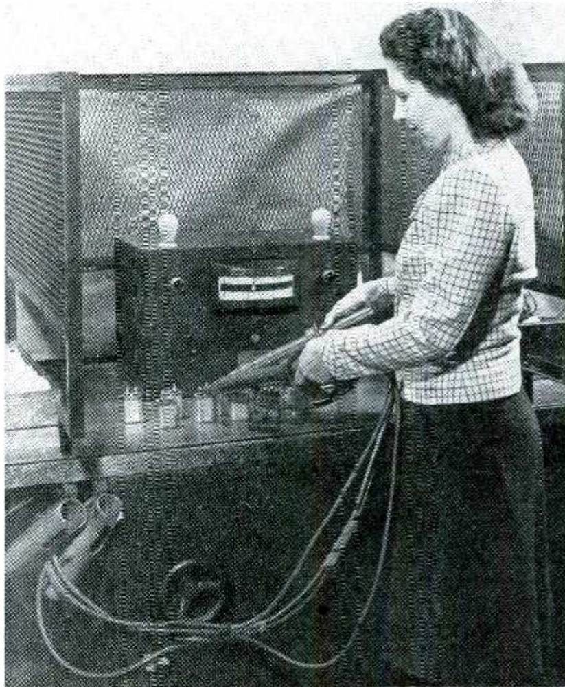
For voltage tests up to 5,000 volts, test prods handled by an operator can be safely used. Buttons on the handles of the prods control application and removal of test charge
