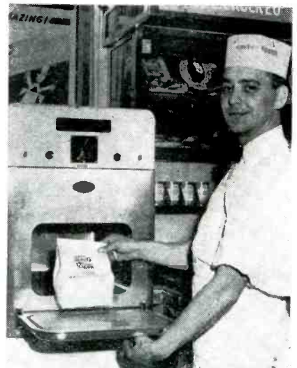
For take-out service, raw hamburgers are first wrapped in paper, placed in the bag, and then cooked by the Radarange
