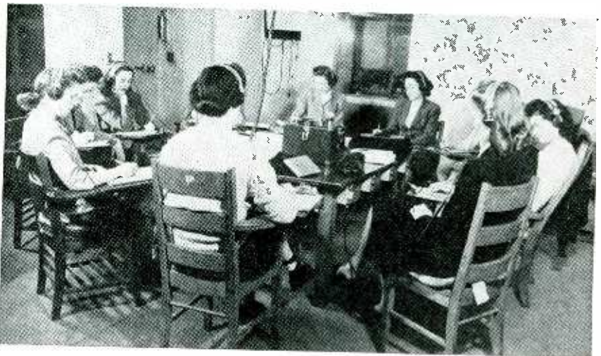
Listeners, developing data during articulation tests in which atmospheric static, such as that from lightning discharges, is artificially simulated under controlled laboratory conditions
