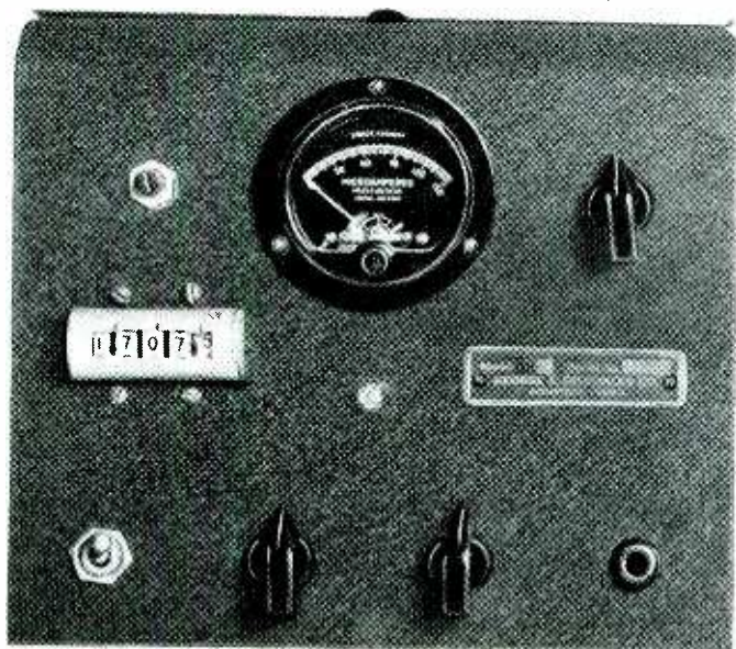
FIG. 3—Complete vacuum-tube integrator. Maximum and minimum limit controls are on the front panel
