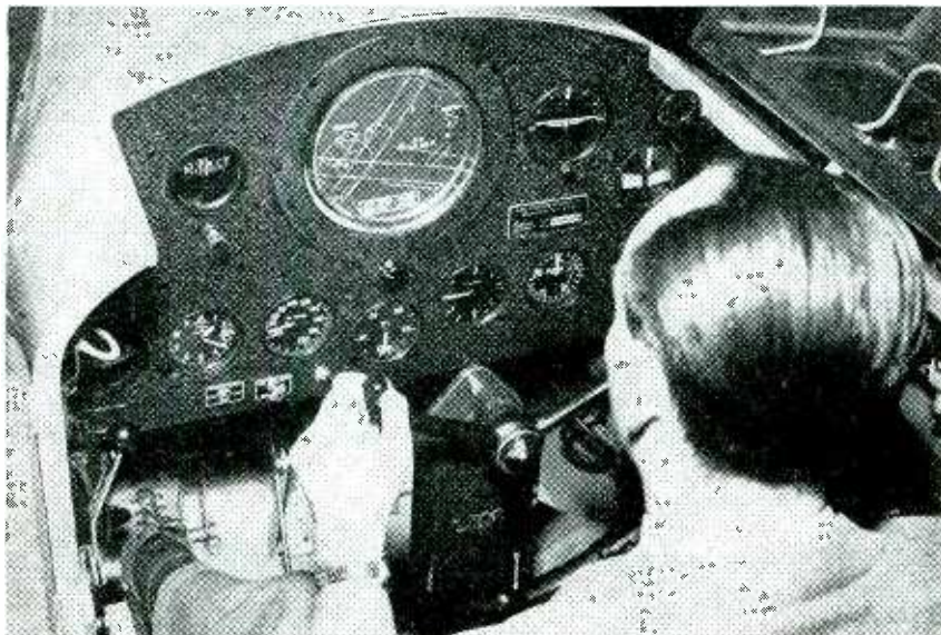
Special installation of Teleran receiver in cockpit of flight simulator brings this air navigation aid to the second of three major steps in its development program by RCA. Final step is actual flight test, scheduled to start in Washington, D. C. in the fall. The system utilizes television and radar to provide the pilot with an aerial roadmap combining traffic, route, weather, and other vital information
