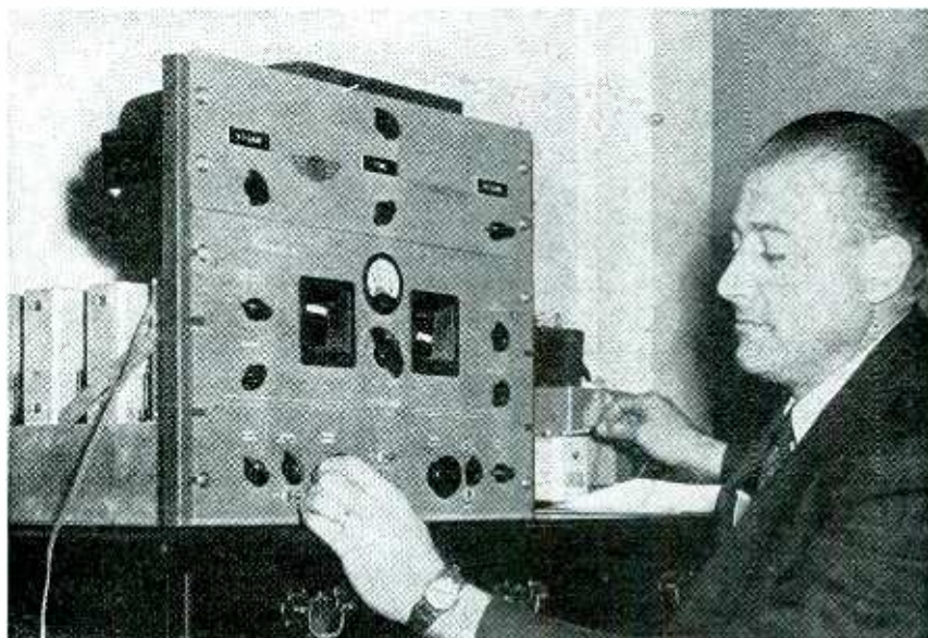
The noise-discriminating system developed by the author is used in conjunction with a conventional communications receiver
