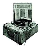
K8 Recorder (12") is complete with amplifer and speaker, operates at both 78 and 33½ rpm, outside-in and inside-out. It is equiped with a high frequency equalizer. Fifteen minutes of voice quality may be recorded on a single side of a 13½ disc. This unit is used by many schools, co-leges, broadcast stations and recording studios.
