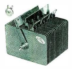
Large Stack) Selenium Rectifier. Three phase bridge, fan cooled. Output rating 100 amperes, 14 volts DC. Size over all 73/4" x 51/2" x 6". (Small Stack) Selenium Rectifier. Single phase DC valve. Blocks 30 volts, passes 0.15 amperes DC. Size over all 1" x 1½" x 3%".
