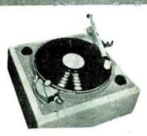
62A Transcription Turntable has been widely used by broadcast stations and recording studios during the part five years. It is rim driven through a machined rubber tire at the outer diameter of the turntable, providing a very simple and quiet drive.
