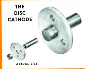
THE DISC CATHODE, another outstanding Superior development, consists of a nickel tubular shank, a ceramic insulator, and an emitting cap welded to the shank. Through the use of integral beads (embosses) on the tubing, the insulator is firmly held, yet with much less heat loss than with other designs.
