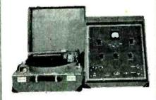
The Y Recorder (16") is the lightest portable recorder having all the features necessary for high quality recordings. The turntable is driven by a synchronous motor through a machined rubber tire on the outer diameter of the turntable. The 10 watt amplifier is equipped with two microphone inputs, connections for double turntables, high and low frequency equalizers and 10" speaker.
