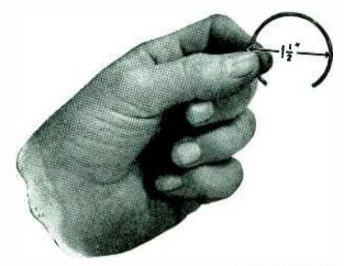
CONVENTIONAL POTENTIOMETERS have a coil diameter of approximately 1½" and provide only 4" (about 300°) of potentiometer slide wire control.
