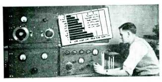
Power Factor Test on Standard Dilecto Grades—The standard test method is called the Resonant Circuit Resistance Variation Method. Measurements are at 10° cycles per second. Equipment for this test consists of a stable high frequency generator, a vacuum tube voltmeter, decade resistors, and a Standard Precision Type Variable Air Condenser.
