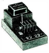
B.L "RECTOPAC". Copper Sulphide Rectifier assembly. Output rating 10 amperes, 10 volts DC. Operates from 115 volts 50-60 cycles AC. Size 71/8" x 4" x 4".
