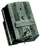
1-D Cutting Head provides stability, uniformity, and sensitivity with low distortion for recording transcriptions having specified response characteristics such as flat, NAB, etc. Response: 50-10,000 cps. Crossover at 500 cps. Response and level not offected more than  $\pm 21/2$  db between  $60^\circ$  and  $95^\circ$  Fahrenheit.
