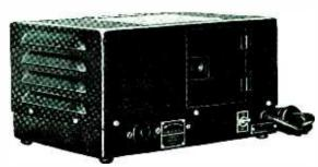
B-L SELENIUM RECTIFIER ASSEMBLY. Output rating 0.5 amperes, 115 volts DC, filtered and regulated. Operates from 115 volts, 50-60 cycles AC. Size 12" x 6" x 8".
