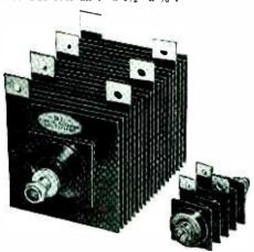
(Large Stack) Copper Sulphide. Three phase bridge, fan cooled. Output rating 100 amperes, 7½ volts DC. Size over all 8" x 4½" x 3½". (Small Stack) Copper Sulphide. Single phase bridge, convection cooled. Output rating 3.2 amperes, 5 volts DC. Size over all  $2\frac{1}{2}$ " x  $1\frac{3}{4}$ " x  $1\frac{3}{4}$ " x
