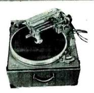
6N Recorder (16") has proven ideal for most broadcast stations and recording studios because of its high quality and relatively economical cost. It is supplied in carrying case for portable and remote assignments as well as in a cabinet. Its design is of the conventional rim driven type with overhead feed mechanism.
