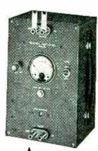
**MODEL 302 ELECTRONIC VOLTMETER.** This Sensitive Electronic Voltmeter is portable and operates from lightweight batteries contained within carrying case. Reads AC voltages from 1 millivolt to 100 volts over frequency range of 5 cycles to 150,000 cycles. Accuracy 2% at any point on scale. Can be used as highly stable amplifier. Input impedance ½ megohm. Uses standard Eveready or Burgess batteries. Battery life over 150 hours.
