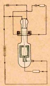
This drawing from the von Lieben German patent No. 179.807 showed an oxide coated cathode, a control element and an external relay circuit through which amplified current flowed
