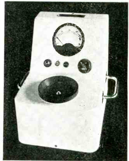
Fig. 2—Unskilled workers differ in results by less than 0.2 percent when using the moisture meter
