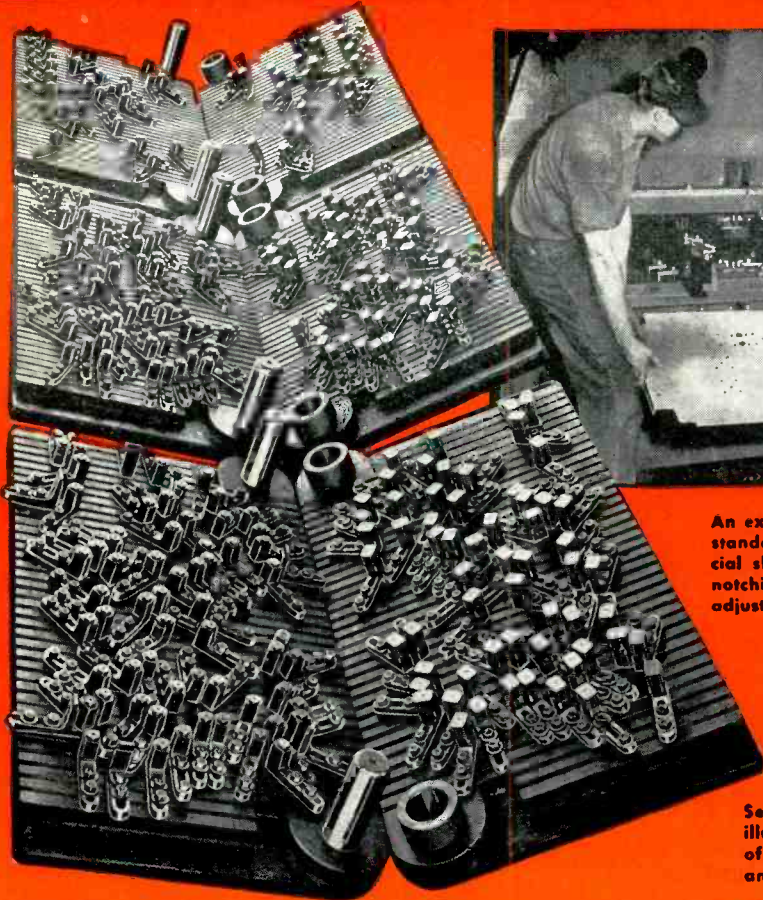
Typical 3 section set-up of Whistler multi-use punch and die units.
