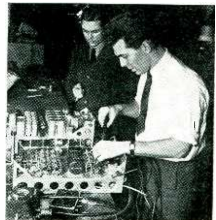
Electronic equipment for the Fairchild radio-controlled cameras for photographing atomic bomb tests on Bikini Atoll
