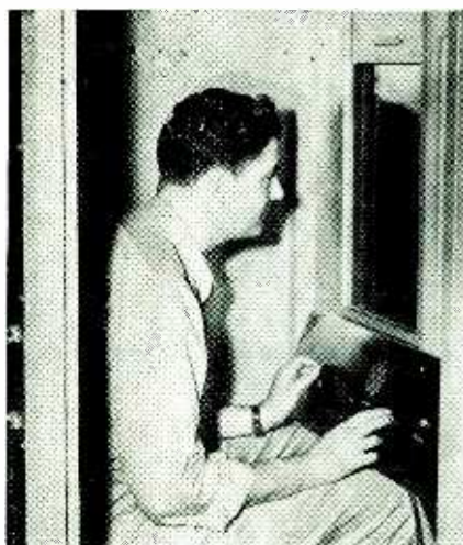
Fig. 2—Operating position of the Inspectoscope. Contents of the packages are viewed through the window above the panel
