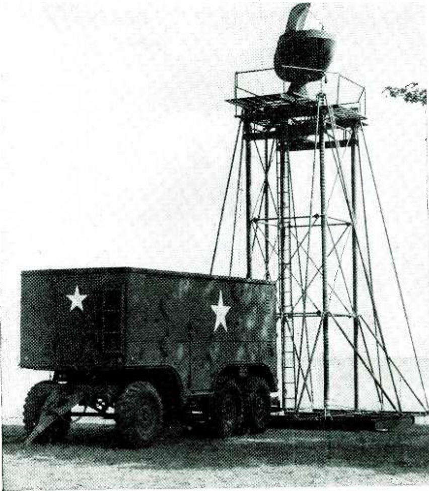
AN/MPG-1 trailer, tower and radiator. The "bath-tub" radiator is elevated within the tower to raise it to operating position
