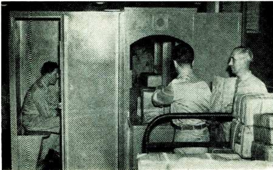
Fig. 1—Military mail clerks at the right are placing packages from soldiers abroad into the examining bay of the Inspectoscope which x-rays them for illegal objects
