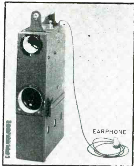
Experimental model of the sensory aid for the blind developed at the Signal Corps Engineering Laboratories
