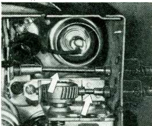
Coupling external control shafts to tuning elements—as in this radio receiver—damps noise-causing vibration, eliminates need for precise mounting and alignment of tuning elements—also gives complete freedom in their location.
