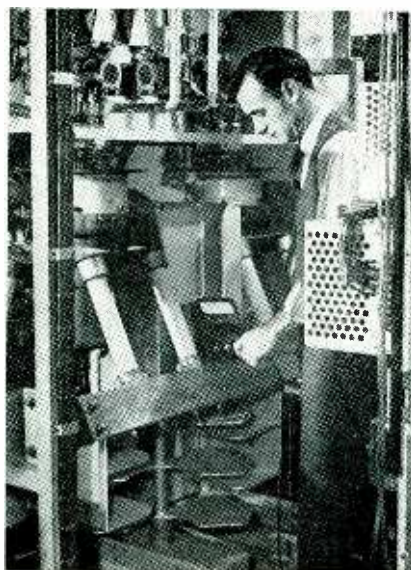
Power tubes and tuning capacitor of the 125,000-watt electronic vulcanization unit installed at the Firestone plant in Fall River, Mass.
