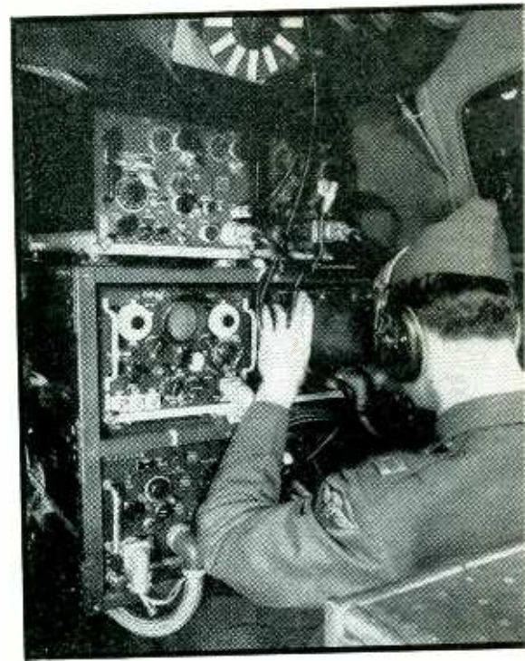
Search and jamming equipment on a Navy rcm plane: from top to bottom; antenna selector switch, APT-1 electronic jammer, panoramic adapter (to sweep receiver frequency) pulse analyzer, cathode-ray d-i indicator (in use by operator), second jamming transmitter, and search receiver (hidden by operator)
