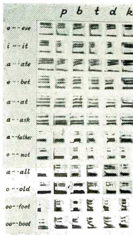
Typical speech patterns for representative syllables as they appear on the moving belt or the fluorescent screen
