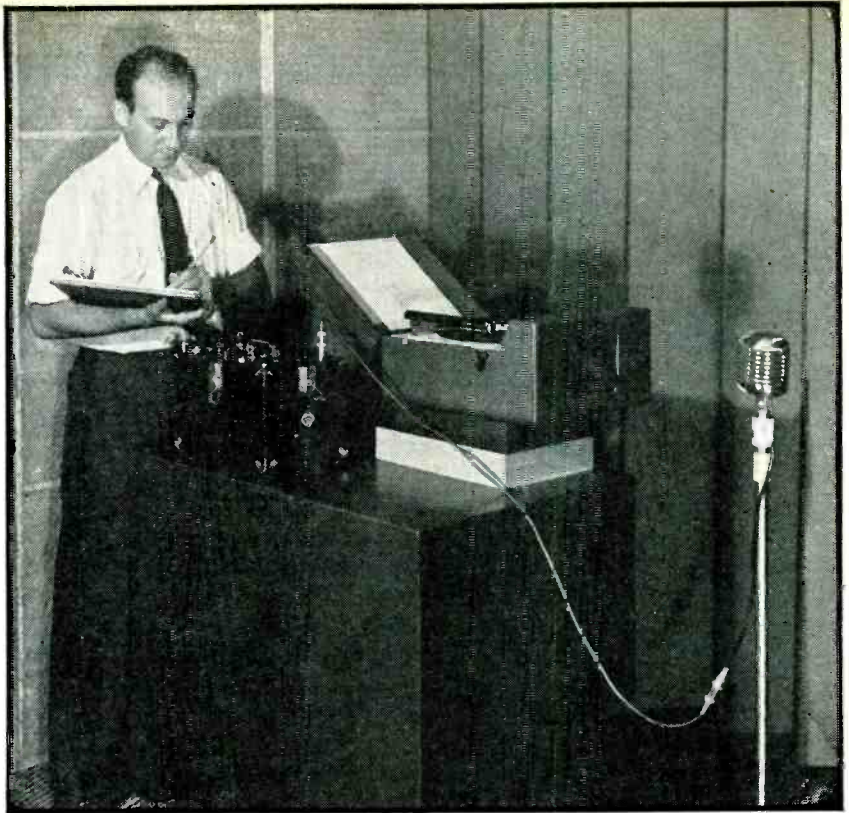
Overall frequency characteristic of a portable record player is measured by means of a calibrated microphone and sound level meter
