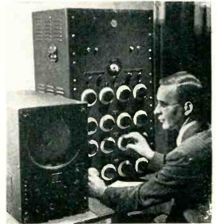
Fig. 1—An RCA technician manipulates the controls of the Antennalyzer which solves the mathematics of directional antenna-array design
