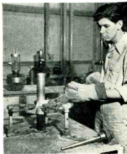
FIG. 3—Anodes for small air-cooled transmitting tubes are brazed with a smaller number of burners
