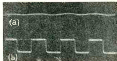
Fig. 3—Trace of input (a) and output (b) on a two-beam oscilloscope show the pulse amplification obtainable at 1000 cps. The output peak voltage is 100 volts. Exponential decay of the square waves are caused by stray reactances in the connections to the oscilloscope
