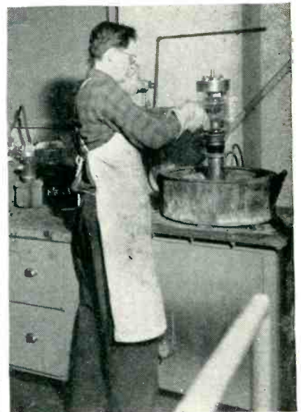
FIG. 4—Lowering the tube into the radiator assembly for soldering
