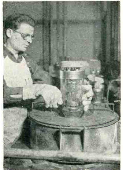
FIG. 5—A weight on top of the tube maintains constant pressure to force the anode into the radiator
