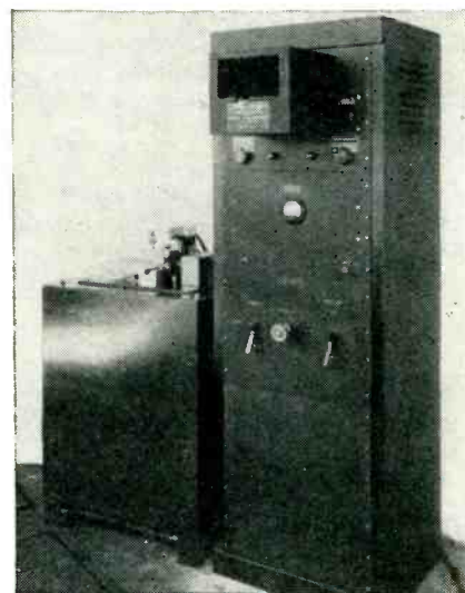
Parts to be balanced are mounted for test on the seismically suspended platform at left. The electronic equipment in the cabinet at right includes a cathode-ray tube indicator and a phototube tachometer.
