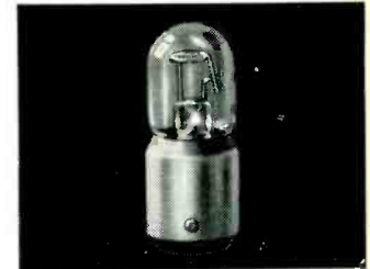
NE-17 Indicator and pilot light lamp that flashes to show condition of B-battery in portable radios. Frequency of flashes decreases as battery runs down.
