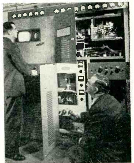
R. D. Kell and T. L. Gottier made adjustments on an experimental 300-mc transmitter for television developed at the RCA Laboratories
