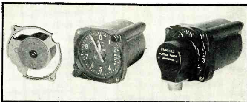
Left to right: Pickup unit that attaches to face of instrument on plane; altimeter on plane, with small permanent magnet attached to its pointer; altimeter with pickup
