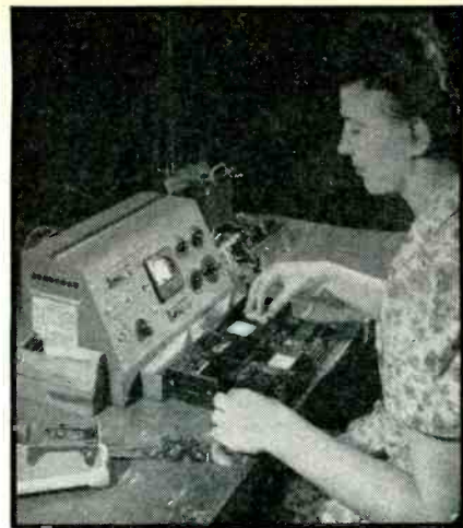
Layout for assembling silvered mica capacitors with looped-in foil, with provisions for checking capacitance continuously during assembly
