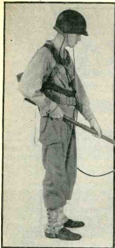
Detector set in operation. Operator is using headphones, as required in locations where ambient noise level is high or silence requirements prohibit use of the loudspeaker-type resonator
