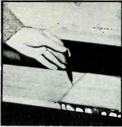
FIG. 12 (above)—Scarf joint in \bar{a} \frac{3}{4} x 6-in. board made by the method illustrated in Fig. 11
