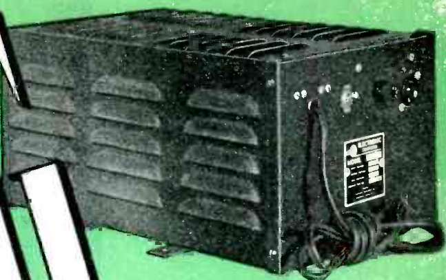
This E-L Power Supply (Model S-1374) is a high-powered unit, putting out 750 volt-amperes. Input voltage is 115 volts DC, and output voltage is 115 volts, 60 cycles AC. Efficiency is 70%. It weighs 50 pounds.
