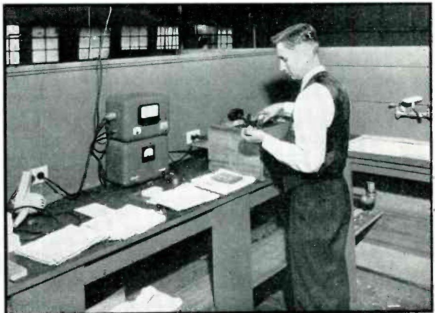
FIG. 6—Mass etching of crystals, latest innovation in the chemical method of finishing. Harmless fluorides less difficult to handle than hydrofluoric acid have recently been developed for such work
