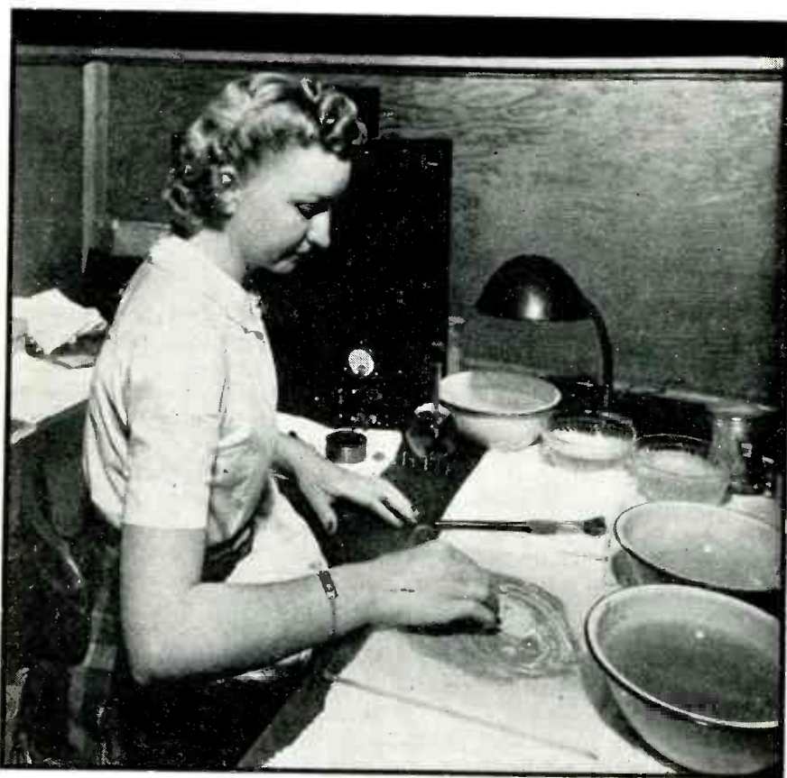
FIG. 1—Individual finishing position and operator. Test gear may be seen in the background, with a heavy, circular metal block and light copper plate constituting electrodes projecting from it for rapid and convenient frequency and activity checks. The girl is lapping a crystal on a flat glass plate smeared with abrasive
