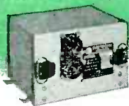
Here is a low-powered E-L Power Supply (Model S-1361). Its output power is 10 watts. Input voltage is 24 volts DC, and output voltage is 350 volts DC at 25 ma. It weighs only 5 pounds.
