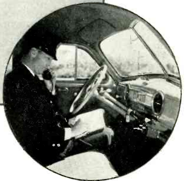
BELOW: Control panel for mobile radiotelephone set is mounted at base of dashboard in squad cars
