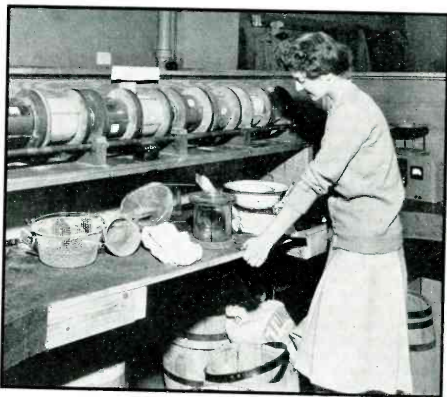
FIG. 4—Finishing crystals by "tumbling." They are placed in glass jars, along with abrasives, and the jars are rotated by means of a motor
