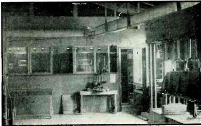
FIG. 5—Radio-frequency equipment installed at Tolerton Lumber Company, Alliance, Ohio, for making laminated spars. The r-f generator is located in the room in the background. Transmission lines consisting of sheet-metal outer conductors and copper tubing inner conductors can be seen running around the top of the room to the edge-gluing press just barely visible at the left and the big flat-gluing press at right
