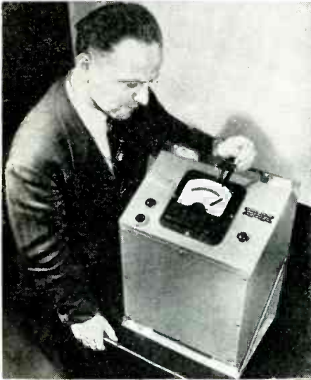
H. P. Kuehni, of G-E general engineering laboratory, points to the safety limit marking on the dial of the crane stability gage he developed
