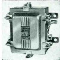
corners are gas welded inside and out. The unit is closed by a simple eyebolt and wing nut arrangement of clamping design which protects the rubber gasket from excessive pressure caused by forcing the wing nuts too tight. Federal Electric Products Co., 50 Paris St., Newark, N. J.
