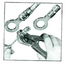
since the terminal barrel is symmetrically located with respect to the plane of the tongue, eliminating the necessity of distinguishing between and stacking two different terminals. These new terminals (for wire sizes 22 to 10) are pure copper and hot electrotinned for maximum corrosion resis-tance. The terminals are crimped on the wire with hand, foot or power tools.
