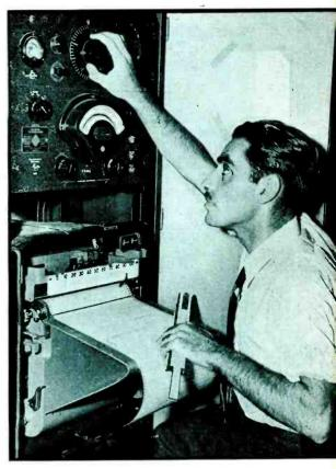
Equipment for receiving and recording the signals from Diamond-Hinman radiosonde. At top is a super-regenerative receiver; below it an electronic audio frequency meter and at the bottom a recorder which makes a record of the frequency meter readings
