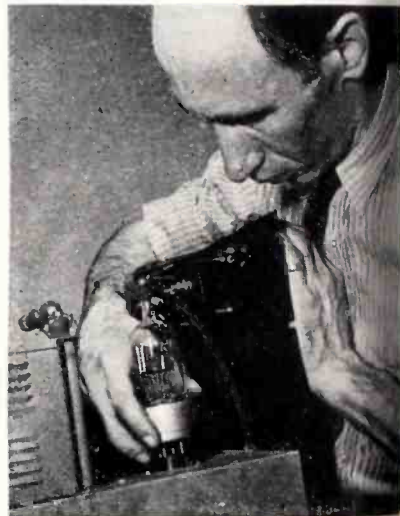
Fig. 2—The heart of the system, a special half-wave rectifier tube with gas intake and exhaust ports
