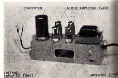
Fig. 3—Photograph of the electronic portion of the equipment
