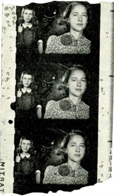
A sample of the Electroplane camera's work at full f/3:2 aperture. The girl walking in the foreground is four feet away, her companion moving in the middle-distance eight and the rear wall 25 feet away
