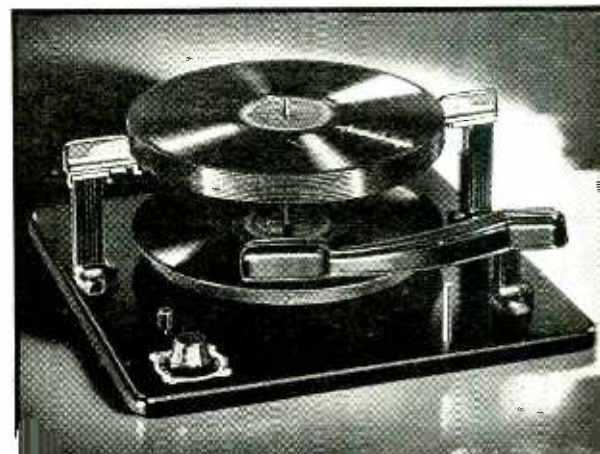
In the Farnsworth changer the bottom is pushed back and forth until it rests on a pair of hooks which are removed simultaneously
