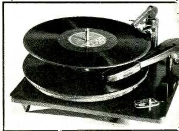
The bottom record is pushed off the two supporting areas by an arm in the separator post in this changer by General Instrument
