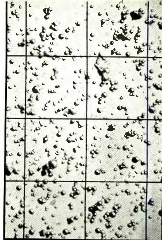
Photomicrographs of two typical types of carbonyl iron
