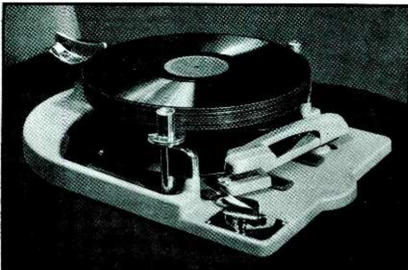
The RCA two-side playing automatic record changer uses a dual pickup, one unit for the top of the record and the other for the bottom. A small-diameter turntable permits the playing of the bottom side
