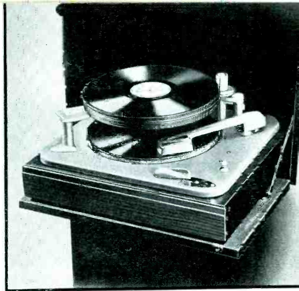
The record stack in the RCA changer is supported at one edge by the separator post and at the other by a stationary support
