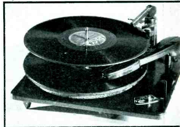
The bottom record is pushed off the two supporting areas by an arm in the separator post in this changer by General Instrument
