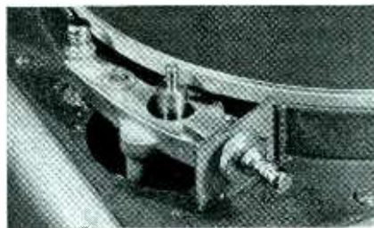
• Simple, foolproof Presto drive system—steel motor pulley drives against rubber tire on turntable rim, only 2 moving parts.
