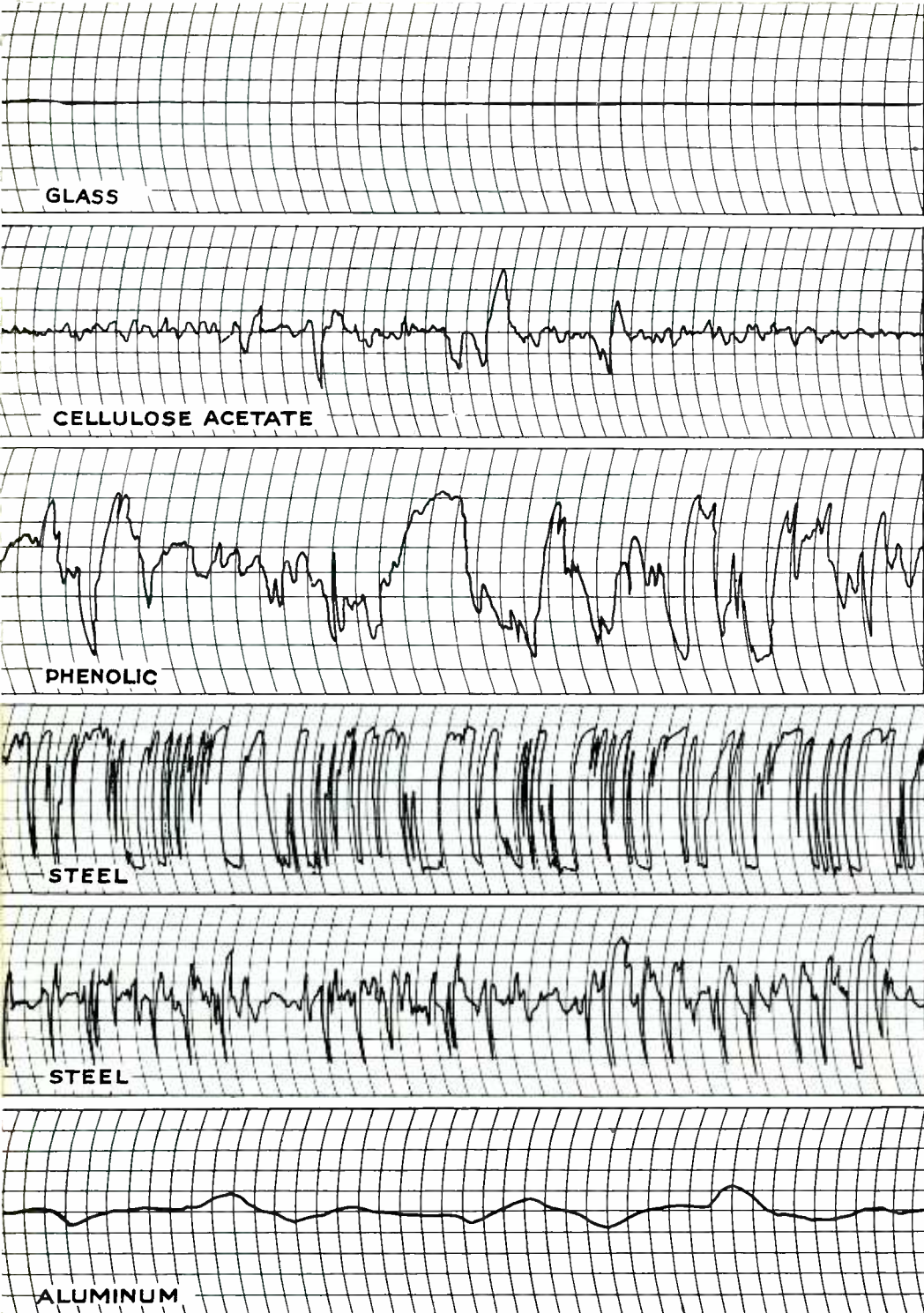
Fig. 1—Surface characteristics of several possible base materials for recording discs. Each vertical division indicates a departure from absolute smoothness of five millionths of an inch. The horizontal distance is eighty times greater than the actual distance traversed
