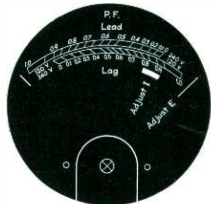
Fig. 10—Meter scale for power factor meter with lagging and leading factors for 150 and 250 volt circuits
