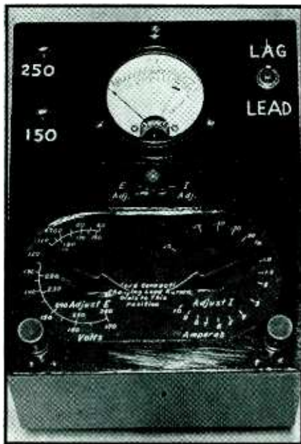
Photograph of the power factor meter which reads leading or lagging power factor directly on 150 or 250 volt circuits
