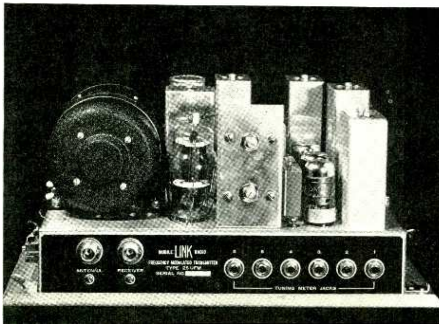
Fig. 6—Front view of the mobile transmitter with cover removed. Note the coaxial jacks at the left for the antenna and connecting cable to the receiver
