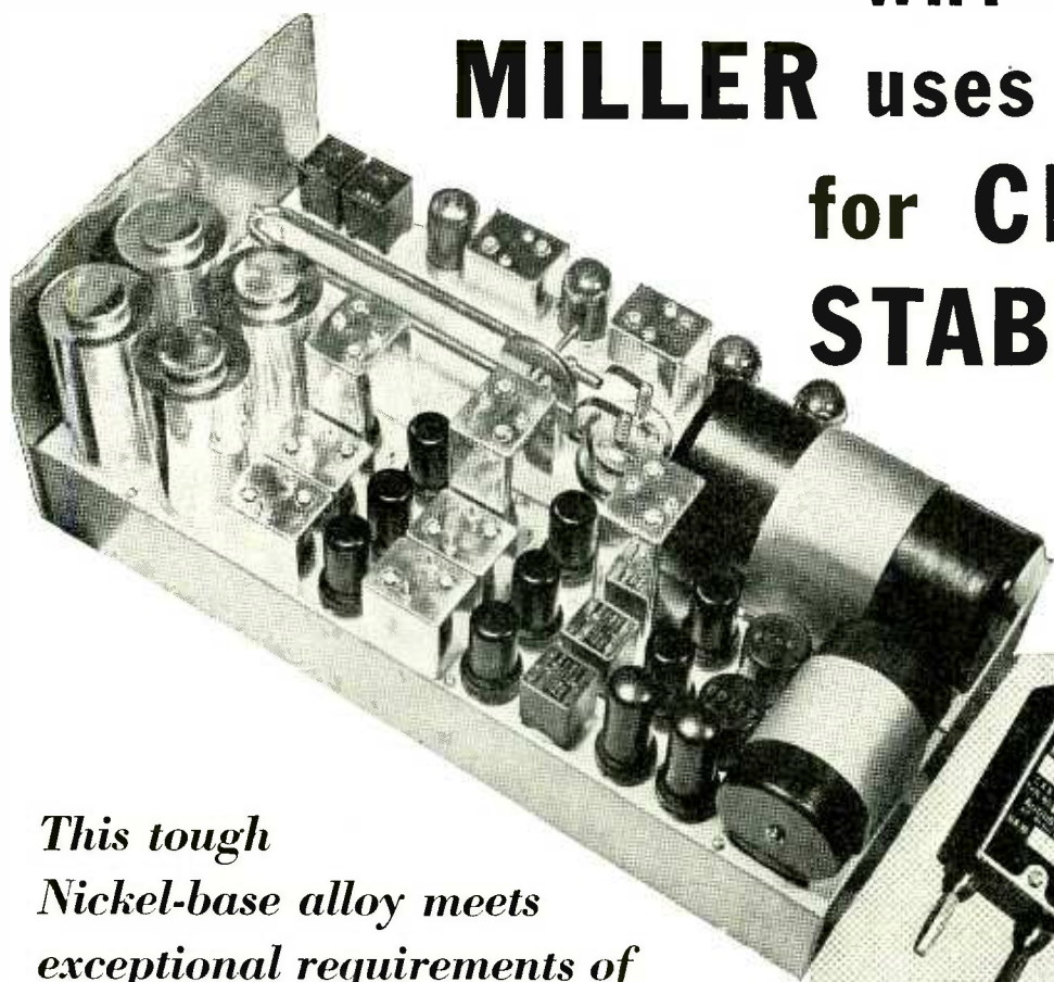
(Below) Monel plates, springs and screws as used in crystal stabilizers made by August E. Miller Co., 1922 Bergenwood Rd., North Bergen, N. J. At left is shown transmitter with stabilizers inserted on chassis.
