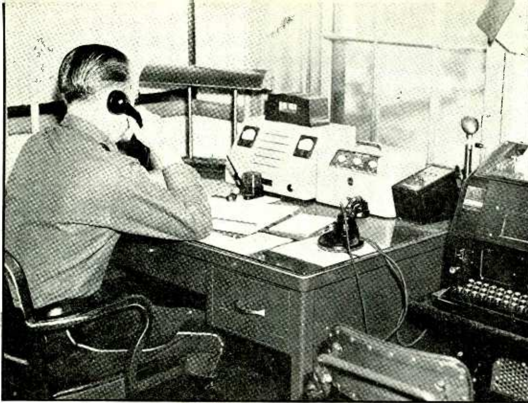
Fig. 10—The control unit at headquarters. The transmitter is put in operation when the operator pushes a button on the handset. Transmission occurs on 39,500 kc, reception on 39,180 kc
