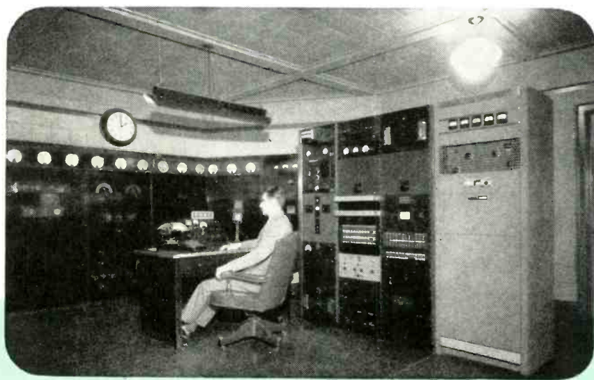
Chief Engineer C. B. Persons at the controls of WEBC and W9XYH. At the extreme right is the 250-watt General Electric FM transmitter.
