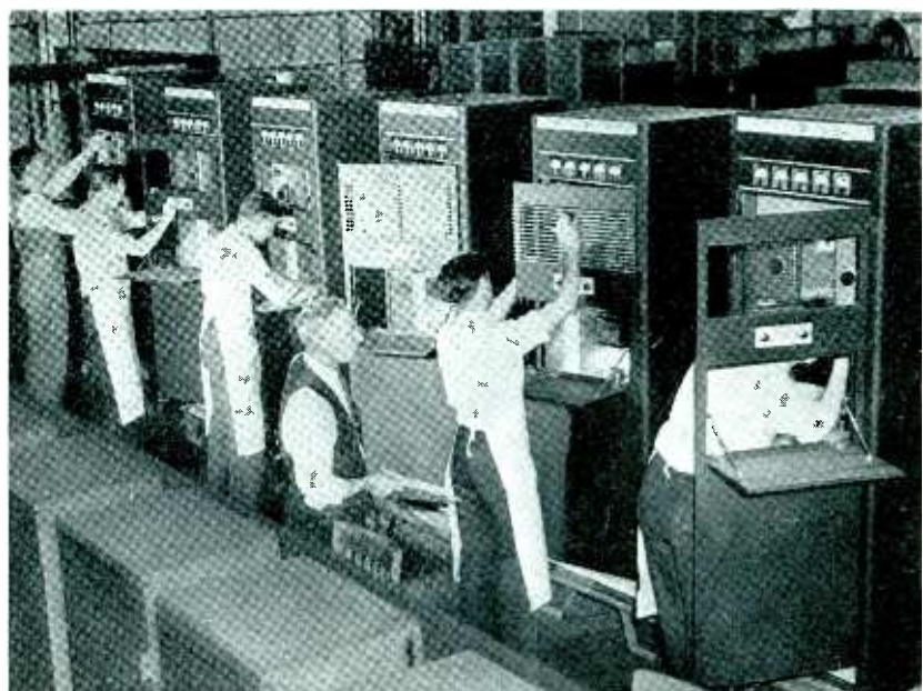
A lineup of 1-kw f-m transmitters in various stages of completion in the G.E. Radio Dept., Schenectady
