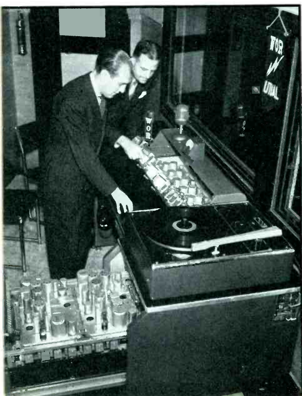
Alfred Wallenstein and J. R. Poppele, Chief Engineer, examine the innards of the new console installed in WOR's Studio One especially for f-m broadcasting
