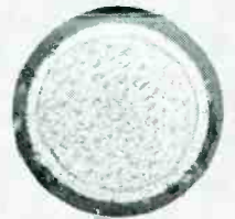
Photomicrograph of cross-section of Westinghouse thoriated-tungsten filament wire, showing properly controlled depth of tungsten-carbide layer for good strength, emission and life.
