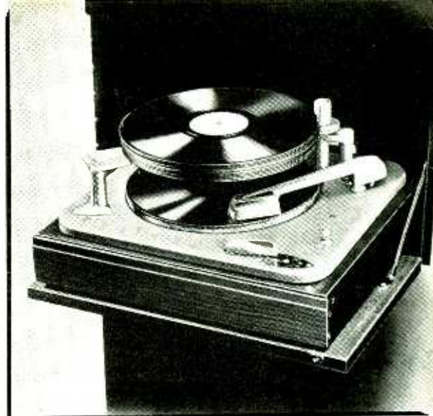
The record stack in the RCA changer is supported at one edge by the separator post and at the other by a stationary support
