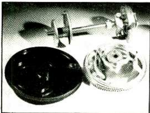
(Above) Typical cams used in automatic record changers. The main cam is the heart of the changer mechanism in that it controls all of the operations after it is started
