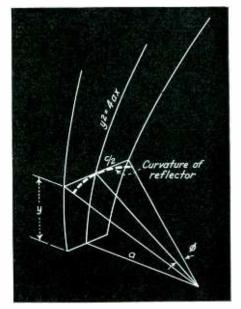
Fig. 6—Mathematical construction diagram of the parabolic reflector and collector
