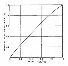
Fig. 6—Curve showing that the relation between power rectification efficiency and the ratio of d-c voltage to a-c voltage is nearly linear
