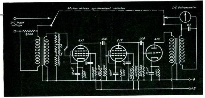
Circuit diagram of amplifier and switches. The combination of the switches and the circuit rectifies a series of half wave impulses to deflect the meter
