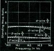
Fig. 4—The standing wave ratio is quite constant over the operating range from 14.0 to 14.4 Mc. Å 570 ohm line was used
