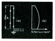
Fig. 5—A three-eights wave vertical antenna working against ground and its total current distribution curve
