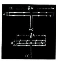
Fig. 2—Two wire, three-quarter wave antenna (terminal resistance 450 ohms) and four-wire, threeeighths wave antenna (terminal resistance 230 ohms)
