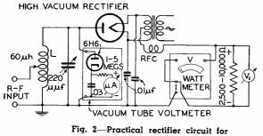
rig. 2—Practical rectifier circuit for r-f power measurement
