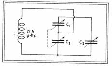
Fig. 2—Series-parallel method of tuning to insure constant bandspread
