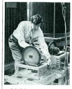
G. D. McCann sets into trial operation one of the fifty fulchronograph surge recorders which have been installed to study lightning. The fulchronograph makes a record of current in a natural lightning stroke throughout its entire duration
