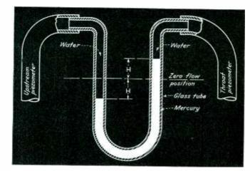
Fig. 2—Mercury-filled U-tube, connected to the throat an upstream point on the Venturi tube
