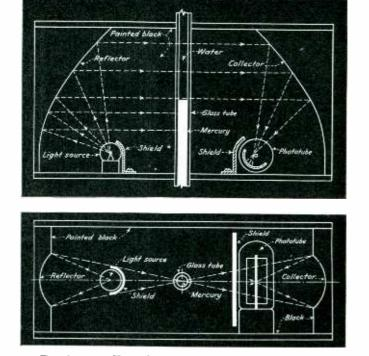
Figs. 3 and 4—Vertical and horizontal sections of the measuring unit. The height of the mercury column determines the amount of light reaching the phototube
