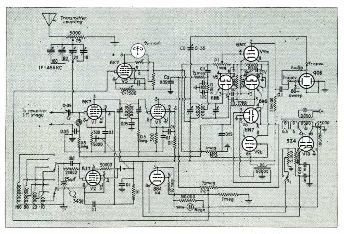
Fig. 6—Circuit diagram of the complete modulation monitor. It is connected to the final i-f stage of a receiver. For measuring a transmitted signal, the 5000-ohm portion of the  $V_1$  cathode resistor is cut in and the plate and screen circuits of  $V_2$  are closed
