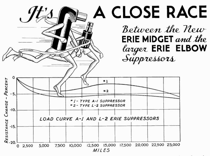
Racing along together in our laboratory for an equivalent of 25,000 miles at 50 miles per hour, the recently developed Erie Midget Suppressor proved itself equal in efficiency with the larger Erie Elbow Suppressor. Run under a primary voltage of 9 volts with a 1/4" spark gap . . . conditions more exacting than encountered in actual installations . . . the type A-1 Midget finished with a drop of 6.25% and the type L-2 Elbow with 6.67%.
