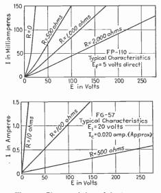
Fig. 2-Characteristics of both vacuum and gas triodes used as rectifiers.
