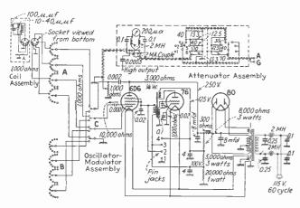
Fig. 1—Circuit diagram of the signal generator which provides a frequency range from 115 to 16,000 kc.
