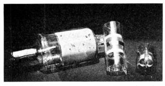
Several types of multiplier tube. The large tube with pure uncoated nickel cathodes produced one-half microampere per lumen sensitivity acting as a photoelectric device.
