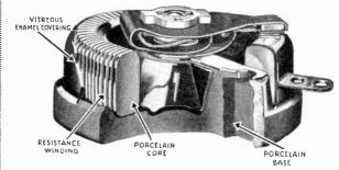
The cross-section picture shows several of the exclusive features of Ohmite all procelain rheostats—solid porcelain core—vitreous enamel bond between winding, core, and base—no organic material to smoke or char—flat contact surface—large number of contact steps—shafts insulated against high voltage.
