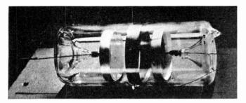
Plate-like cold cathodes with anode ring between. A tube five inches long with cathodes approximately 2 inches in diameter will produce 10 watts or more of high frequency power.
