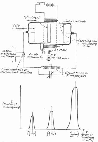
The double-cathode electron multiplier and associated apparatus. Connected as shown the tube acts as a highly efficient r.f. current amplifier. The volt ampere characteristics are shown below. The several peaks are produced by anode voltages bearing a definite relation to the transit time of the electron.
