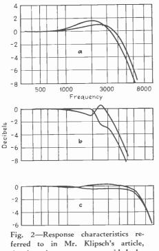
ferred to in Mr. Klipsch's article, showing improvement provided by neutralization.
