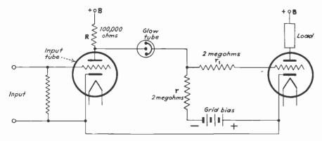
D.C. amplifier which uses a glow discharge lamp as the interstage coupling.
