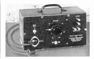
A new simplified sweep circuit for cathode-ray oscillographs.
