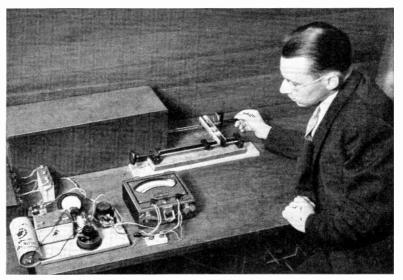
Set-up used in the Bell Laboratories for measuring the "Q" (ratio of inductive reactance to resistance) of circuits tuned to wavelengths in the neighborhood of 60 centimeters.
