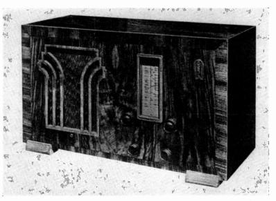
The waveband in use in this English superheterodyne is shown by colored lights behind the tuning indicator.
