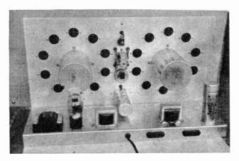
Fig. 2—The oscillator assembly showing socket for the coils for each frequency.
