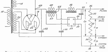
Power supply ripple neutralized by a "self-bucking" system. U. S. Patent No. 1,965,661.
