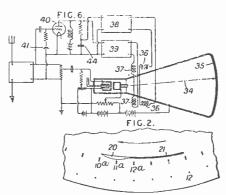
chronizing impulses are transmitted with the picture signals in the same channel, the synchronizing impulses are separated from the picture signals by amplitude selection and the synchronizing impulses of one set are developed with a steepness of wave front substantially different from that of the other set. R. D. Kell, Marconi Co. No. 407,409.
