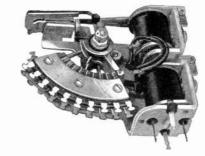
The Autelco Minor Switch can be used to select any desired contact of a group of ten, control being accomplished by push button, telephone dial, etc. Switch is operated and restored by electromagnets. One, two or three levels can be furnished, ten contacts per level, with one, two or three non-bridging double-spring wipers. Arrangements can be made for operation on from 6 volts up to 110 volts, D.C. Current-carrying capacity per wiper, at rest—3 amperes, D.C. or A.C.
