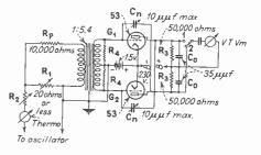
Fig. 1-Circuit diagram of neutralized push-pull audio amplifier.
