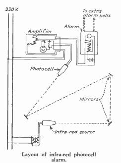
be increased to meet the particular requirements of the installation. The use of the multiple light path has the same advantage as the use of a series circuit in electric alarm practice, that is, interference with the light at any one or more points of the beam will actuate the alarm. A neatly mounted amplifier and alarm unit are connected to the photocell output. The power supply for the entire system is obtained from regular 110 or 220 volt lines.
