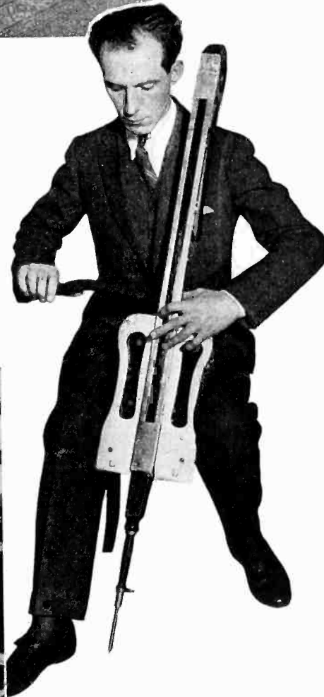
Professor Leon Theremin and his fingerboard cello instrument. With the left hand, the player fingers a contact strip, much as he would the strings of a viol, and with the right hand he works the volume lever.
