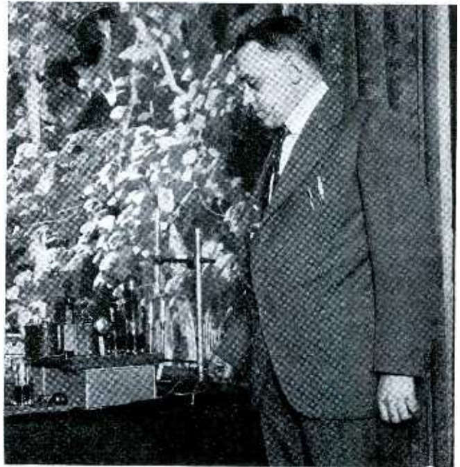
Dr. H. C. Rentschler and his ultra-violet dosage meter. A condenser is permitted to charge by the photo-electric cell so long as radiation falls upon the latter. The condenser discharges at regular intervals and registers the amount of ultra-violet that has fallen on the cell—and on the patient.
