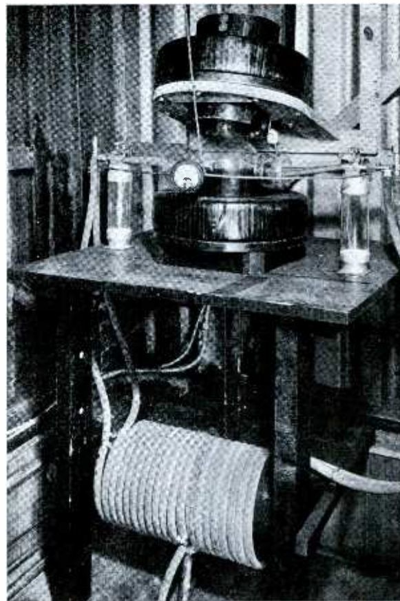
Fig. 4—Water-cooled split-anode magnetron and associated apparatus for production of high-power high-frequency oscillations
