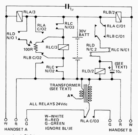
are replaced, RLC is shorted through the 100 Ohm resistor and turns off, resetting the bellringing circuit. The
