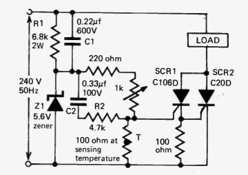
of line voltage appearing at the anodes of both SCRs.
