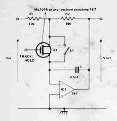
When the switch is closed (or the FET conducting), circuit is behaving
