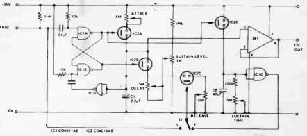
while IC1(d)'s output will go high again. When S1 is in position '2' the sustain is controlled by the monostable thus formed. It is retriggable so that should a second trigger arrive before the cycle has completed the cycle will restart. The 741 buffers the output.
