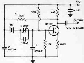
Fig.6. Parallel mode LF oscillator.
