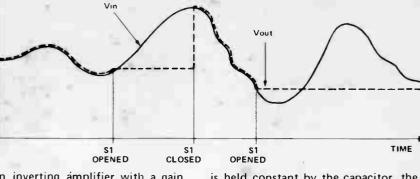
as an inverting amplifier with a gain of  $\frac{R2}{R1}$ . As the inverting terminal of of the op amp is a virtual earth, the capacitor is kept charged to the output voltage by the op amp. When the switch is opened (and the FET nonconducting) the voltage at the output
