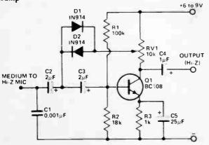
Maintaining high average а modulation level for mobile transmitters communications considerably improves the of transmitter, effectiveness а especially under difficult conditions. This circuit provides a small amount of preamplification as well as variable clipping level (preset).
