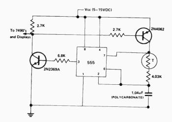
9.06:1 over the temperature range OOC to 50°C. The capacitors need to be temperature stable and may need to be hand selected and added to give the
