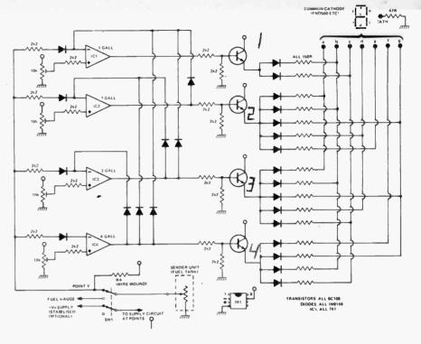
In the case of IC4 (representing 4 gallons), the voltage at point Y may be of a level to give IC4 a + output, but also be lower at pin 3 on ICs 3, 2 and 1. This would mean that the non-inverting inputs would, in each case, also be positively biased, giving a positive output from each IC. To overcome this positive feedback from pin 6, of any IC which has a positive output, is fed to inverting inputs to preceding ICs causing those particular ICs to 'turn off'.
