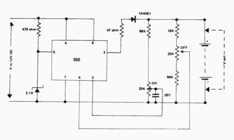
The circuit is calibrated by substituting a variable voltage supply for the NiCd batteries. The HIGH adjustment is set first so that the output switches off at the maximum battery voltage and then the LOW is set for minimum battery voltage. It is simplest to leave the output disconnected from the resistor until after the setting up procedure.
