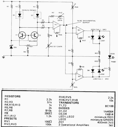
Apply probe D1 to a liquid at a temperature 10°C different from above, then adjust gain control RV2 until there is 10V at the diff. amplifier output. The CMRR
