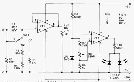
For example, with SW1 in position 2, and with a reading of 2 on RV1, the input voltage will be 2V. With a little practice, the voltage can be read to  $\pm 2\%$ , comparable to a moving coil instrument. The input impedance on all ranges is  $3.2M\Omega$ .
