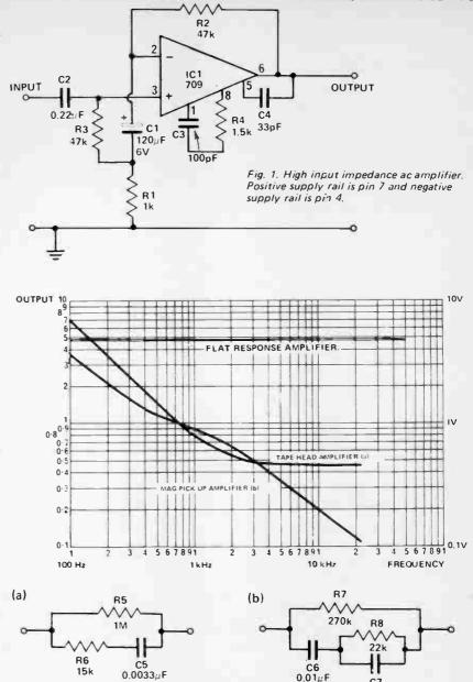
Fig. 2. Alternative feedback networks. (a) Tape head; (b) Magnetic pick-up.
