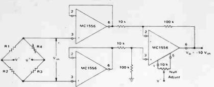
The MC1556 operational amplifier may be used as a voltage follower in a bridge amplifier application. The high
