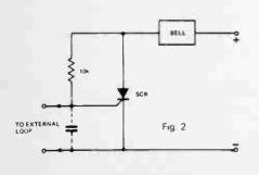
In some instances this type of false triggering can be overcome by connecting a 2uF capacitor between the SCR's gate and cathode but generally speaking it is bad practise to connect long 'aerials' directly to the gate circuit of an SCR.
