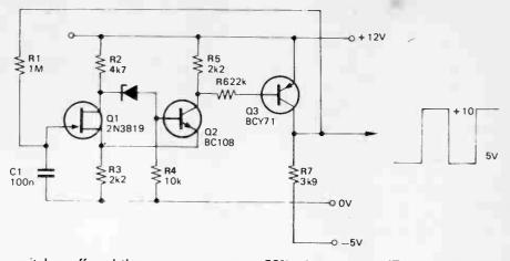
switches off and the output goes to -5V. Capacitor C1 now discharge towards -5V, but when the voltage across C1 falls by approximately 3V, Q1 ceases to conduct, turning on Q2.
