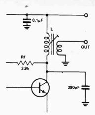
Fig.8b. Adding a coil to the circuit shown in Fig.8.
