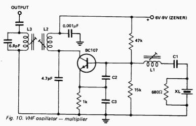
65 MHz Xtal 130 MHz OUTPUT L1 = NEOSID AZ ASSEMBLY (4mm FORMER & F29 SLUG) WOUND WITH 12 TURNS OF 4.55 mm ENAMEL WIRE, CLOSEWOUND
