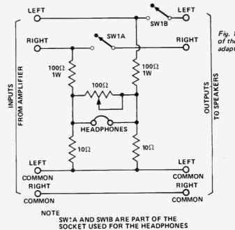
Fig. 1. Circuit diagram of the headphone adaptor. шć
