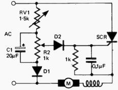
suitable for most fractional horsepower motors — for optimum results it will be necessary to adjust component values to suit the motor used.
