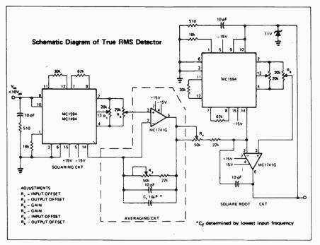
second op amp is used with a multiplier as the feedback element to produce the square root configuration. This method eliminates the
