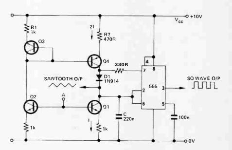
cycle recommences; the repetition frequency is determined by the magnitude of I, which is set by the voltage applied at the input point A.
