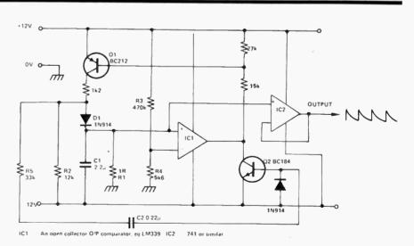
seconds by the positive feedback loop through R5, C2 and Q2, to ensure C1 charges fully. After this time C2 is also fully charged, and Q2 turns off, turn-
