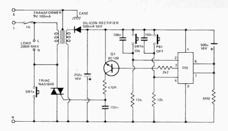
it must be rated accordingly. SW1b is used to trigger the 555 and start the timing period. Q1 will then be turned on, providing gate current to turn on the triac. When SW1 is released the supply and the load is maintained until the end of the timing period. PB1 is provided so
