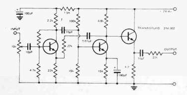
Fig. 2. Circuit details of switching mixer shown in Fig. 1. TOP: One-shot multivibrator 'm'. CENTRE: Gated mixer-amplifier 'G'. BOTTOM: Lineamplifier 'L'.
