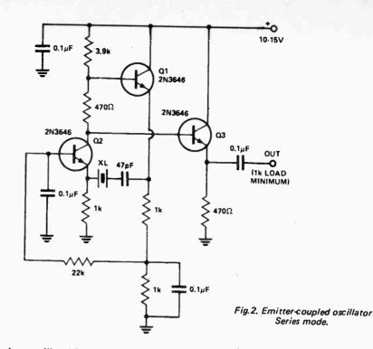
resistor will achieve this. Output then rises to about 5 V peak to peak. Power supply voltage can be reduced in this case to lower crystal dissipation.
