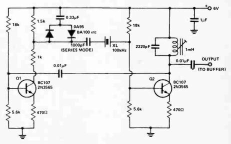
Fig.7. 100 kHz crystal oscillator (with tuned circuit).
