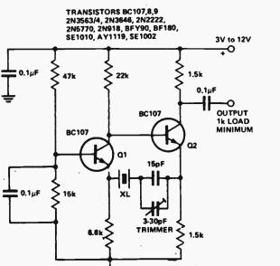
Fig. 1. Aperiodic Butler oscillator (series mode)
