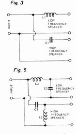
Constant k crossover networks. Fig. 2 – series type, 6dB/octave. Fig. 3 – parallel type, 6dB/octave. Fig. 4 – series type, 12dB/octave. Fig. 5 – parallel type, 12dB/ octave.
