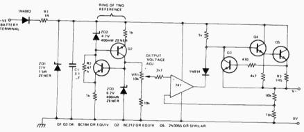
between 10 and 6 volts, so, for instance, most battery cassette equipment may be driven. Short-circuit protection is provided by Q3; when the output current exceeds 400mA
