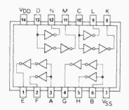
CO4042A QUAD D-TYPE LATCH (CLOCKED)
