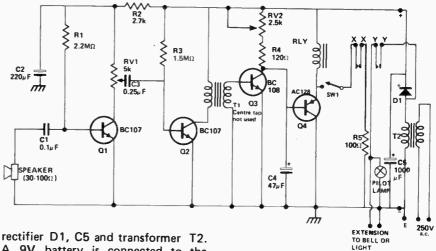
rectifier D1, C5 and transformer T2. A 9V battery is connected to the positive and negative points shown, with an on-off switch in circuit. Quiescent current is about 6mA,
