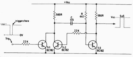
held down by the triggering waveform, so the switch-on of TR3 is not regenerative. For this reason the falling edge of the output pulse is not as fast as it might be, but is sufficient for most purposes.
