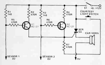
sounds the alarm. The self-latching characteristics of the SCR now make the transistor and its sensor lead inoperative and the alarm can only be stopped by switching off the concealed switch, S1.
