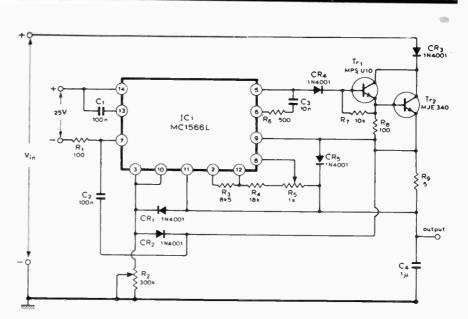
regulator receives its input from an auxiliary 25 V supply external to the chip.
