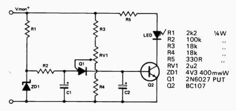
The circuit is shown in Fig. 1. The PUT (Q1) is used in a relaxation oscillator circuit. As the voltage being monitored ( $V_{mon}$ ) falls, the voltage on the gate ( $V_g$ ) falls whilst the anode voltage ( $V_a$ ) remains essentially constant. Oscillation commences when  $V_a$  falls below  $V_a$  by 0.6 volts.
