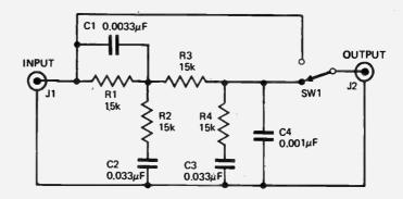
We would like to emphasize that this is a 'compromise' circuit. Ideally a loudness control must be designed specifically to suit the amplifier for which it is intended. Also the degree of loudness compensation should be related to the volume control setting.
