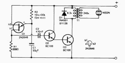
The pulses from Q1 are directed to Q2 which in turn drives Q3 into saturation.
