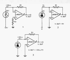
The feedback resistance, R1, is dependent on cell sensitivity and should be chosen for either maximum dynamic range or for a desired scale factor and should be chosen to minimize bias current error over the operating range.
