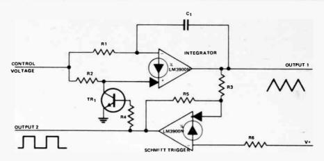
The greater the value of the control voltage, the greater the frequency of oscillation. However,
