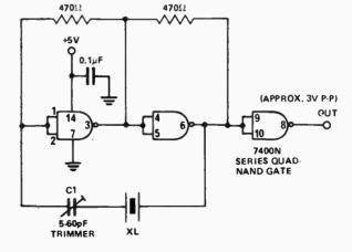
Fig.4, Reliable TTL crystal oscillator.
