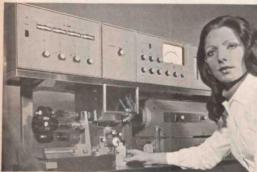
Fig. 8. An atomic-absorption flame spectrophotometer.
