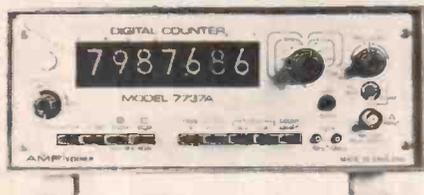
The readout is a seven-digit in-line display with automatic positioning of the decimal point, and the instrument features a switchable display-storage memory.
