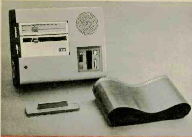
Fig. 2—IBM takes honors for elegance. Magnetic belts can be used interchangeably on other IBM Executory dictation equipment. Object in left foreground is permanent-magnet bulk-erase device.
