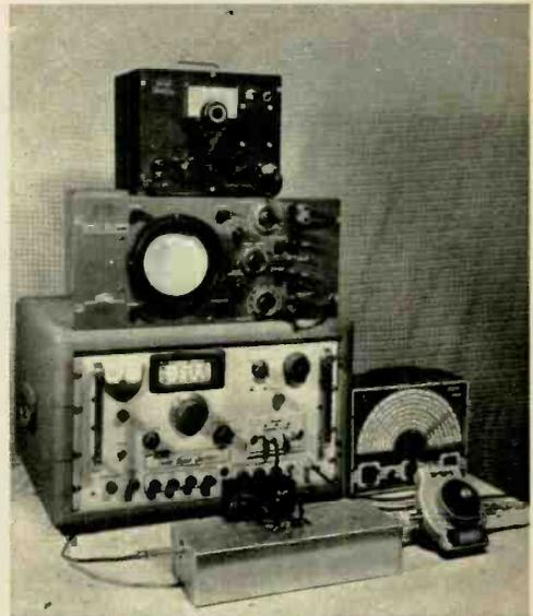
Fig. 4—Equipment used to test splitters. Below marker generator (top) is Dumont 340-R scope which sits on Jerrold 900B sweep signal generator. At right of test fixture is precision attenuator.
