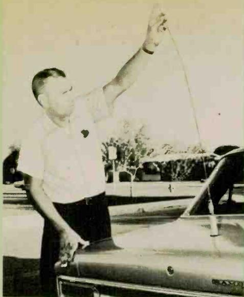
Coil-matched whips designed for  $\frac{5}{8}$ -wave mobile operation (above) are being used by increasing numbers of hams on 2 meters. The greater length gives it an advantage on both transmit and receive over standard  $\frac{1}{4}$ -wave mobile whip (right).
