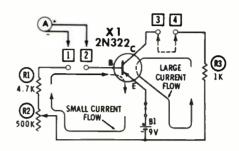
Fig. 1. Common-emitter amplifier circuit.
