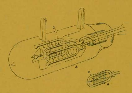
Fig. 3 A small sized Pliotron for use as an oscillation detector. G is a tungsten grid; F, a tungsten filament and A, the anode of tungsten wire. Plan of the experimental detector tube.
