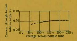
Fig. 27 Typical E-I characteristic for a barretter.
