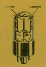
Fig. 8 Construction of a phototube.
