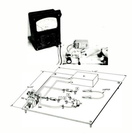
Fig. 2. Pictorial drawing of common-emitter amplifier.
