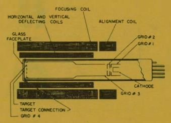
Fig. 20 Construction of a vidicon camera tube.
