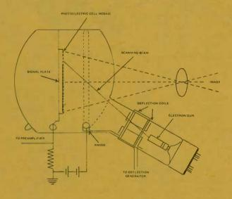
Fig. 14 Plan of an iconoscope.
