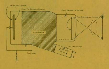
Fig. 16 Plan of the image iconoscope.
