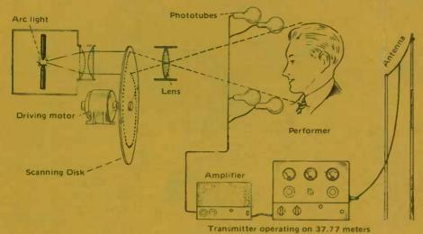
Fig. 6 Plan of a 1930 scanning-disk television transmitter.
