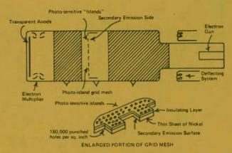
Fig. 12 Plan of the first Farnsworth image-dissector camera tube.
