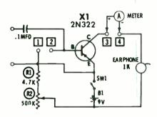
Fig. 6 - Practical AC amplifier circuit.
