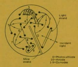
Fig. 23 Plan of a photomultiplier tube.
