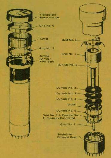
Fig. 18 Construction of an image orthicon tube.
