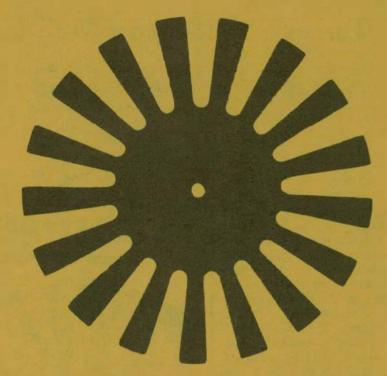
Fig. 2 — This is an actual size contact print made from a Bakelite-Celoron spiderweb coil form which was manufactured by the Nazeley Company, New York City, in the early 1920s. Use this pattern for making your own spider-web coil forms.
