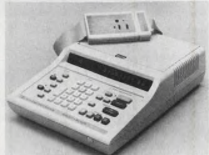
When a bus stops , the source of the failure must be found. Hooked up to the 1602A logic analyzer, this special probe from HP helps engineers visualize problems on the standard instrument interface.
