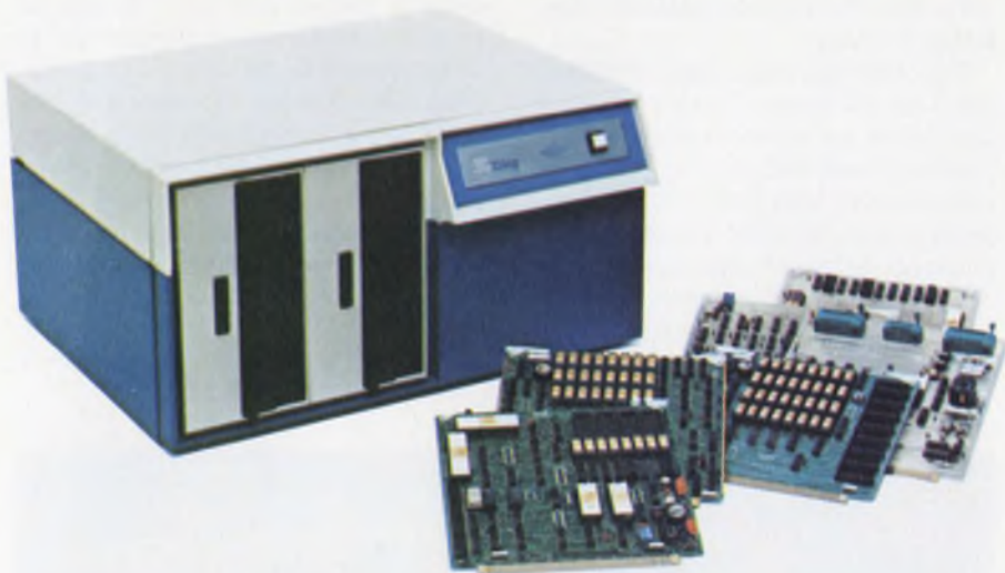
Eight-bit microcomputer systems are being refined to provide low-cost but powerful general-purpose computers. This Zilog MCZ-1 system uses high-level languages and has an operating system comparable to that of a minicomputer.
