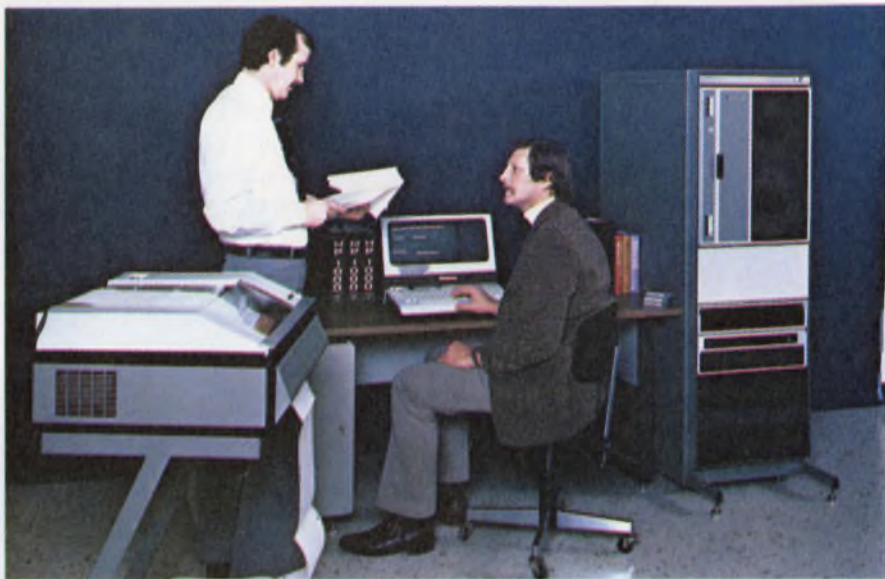
Communications features that link distributed-processing minicomputer systems and peripherals are appearing in minicomputer systems like the HP 1000, which communicates with others over modems or hard-wire links.
