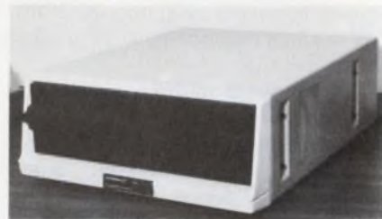
A dual floppy-disc system with on-line storage of a half-million 8-bit bytes, the Motorola EXORdisk II will be a component of M6800 systems tailored for small-business needs.
