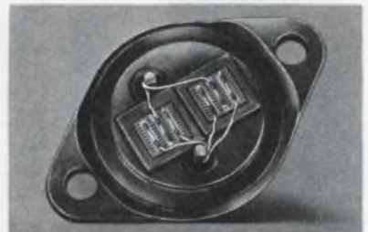
50 A Multi-epitaxial transistor
